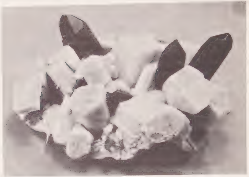
Figure 14. Smoky quartz (dark) and feldspar. Florissant, Colorado. Photograph, courtesy of Ward's Natural Science Establishment, Inc.)
