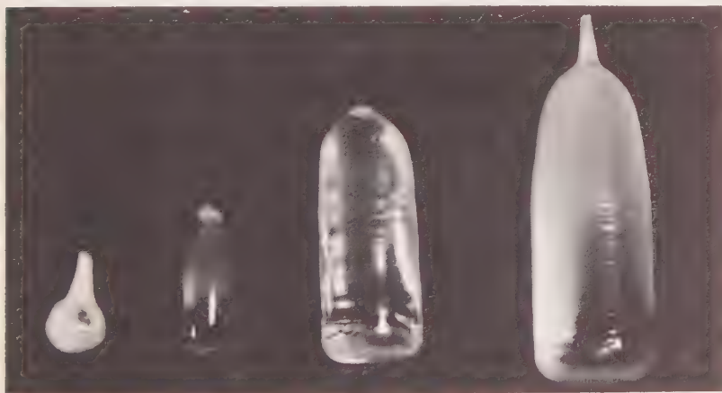
Figure 18. Synthetic sapphires and rubies before cutting. The "boule" on the extreme right is 350 carats. (Photograph courtesy of Union Carbide and Carbon Corp.)
