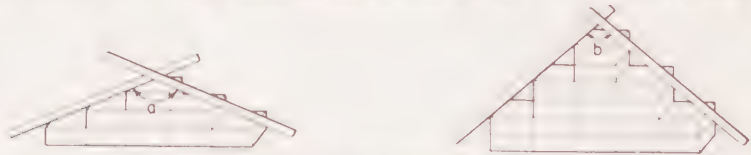
Figure 5. Stacking of identical blocks (or unit cells) showing different slopes and angles for different arrangements.
