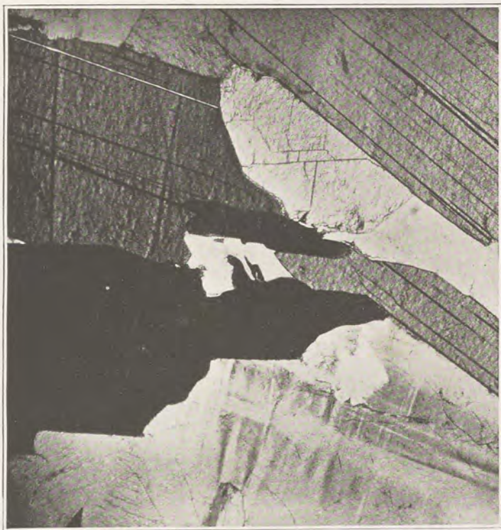
Nepheline syenite from lot 32, Con. VI, Glamorgan township, showing biotite, nepheline and microcline, with two included grains of calcite.
