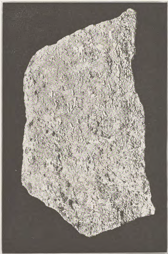
Monmouthite, lot 11, Con. VIII. Monmouth township. Nepheline (grey) with subordinate albite (white) and hastingsite (black).
