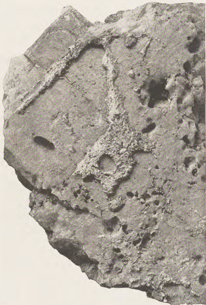
Nepheline syenite pegmatite, showing characteristic weathering, from lot 39, Con. IV, Glamorgan. Nepheline with albite (standing out on weathered surface). The cavities in the surface of the nepheline are caused by the weathering out of calcite.
