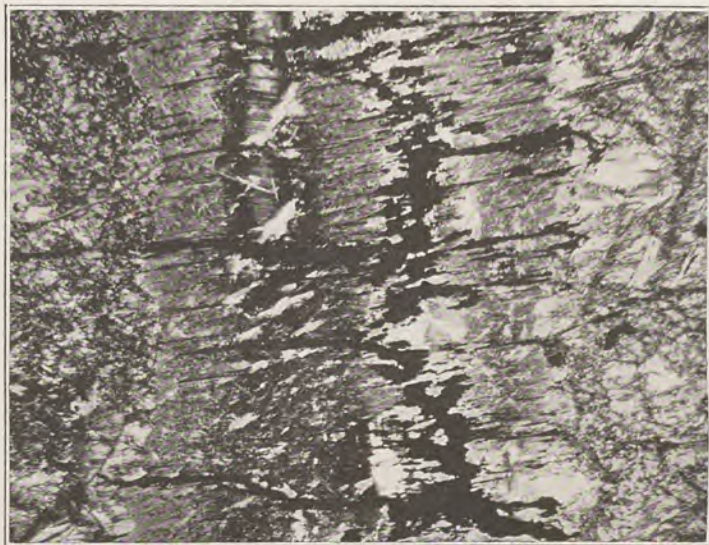
Photomicrograph of an asbestos vein, showing the irregular nature of the magnetite parting, and the contact of the vein with the serpentine wall-rock. X 14; crossed nicols.
