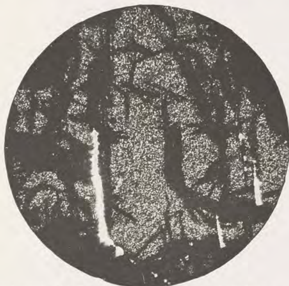
Photomicrograph of chromite ore showing intergrowth of two varieties,—black, opaque iron and chromium-rich variety, showing black; and brown, translucent, magnesian variety, showing mottled. The white streaks are glare from films of inclosed serpentine. X 55.
