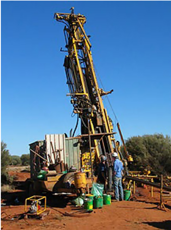
FIGURE 8.1 Heavy-duty drilling rig capable of both diamond and reverse circulation drillings. Source: Photo by S.M. Gandhi.
