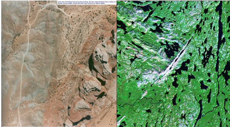
FIGURE 4.4 (Left) A fault trace near Moab, UT, USA, that would be difficult to detect on the ground is easily seen in an aerial photograph. (Right) The Ray Rock gold prospect, North West Territories, Canada. A large-scale linear feature related to an ophiolite sequence developed during Precambrian tectonism. Source: http://www.bdrgeosci.keele.ac.uk/Staff/Images/court.jpg (left) and http://www.ersi.ca/ (right).
