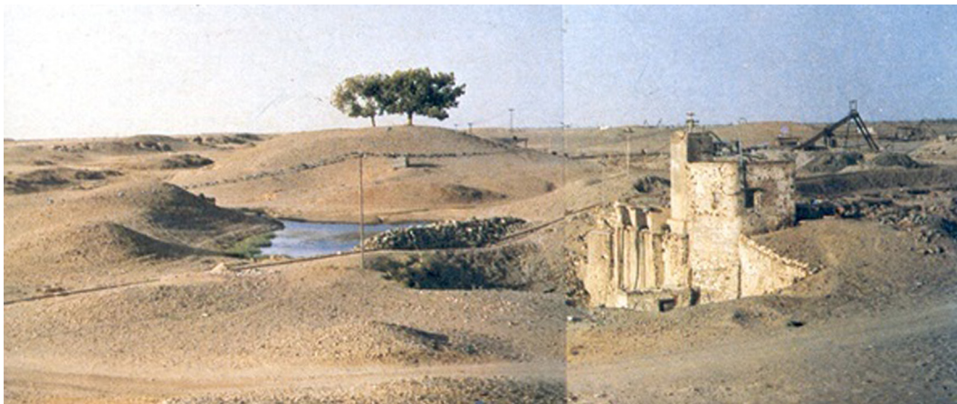
FIGURE A.7 Rampura-Agucha prospect, in March 1981. The well is in the contact of ore body and hanging wall. The head frame of exploratory incline is in the background. Source: Photo courtesy by Gandhi.
