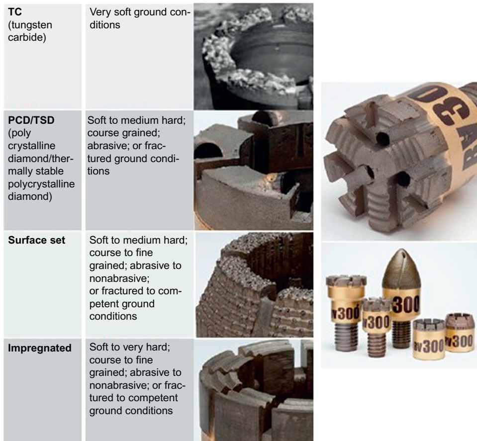
FIGURE 8.3 (Left) Types of drill bits; (right) directional and wedging bits. Source: Sandvik Mining & Construction (2012) .
