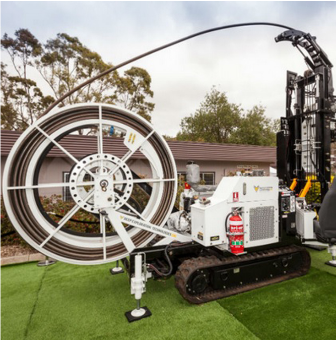
FIGURE 8.6 The coiled tubing drilling rig. Source: Courtesy from DET CRC.
