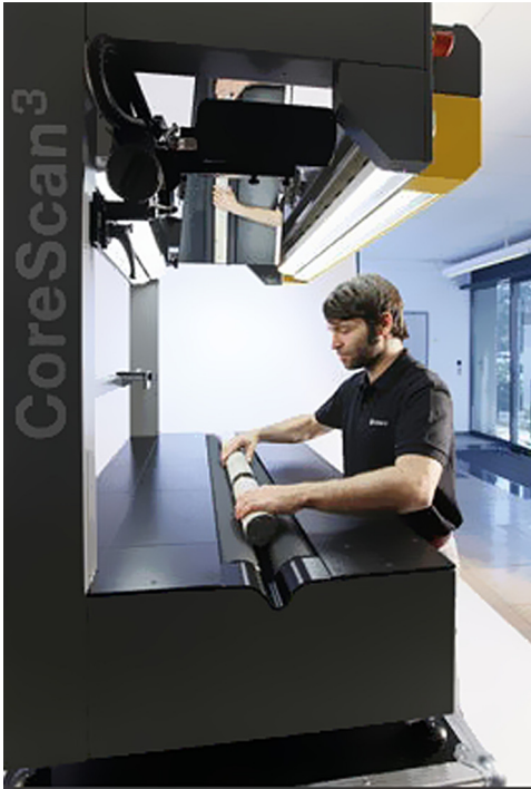
FIGURE 8.10 High-tech drill core scanner. Source: Courtesy from DMT CoreScan.
