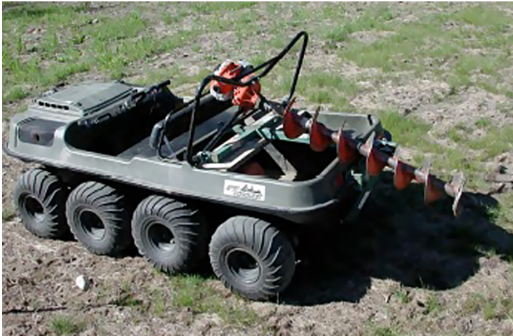
FIGURE 8.2 Large diameter mobile auger drilling machine. Source: Photo by Jacob.
