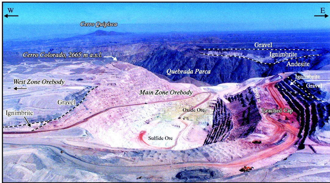
FIGURE 3.5 Panoramic view of Cerro Colorado porphyry copper deposit, Chile, showing various zones. Courtesy: BHP Billiton.
