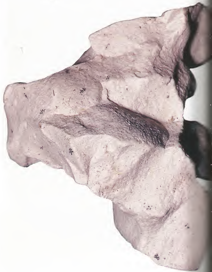
Above: A compact aggregate of montmorillonite, which is usually white but may be colored by impurities.
