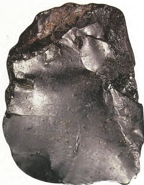
Above: The edges of this bitumen specimen resemble the edges of a seashell—this is known as conchoidal fracture.
