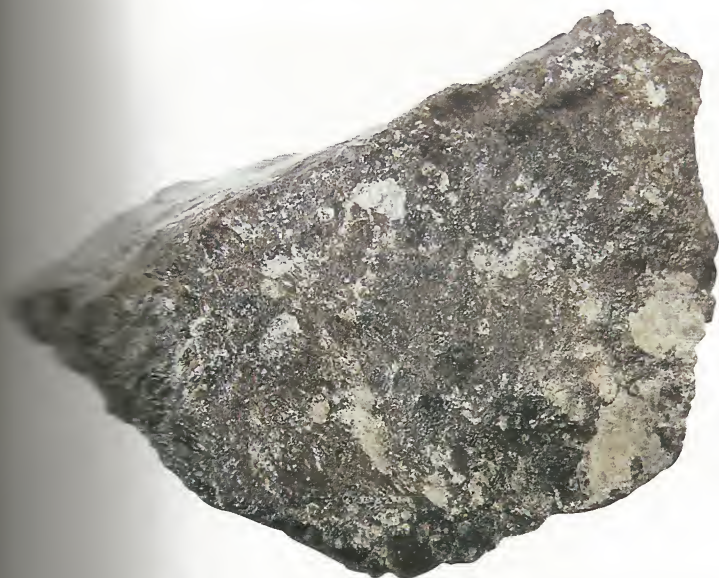
Above: This massive aggregate of columbite may also contain significant quantities of the closely related tantalite.
