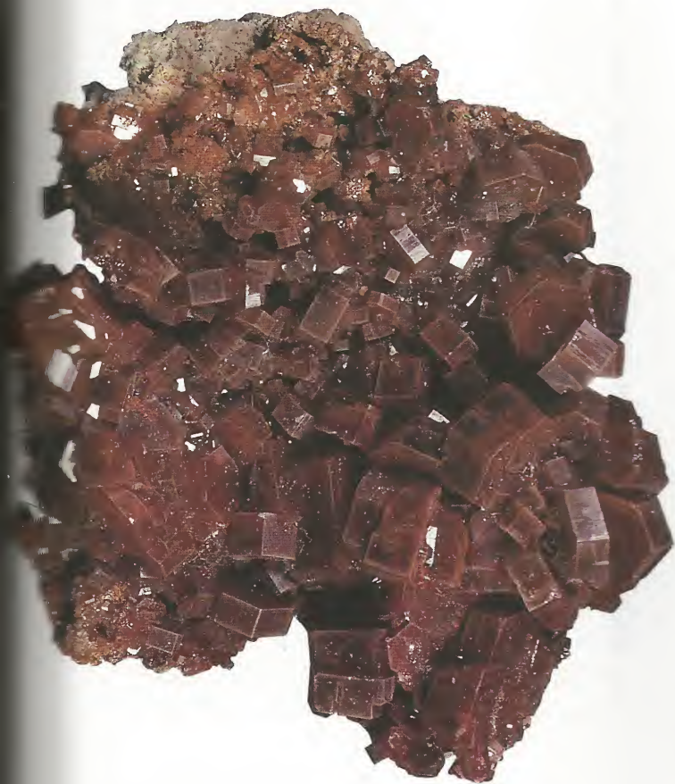
Above: A mass of stubby prismatic vanadinite crystals with hexagonal outlines.
