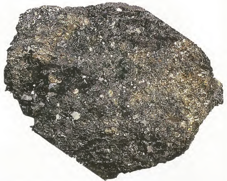
Above: A mass of ludwigite showing the characteristic grayish black color and silky luster.
