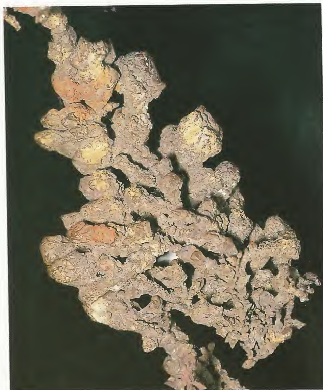
Above: Specimens like this aggregate of copper with vaguely treelike shapes are said to be dendritic.
