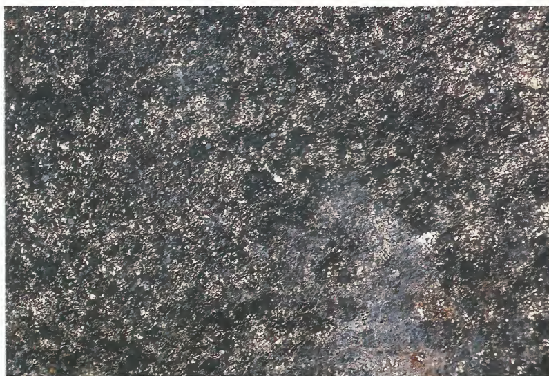
Above: This massive aggregate of pentlandite was extracted from a basic igneous rock formation. Note the metallic luster and the signs of uneven fracture.
