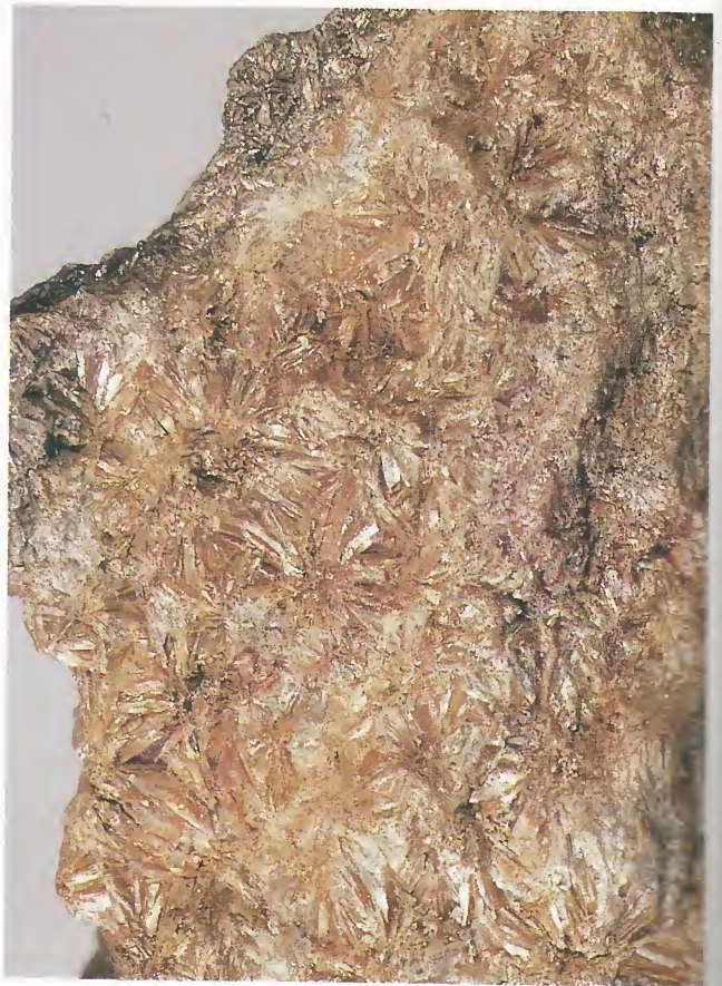
Above: Radiating masses of brown pyrophyllite crystals with a vitreous luster.
