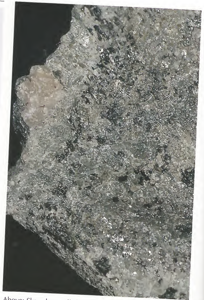
Above: Skarn has well-shaped (euhedral) crystals of numerous mineral types.
