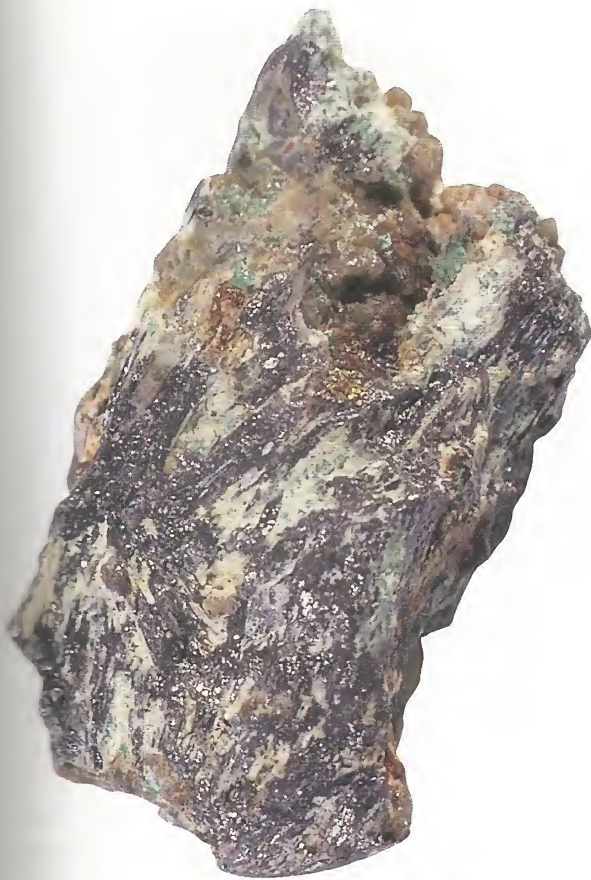
Above: Most bismuthinite is lead gray. It is an opaque mineral with a metallic luster.
