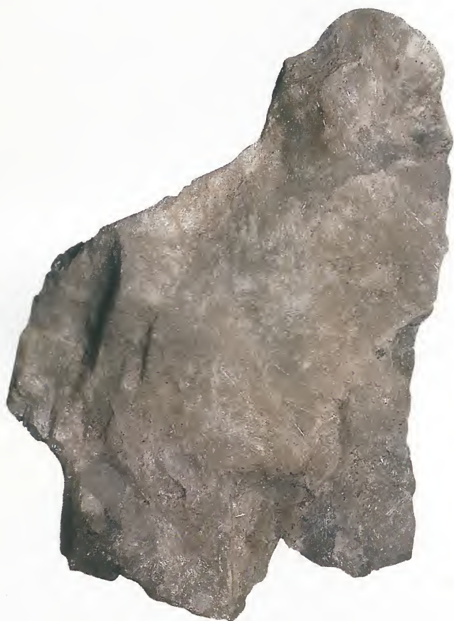
Left: A fibrous mass of sillimanite composed of tiny crystals that are all prismatic and almost square in cross-section.
