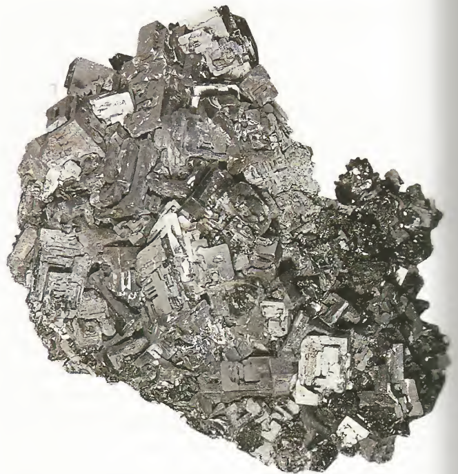
Above: Cubic crystals of galena. Note the bright metallic luster and the clearly defined lines of cleavage.
