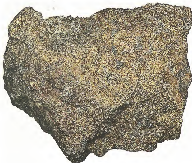
Above: A compact aggregate of chalcopyrite showing the characteristic brassy yellow coloration of this mineral.
