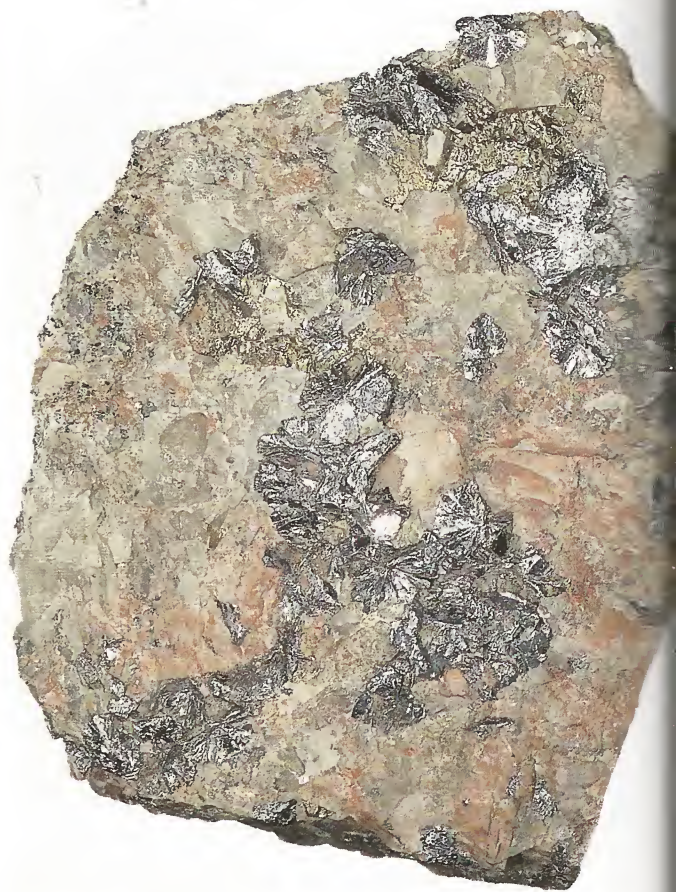
Above: Scaly gray crystals of molybdenite on a groundmass of granite rock.
