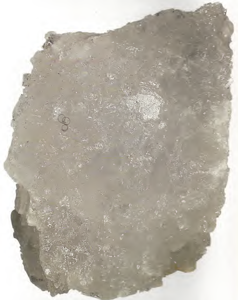
Above: This sylvite specimen is composed of tiny, interlocking cubic crystals.
