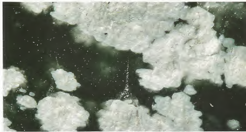
Above: White crystals of cristobalite on a groundmass of volcanic rock.
