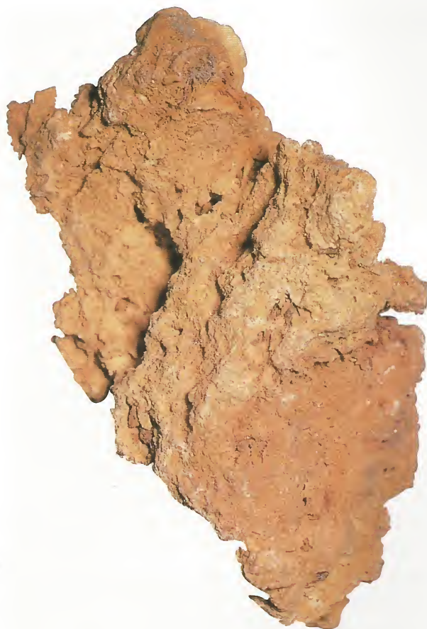
Above: The color of jarosite can range from an earthy dark brown to a yellowish or reddish brown, as in this specimen.
