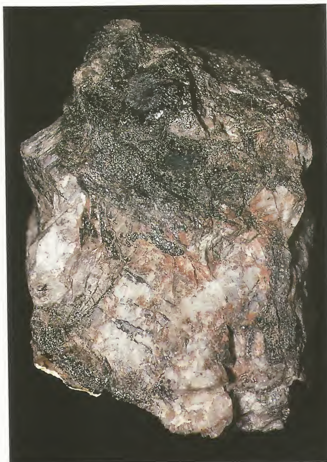
Above: This gadolinite has no clear overall shape—deposits such as this are known as massive aggregates.
