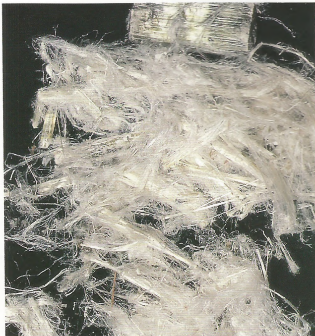
Above: Long, fibrous (acicular) crystals of actinolite.
