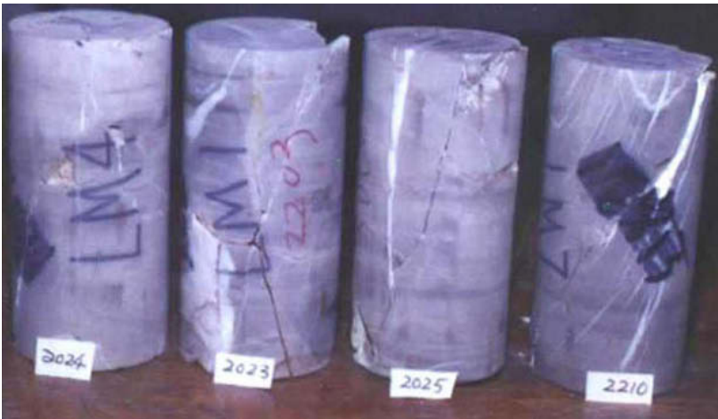
Fig. 4.17. Shear failure induced by the axial compressive loading in limestone samples.
