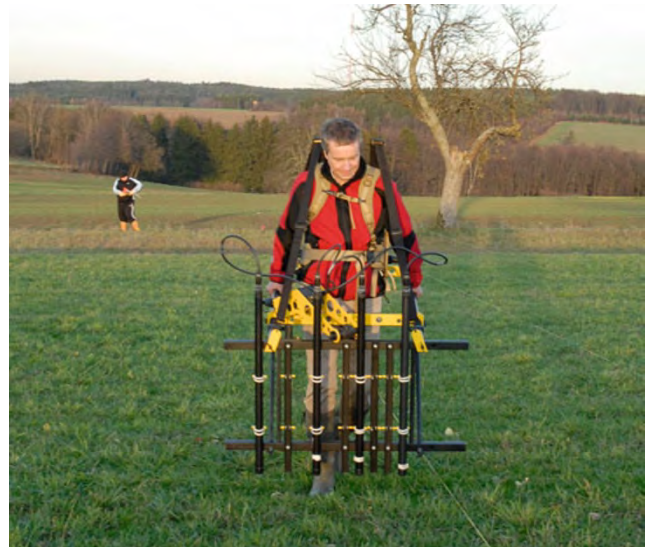
Magnetic Gradiometry, Figure 1 The four-channel fluxgate gradiometer of the Institute Dr. Foerster, Reutlingen, Germany. Measurements in a grid of 0.05 by 0.06 m are possible with this device. The two fluxgate sensors are 0.65 m apart.
