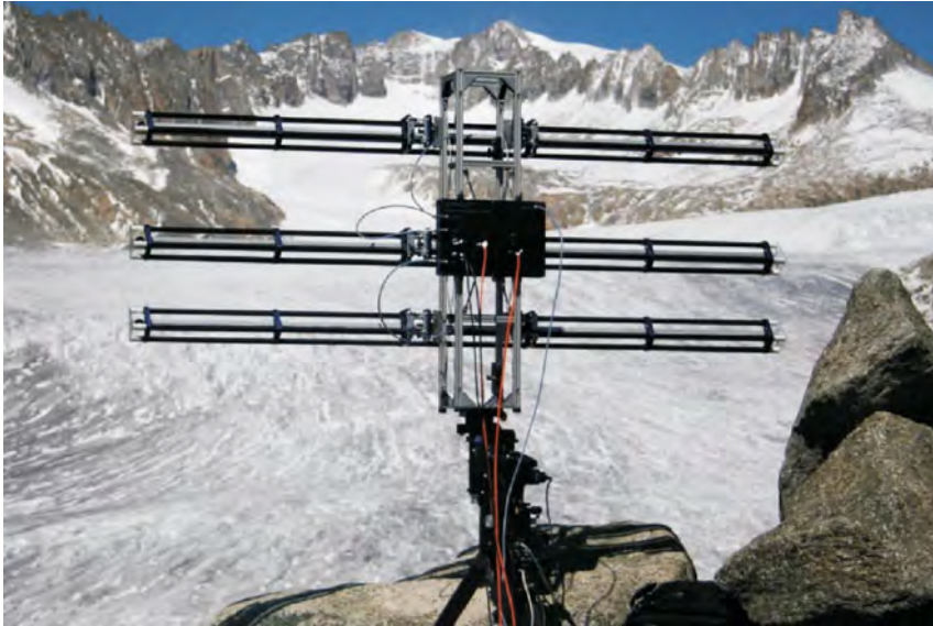
Geodesy, Ground Positioning and Leveling, Figure 4 A ground-based interferometric radar system to monitor deformation.
