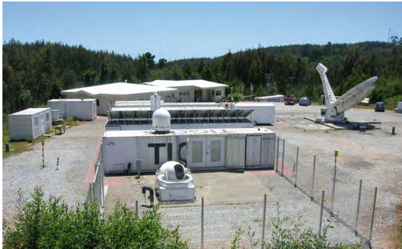
Geodesy, Networks and Reference Systems, Figure 2 The Transportable Integrated Geodetic Observatory (TIGO) in Concepción, Chile. The foreground shows the Satellite Laser Ranging (SLR)-System, behind it a pillar with Global Navigation Satellite Systems (GNSS)-antennas, and on the right the Very Long Baseline Interferometry (VLBI) radio telescope. All geodetic space techniques are placed at one site to define reference points for the global reference frame ITRF. The space vectors between the different instruments can be measured by a local survey. Not visible are the gravity meter and atomic clocks that are part of TIGO.
