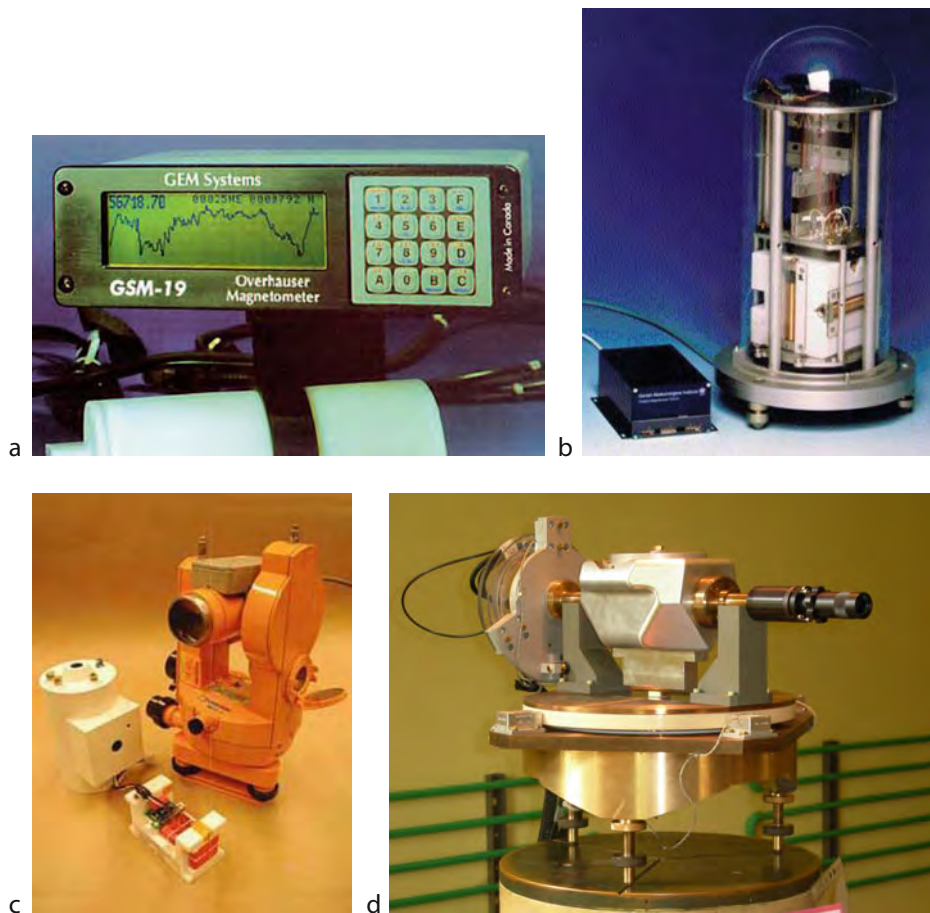
Geomagnetic Field, Measurement Techniques, Figure 1 Geomagnetic observatory sensor package: proton magnetometer (a), fluxgate magnetometer (b), theodolite with fluxgate coupled to the telescope (c). The new prototype of Geomagnetic AUtomed SyStem (GAUSS) is also shown (d).
