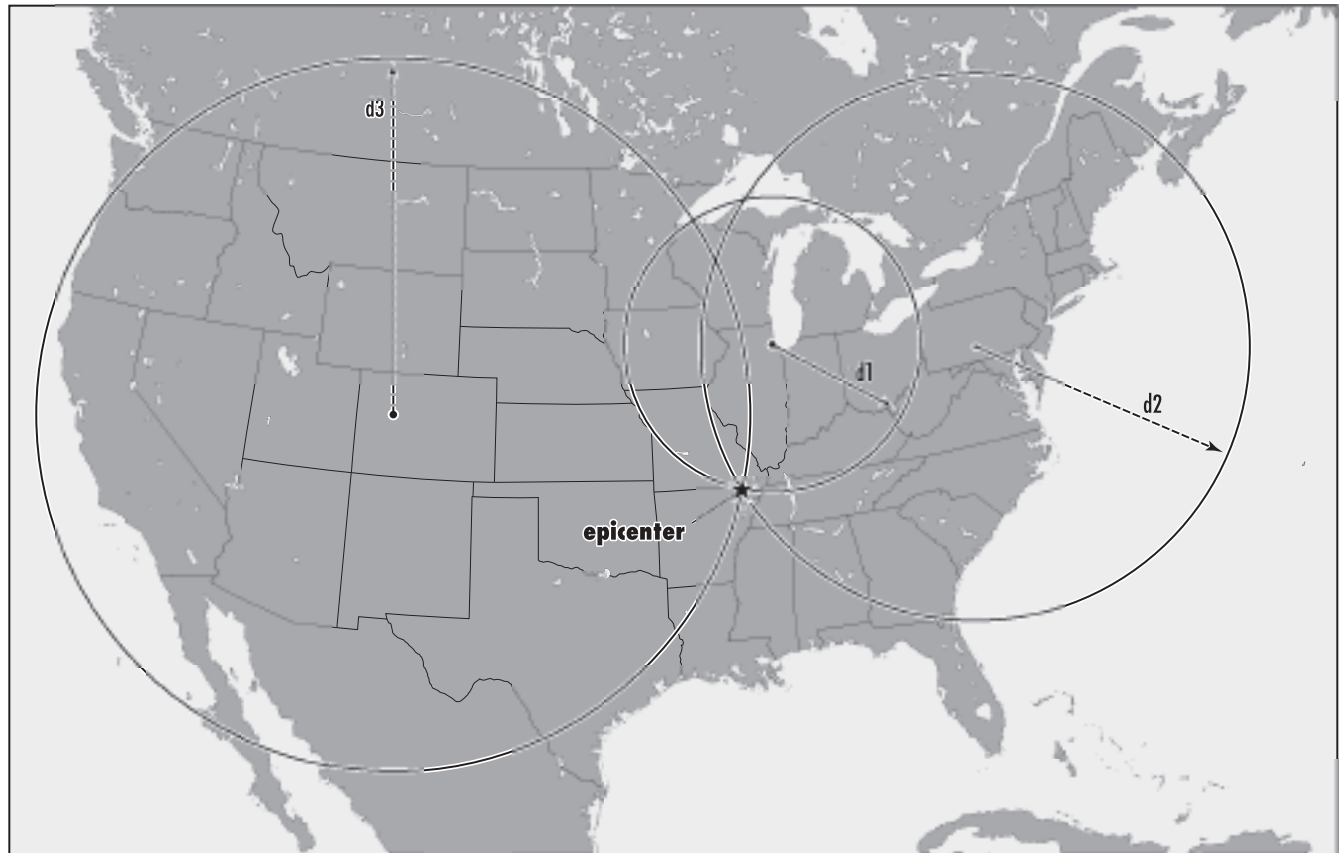
A method of locating earthquake epicenters is by calculating the distance to the source from three different seismic stations. The distance to the epicenter is calculated using the time difference between the first arrivals of P and S waves. The unique place where the three distance circles intersect is the location of the epicenter.
