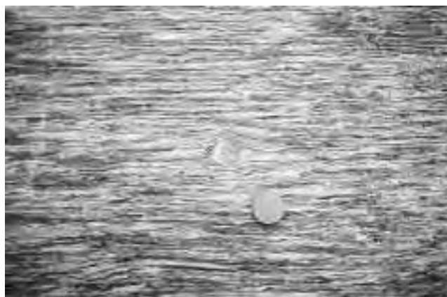
Granitic mylonite showing large porphyroclasts (relict feldspar grains) and mylonitic foliation (from 1-billion-year-old shear zone in Parry Sound, southern Canada) (Photo by Timothy Kusky)
