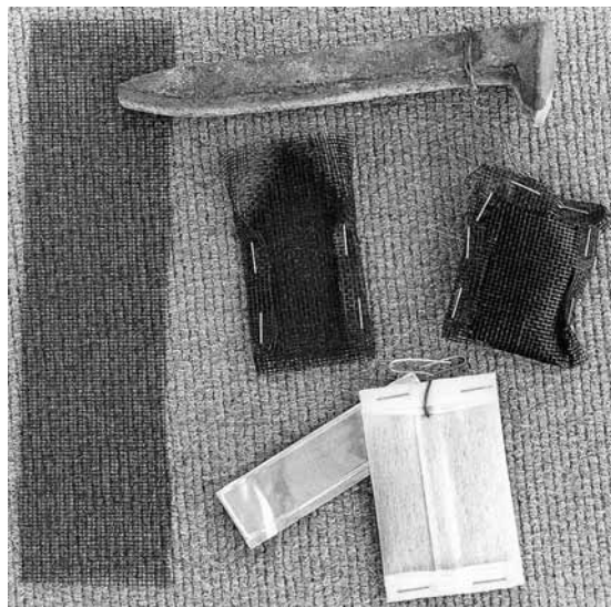
FIGURE 1 Photo showing construction of a passive carbon detector (Dunn Bug). Plastic window screen material is cut into strips, folded, and stapled. The envelope is filled with activated carbon and the top is folded and stapled. An old railroad spike makes a convenient anchor which is attached with copper wire. Another envelope material suggested by Calvin Alexander is cut from a “milk sock” available from farm supply stores (lower right).
