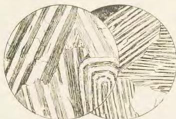
FIG. 61.—LAMELLAR TWINNING IN PLAGIOCLASE. Between crossed nicols.
