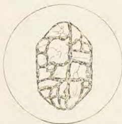
FIG. 66.—OLIVINE ALTERING INTO SERPENTINE.
