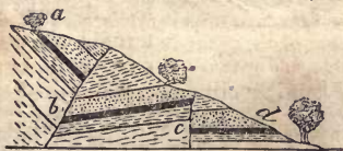
Fig. 258.—Bed dislocated by faults.
