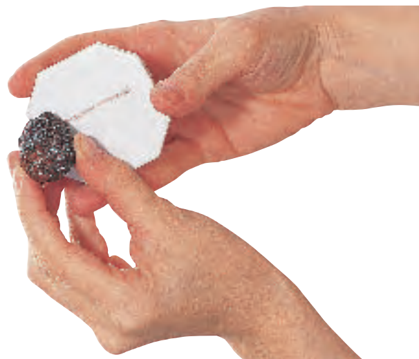
Figure 9 Streak is more useful for mineral identification than is mineral color. Hematite, for example, can be dark red, gray, or silver in color. However, its streak is always dark reddish-brown.
