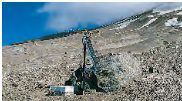
Figure 5 This USGS solar-powered seismograph records small earthquakes on the flank of the Augustine volcano in Alaska.
