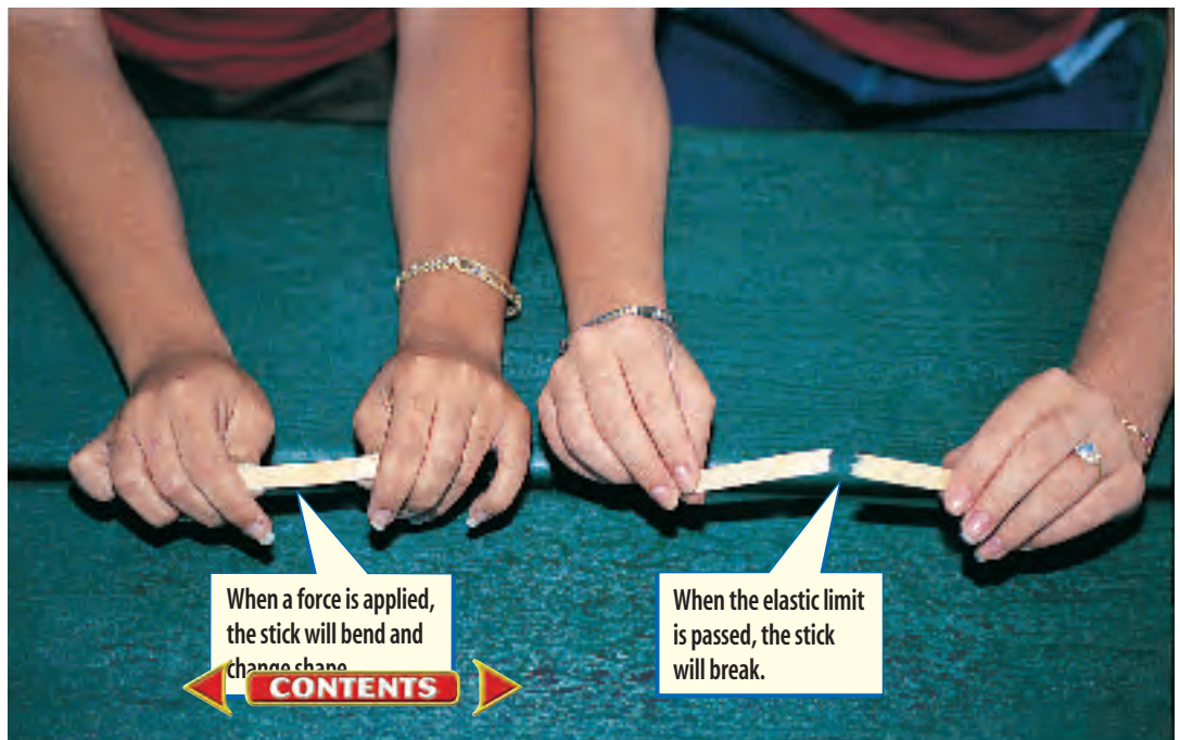
Figure 1 The bending and breaking of wooden craft sticks are similar to how rocks bend and break.
