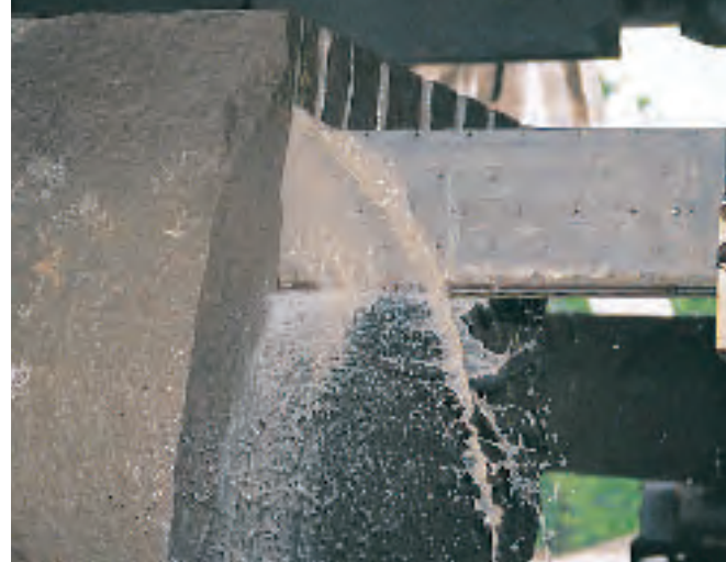
Figure 7 Some saw blades have diamonds embedded in them to help slice through materials, such as this limestone. Blades are kept cool by running water over them.
