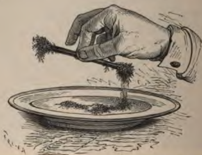
MAGNETIZED BAR, WITH IRON FILINGS ADHERING TO ITS TWO POLES.
