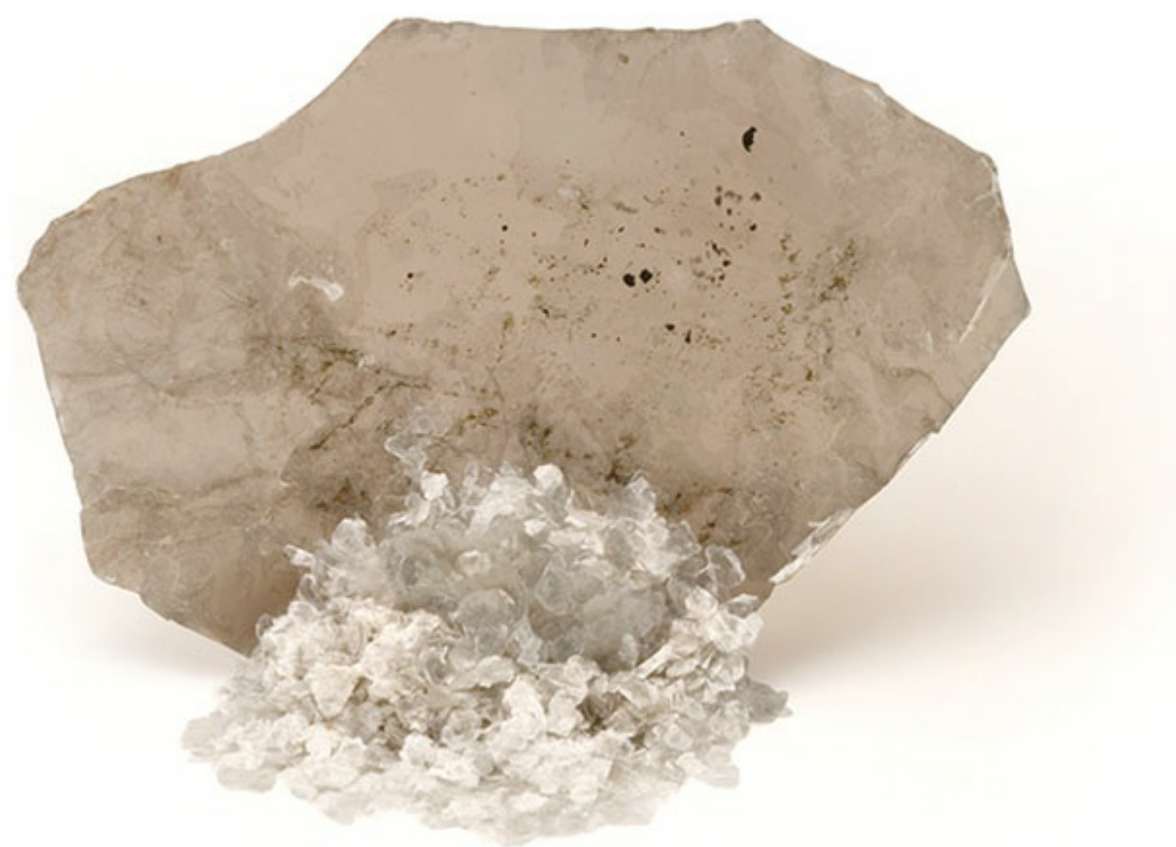
Figure 3.13 A large sheet of muscovite mica, which, when crushed, produces many smaller flaky fragments as a result of excellent basal cleavage.
