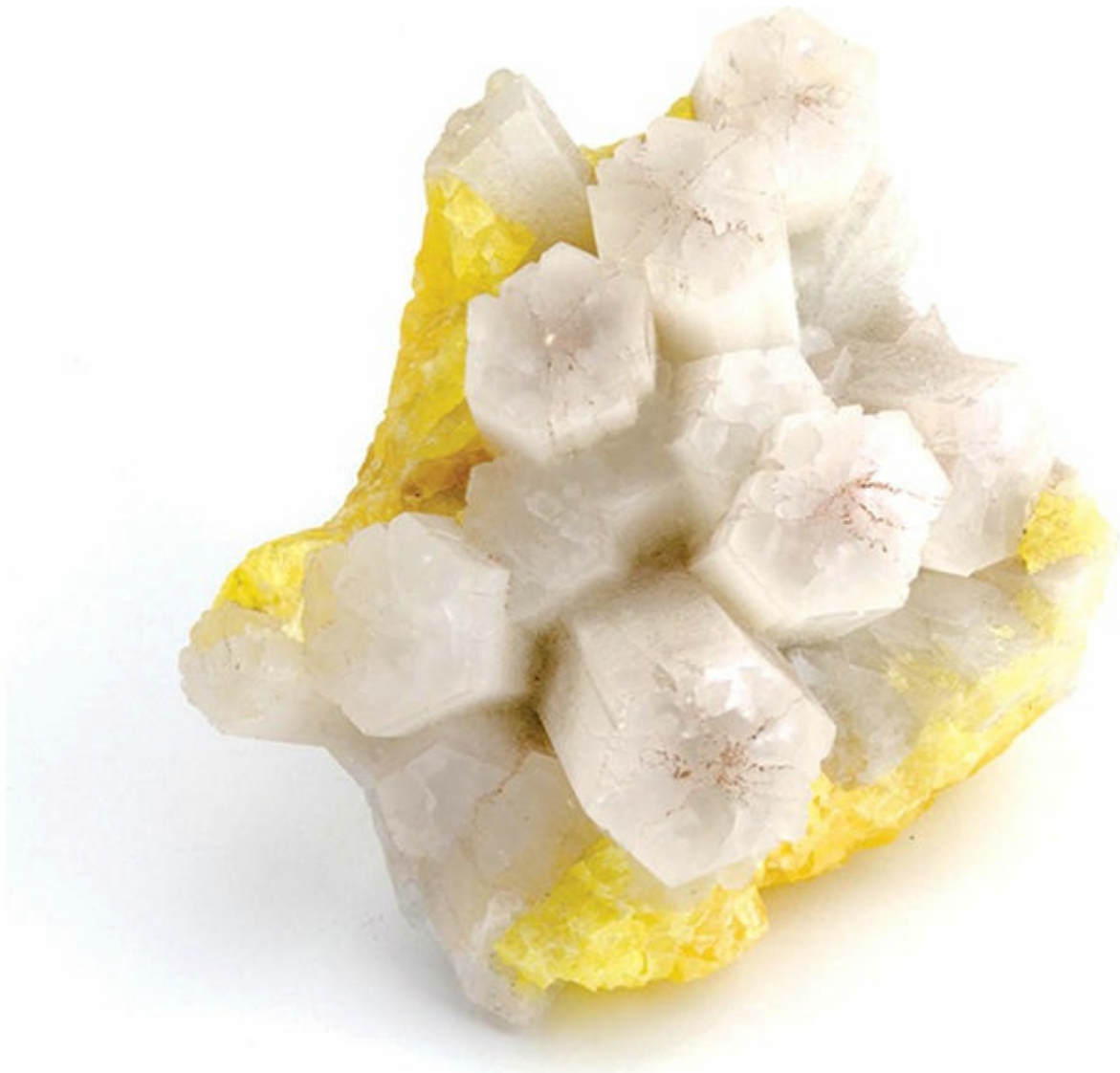
Figure 10.14 A cluster of white pseudo-hexagonal twins of aragonite forming a hexagonal-like prism terminated by a basal plane. This results from the intergrowth of three individual aragonite crystals twinned on \{110\} forming cyclic twins. The yellow mineral in the background is sulfur.
