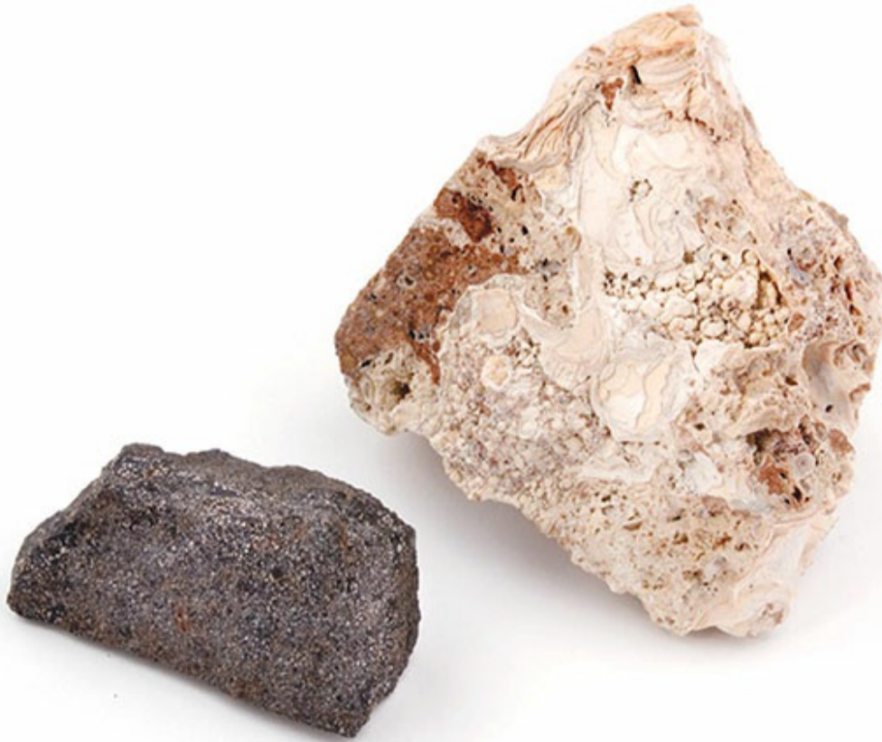
Figure 10.31 On the left, a black, granular hand specimen of phosphorite (the dark color is probably due to inclusions of organic matter); on the right, a phosphatic (apatite-rich) limestone.
