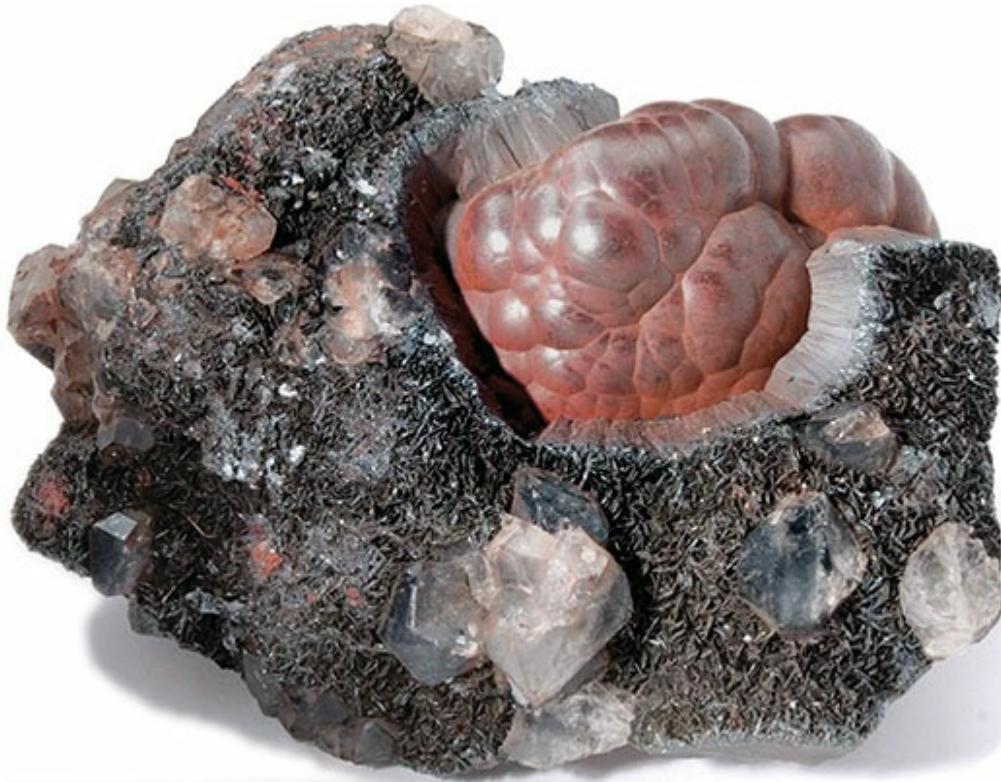
Figure 7.49 Hematite in two different forms: as fine platy crystals with a metallic luster and as a reddish-brown botryoidal mass. The whitish translucent, glassy crystals are quartz.
