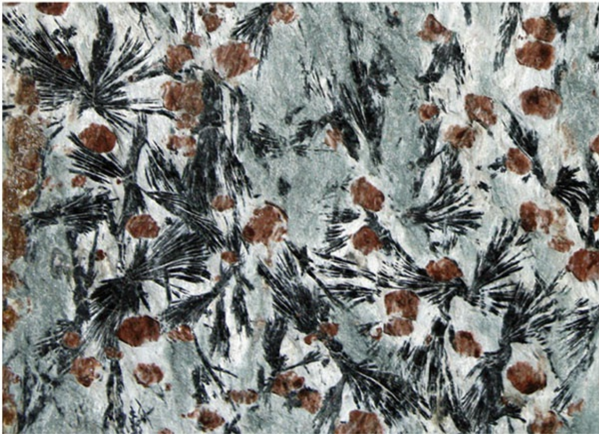
Figure 14.10 Mica-garnet-hornblende schist of the Ordovician Hawley Formation of western Massachusetts with sheaflike clusters of hornblende (garbenschiefer). This rock is the same as the one shown on the cover of the book.
