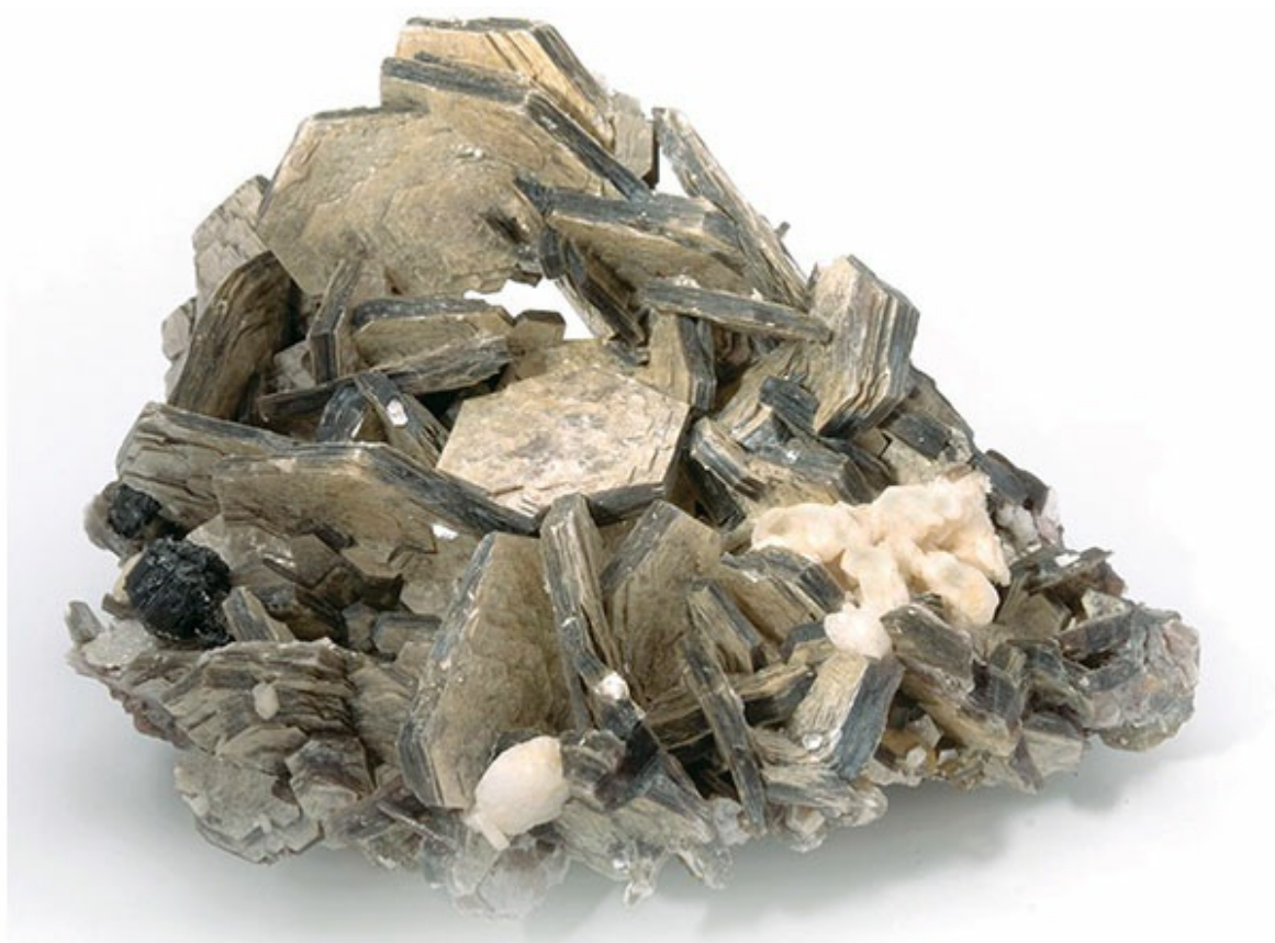
Figure 7.30 Randomly intergrown cluster of well-formed tabular crystals of muscovite with pseudo-hexagonal outlines. These are referred to as pseudo-hexagonal because the underlying structure of muscovite is monoclinic.
