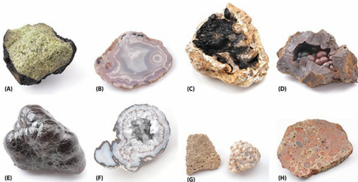
Figure 3.2 Photographic illustrations of many of the states of aggregation listed in Section 3.2. (A) Granular grains of yellow-green olivine in a volcanic bomb of dunite (a rock type made up essentially of olivine). (B) Finely banded as in this polished slab of agate. (C) Botryoidal, as shown by the outer, almost-black
