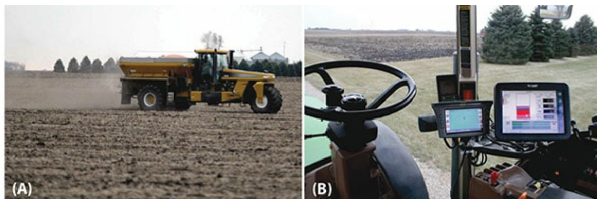
Figure 17.3 (A) A modern farm vehicle carrying three separate sources of nitrogen, phosphorus, and potassium fertilizer that are blended and applied at a specified rate determined by the vehicle's position as determined by a global position system (GPS). (B) Interior of the cab of a modern farm vehicle showing the GPS unit, which actually governs the navigation of the vehicle on the left and the computer controlling the mixing and application of fertilizer and seeds on the right. (Photographs courtesy of Merlin Anderson.)
