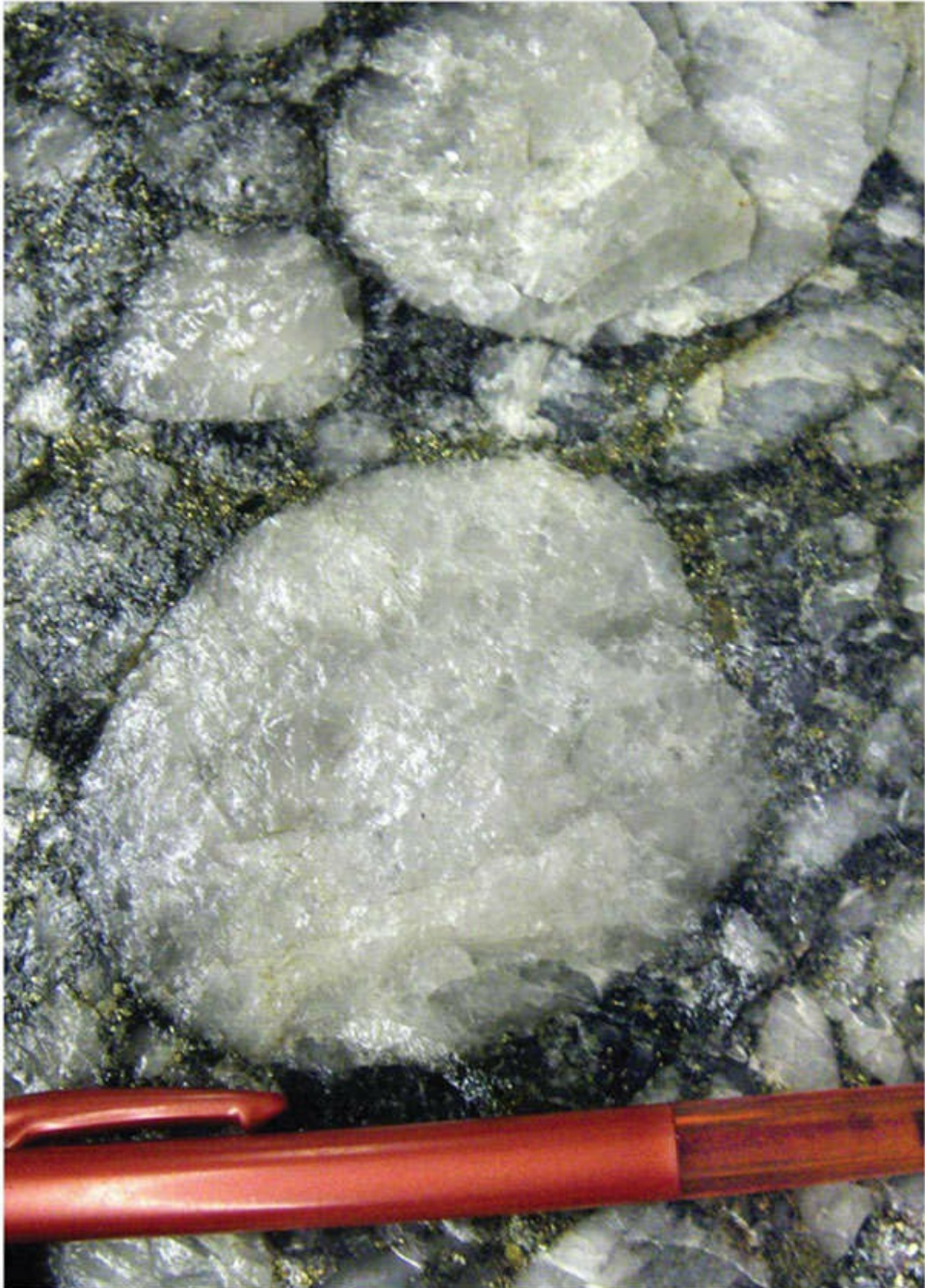
Figure 12.17 The 2.9 billion-year-old Witwatersrand oligomict clast-supported quartz conglomerate of South Africa hosts one of the world's richest gold deposits. The gold, occurs with pyrite between the quartz pebbles. (Photograph courtesy of Grant Cawthorn.)
