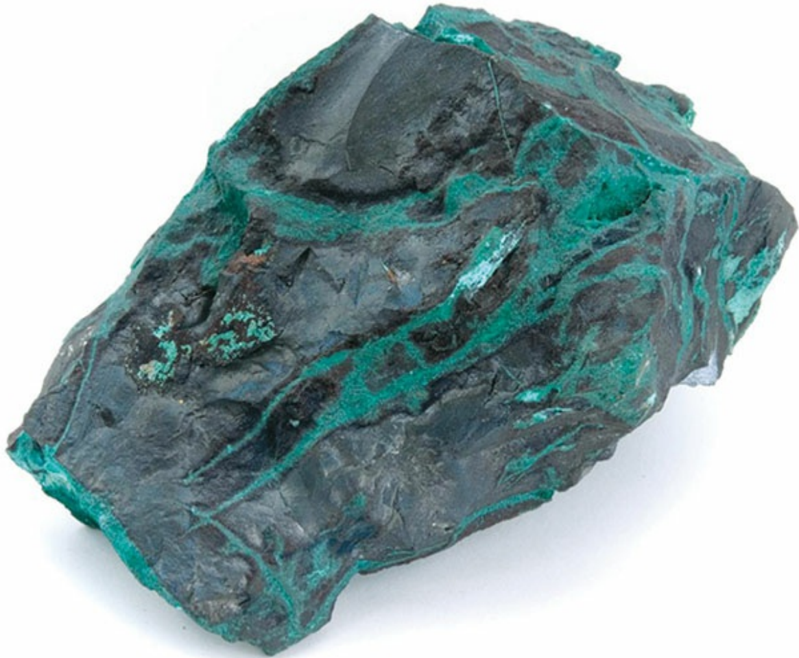
Figure 15.16 Massive black chalcocite with fractures filled by dark-green brochantite, Cu_4SO_4(OH)_6 , an alteration product.
