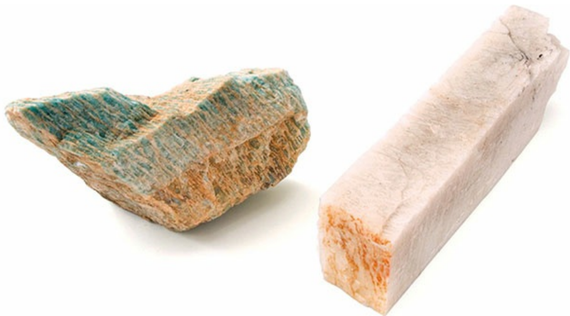
Figure 7.9 On the left, a hand specimen of green perthitic microcline (known as amazonite); on the right, a perfect, blocky cleavage fragment of orthoclase.
