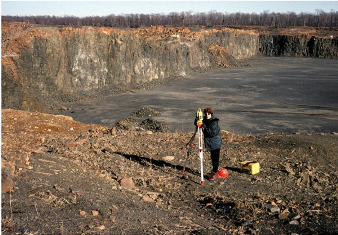
Figure 2.9 The active north face of Tilcon's North Branford quarry, Connecticut, where a thick basaltic lava flow is quarried for its extremely durable rock that is used as aggregate and mixed with asphalt to pave roads. This quarry produces 20 000 tons of crushed trap-rock aggregate per day.
