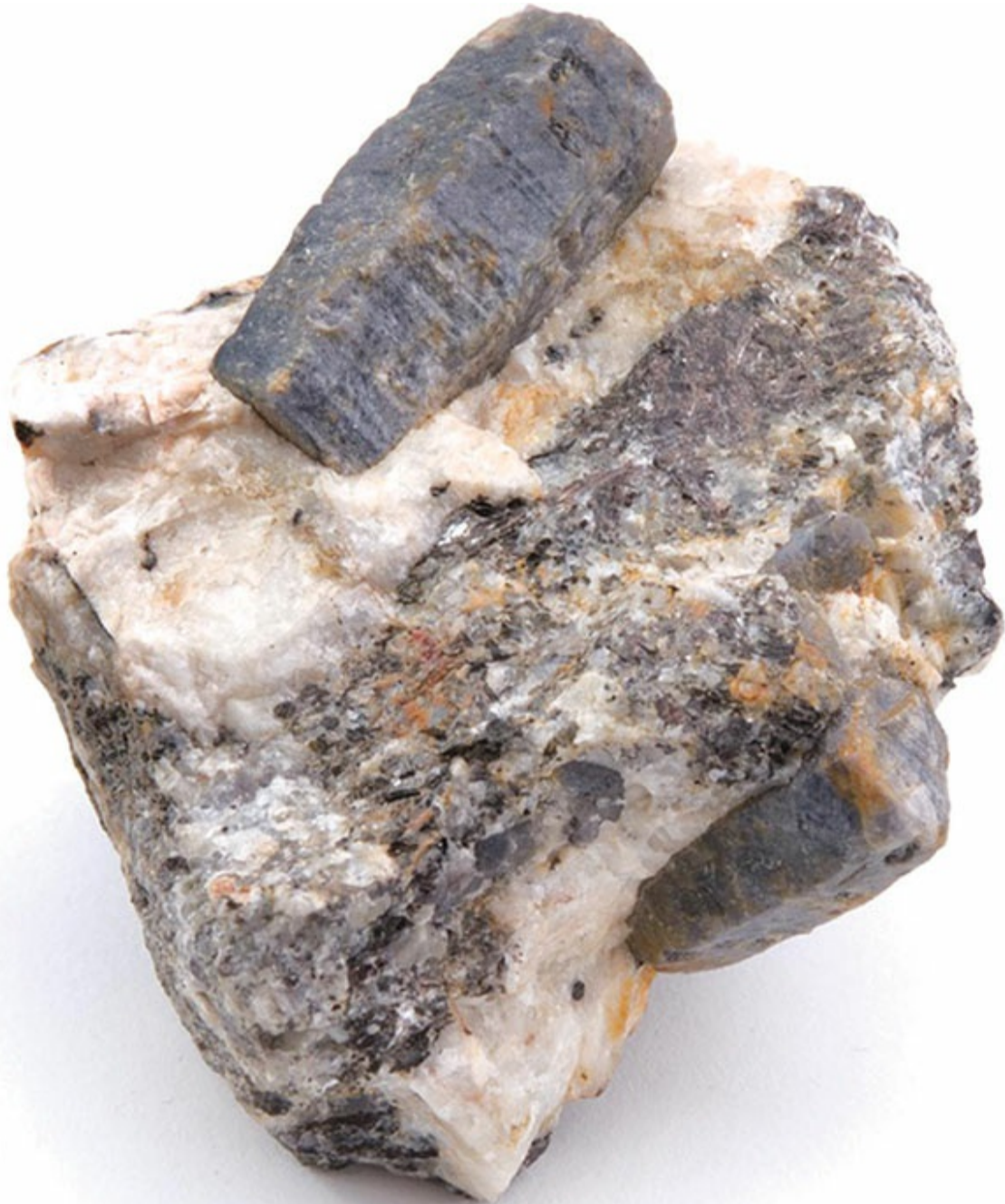
Figure 13.46 Bluish gray barrel-shaped dipyramidal crystals of corundum with horizontal striations. The white matrix mineral is feldspar.
