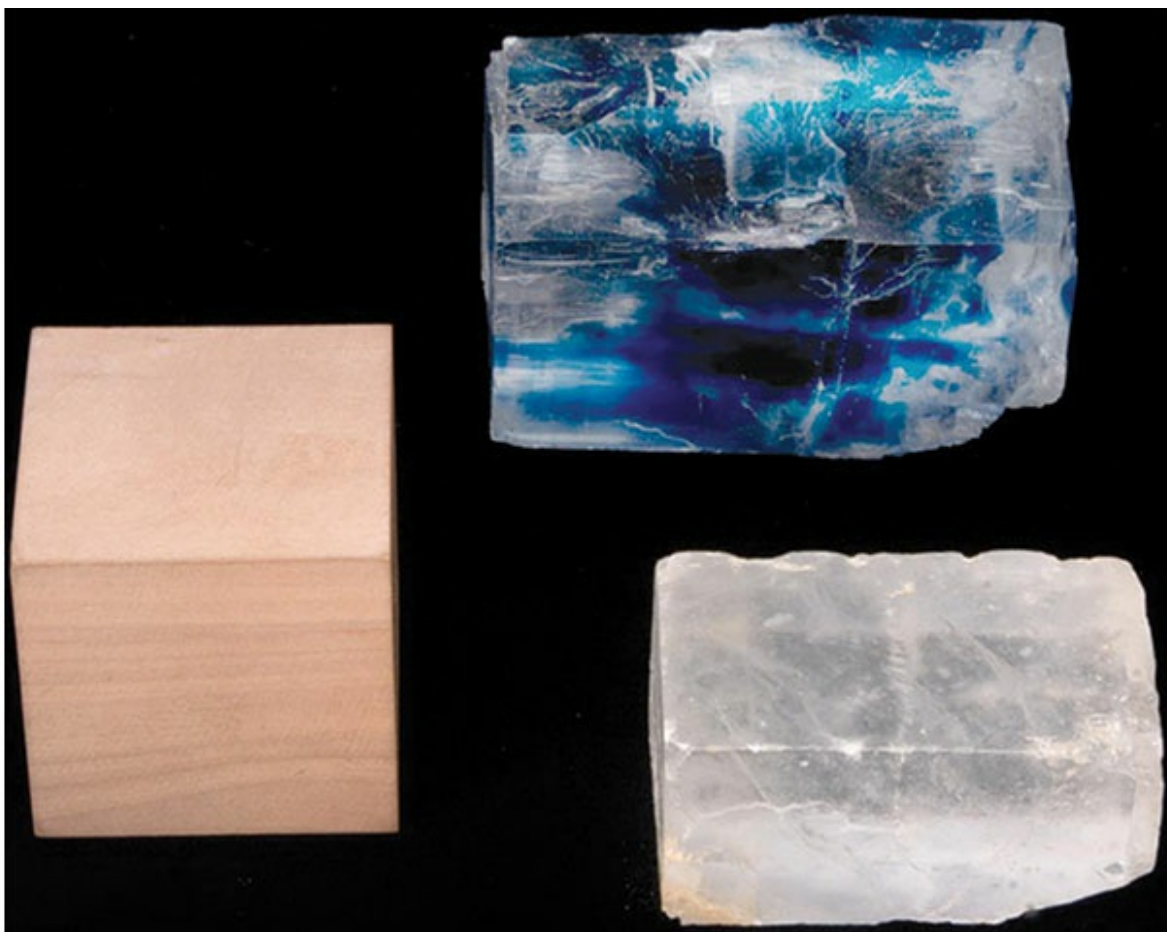
Figure 3.15 Excellent cubic cleavage (three cleavage directions at 90^\circ to one another) in halite, \text{NaCl} . Blue and white translucent cleavage fragments and a small wooden model of a cube.
