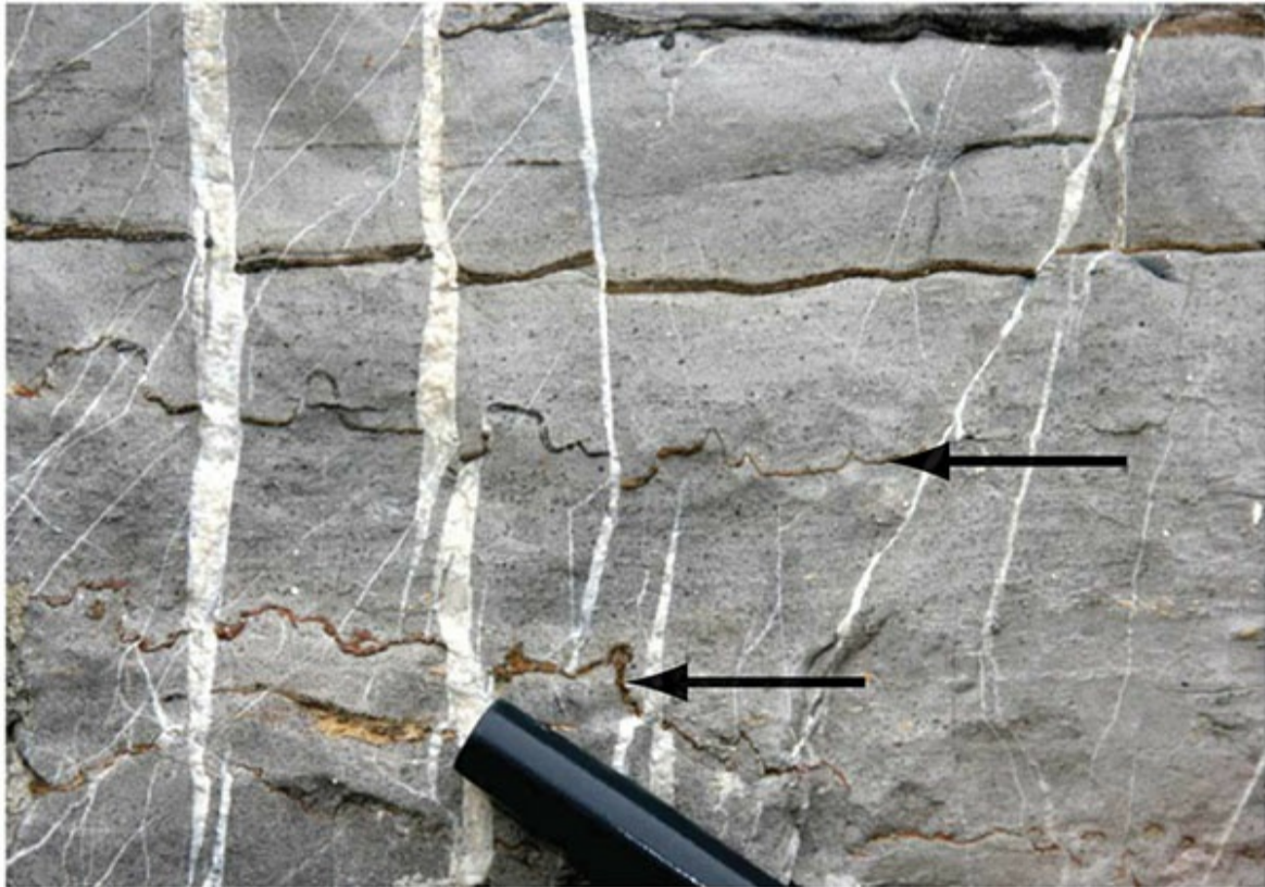
Figure 11.33 Horizontally bedded limestone in which vertical pressure solution generated irregular stylolites (arrows) parallel to bedding, and horizontal extension created white calcite veins along normal faults that are roughly perpendicular to bedding.
