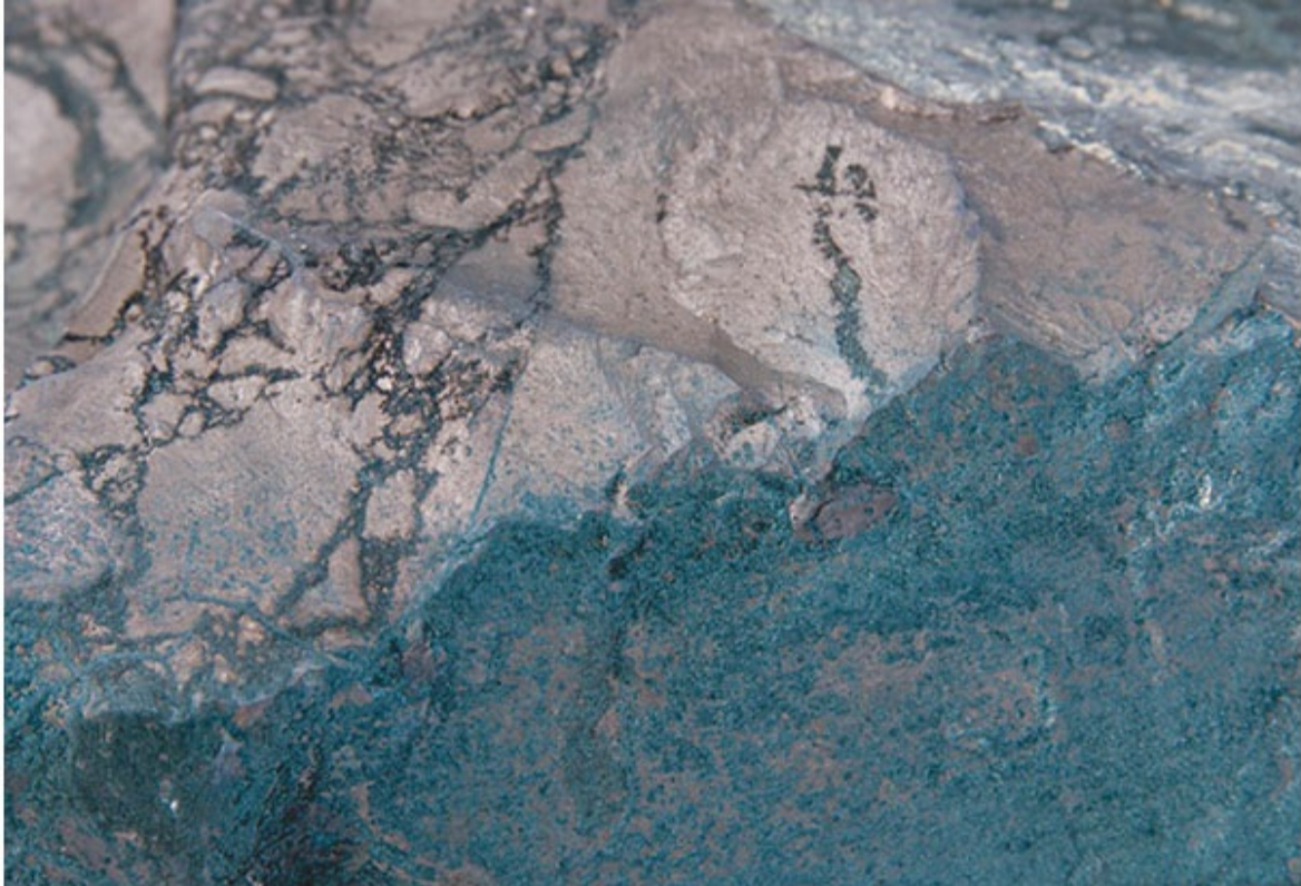
Figure 15.13 Massive bornite with a fresh surface of brownish-bronze color. The tarnished portion shows variegated purples and blues, also known as peacock ore.
