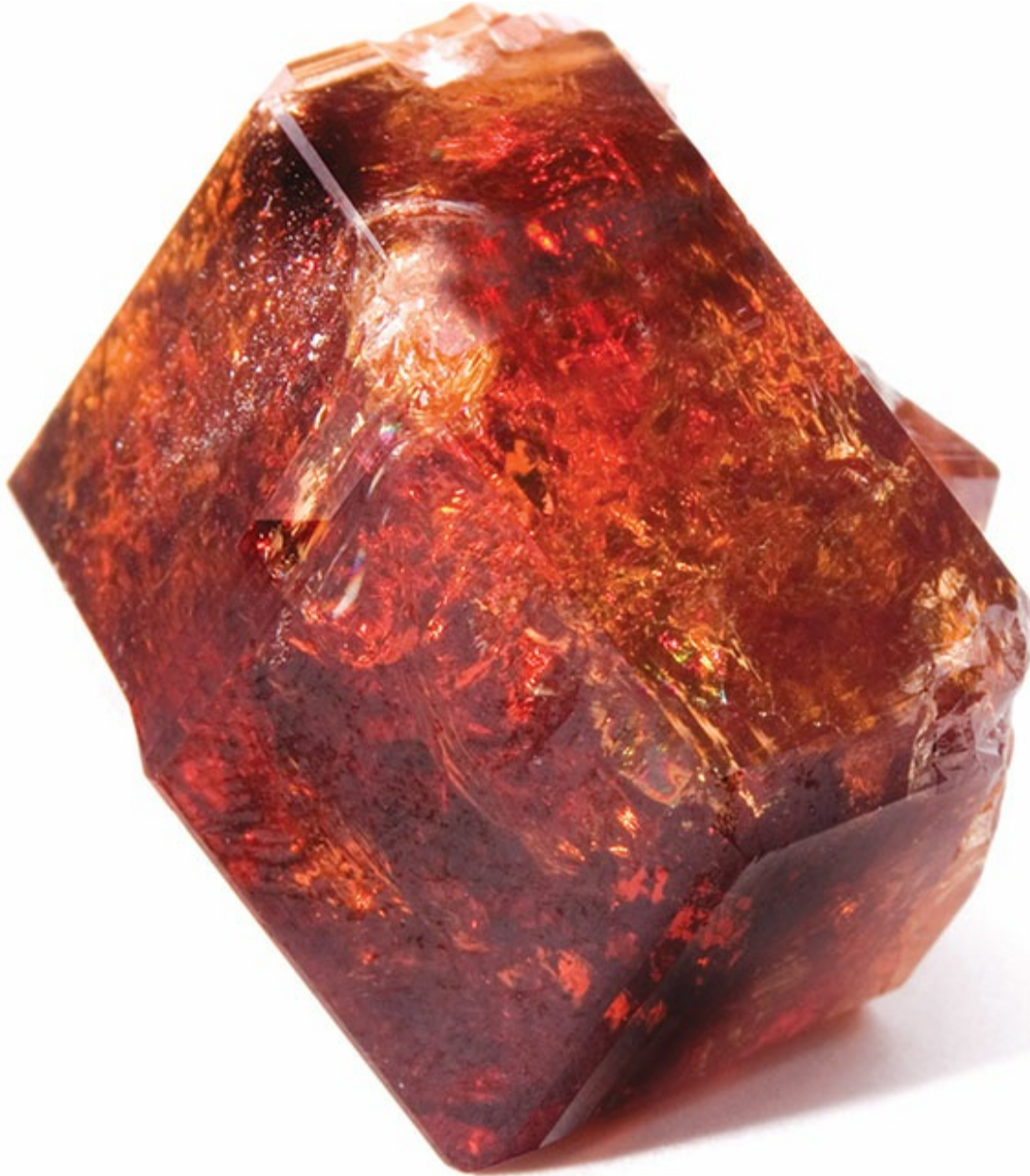
Figure 13.4 An orange-red, distorted dodecahedral crystal of grossular. Although this crystal has a most attractive color, it contains many imperfections (inclusions and microfractures), which makes it unusable as a gemstone.
