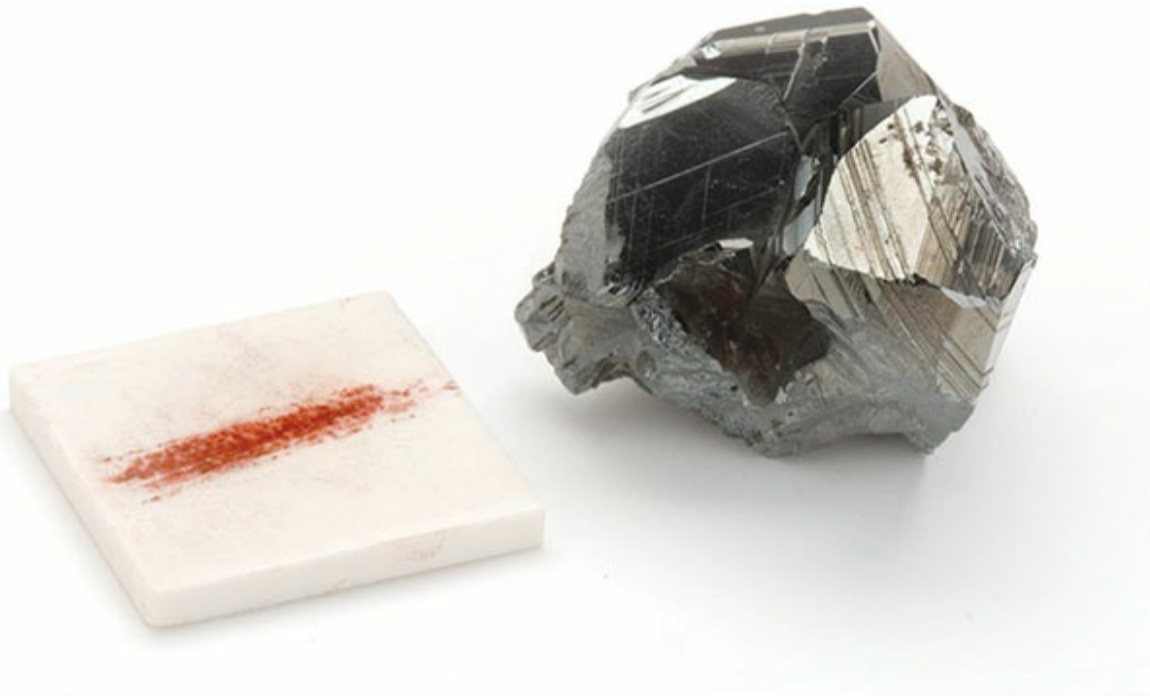
Figure 3.12 A black, metallic crystal of hematite, \text{Fe}_2\text{O}_3 . The streak of all hematite is red as shown on an unglazed porcelain plate.
