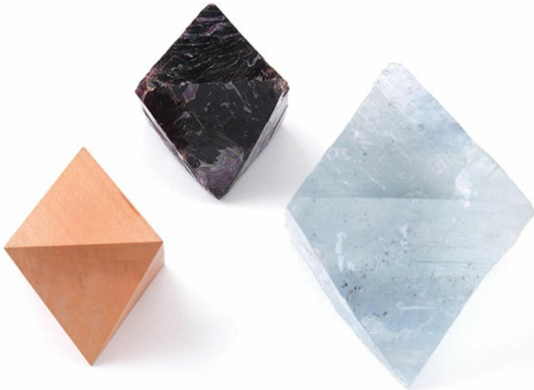
Figure 3.17 Excellent octahedral cleavage in fluorite, \text{CaF}_2 . The wooden octahedron illustrates the same four cleavage directions.
