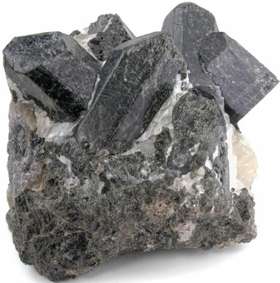
Figure 7.25 Dark green to black grouping of prismatic augite crystals.
