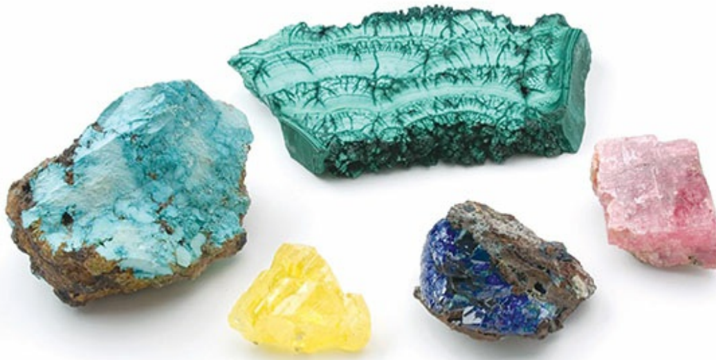
Figure 3.3 Examples of a few minerals that can be uniquely identified by their color. From left in a clockwise direction: turquoise, turquoise in color; malachite, green; rhodochrosite, pink; lazurite, blue (known in the gem trade as lapis lazuli); and sulfur, yellow.
