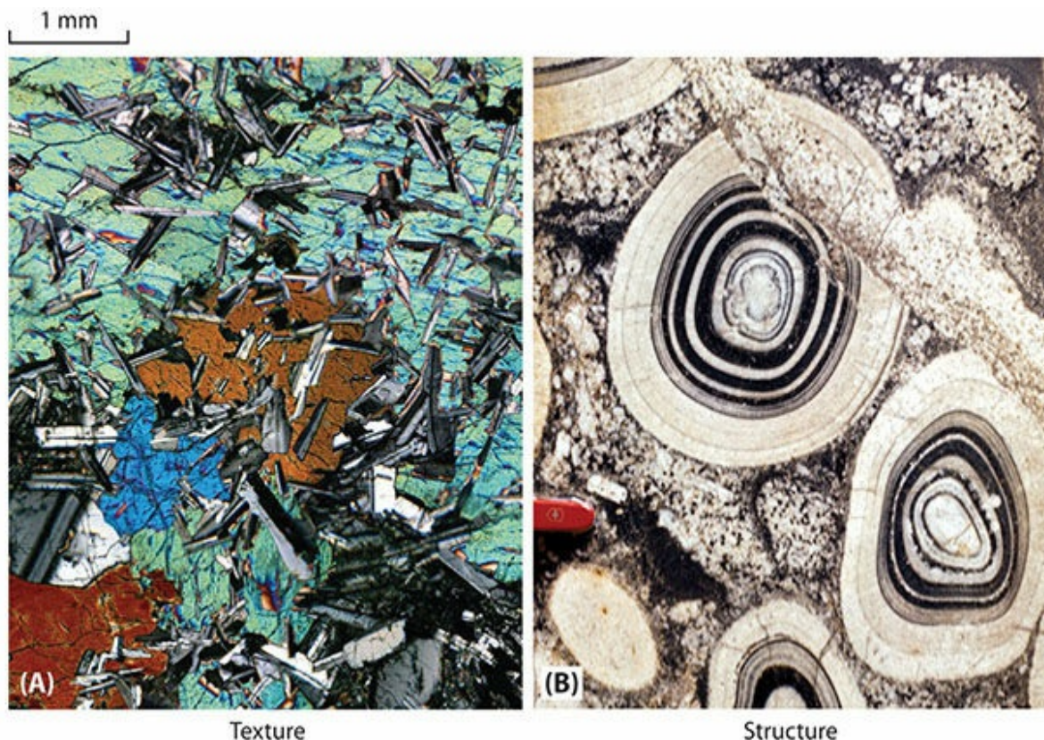
Figure 2.10 (A) Texture refers to the way individual mineral grains are intergrown. It is seen best in thin sections of the rock under a polarizing microscope, as seen here in this photomicrograph of a basaltic rock from the Bird River Sill, South Africa. This texture is described as ophitic, meaning that small plagioclase feldspar crystals (gray) are completely embedded in larger crystals of pyroxene (brightly colored grains). Photograph taken under crossed polarized light (see Chapter 6 for explanation of polarized light). (B) Structure
