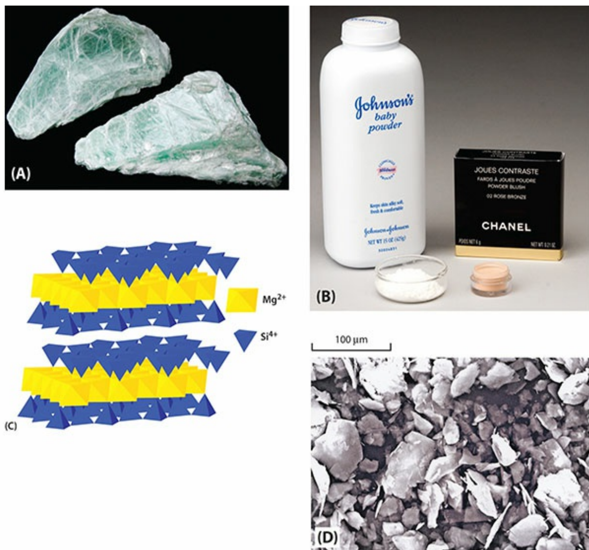
Figure 2.3 (A) Hand specimens of talc, \text{Mg}_3\text{Si}_4\text{O}_{10}(\text{OH})_2 . (B) Commercial containers of baby (talcum) powder and cosmetic facial powder. Two dishes, with talc and facial powder, respectively. (C) A perspective view of the layered internal atomic structure of talc. The \text{Mg}^{2+} ions are sandwiched between two opposing sheets of (\text{SiO}_4)^{4-} tetrahedra. (D) Talcum powder from the Petri dish in (B) photographed by scanning electron microscope. This shows the somewhat variable grain size of the tiny (very soft) flakes at about 400 \times magnification. (Photograph courtesy of Adrian Brearley, University of New Mexico.)
