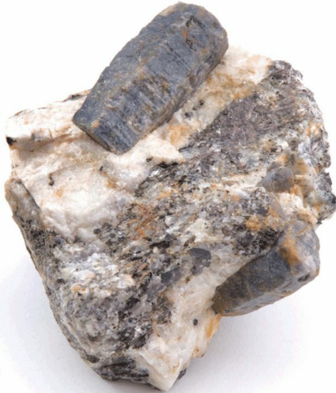
Figure 14.48 Bluish gray barrel-shaped dipyramidal crystals of corundum with horizontal striations. The white matrix mineral is feldspar.
