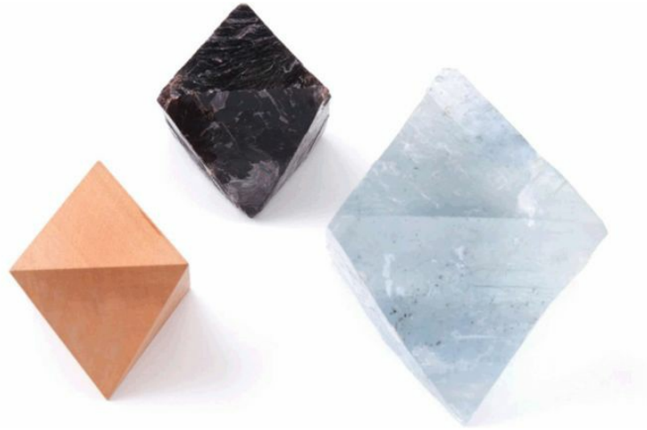
Figure 3.17 Excellent octahedral cleavage in fluorite, \text{CaF}_2 . The wooden octahedron illustrates the same four cleavage directions.
