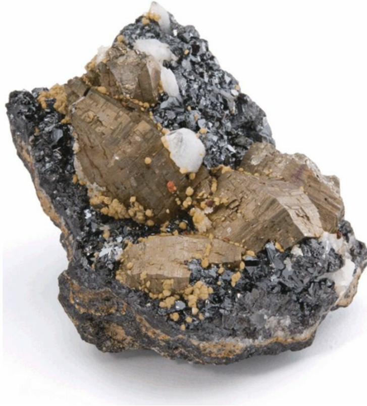
Figure 7.59 Dipyramidal crystals of pyrrhotite among smaller, almost black, crystals of Fe-rich sphalerite, and some white quartz overgrowths.
