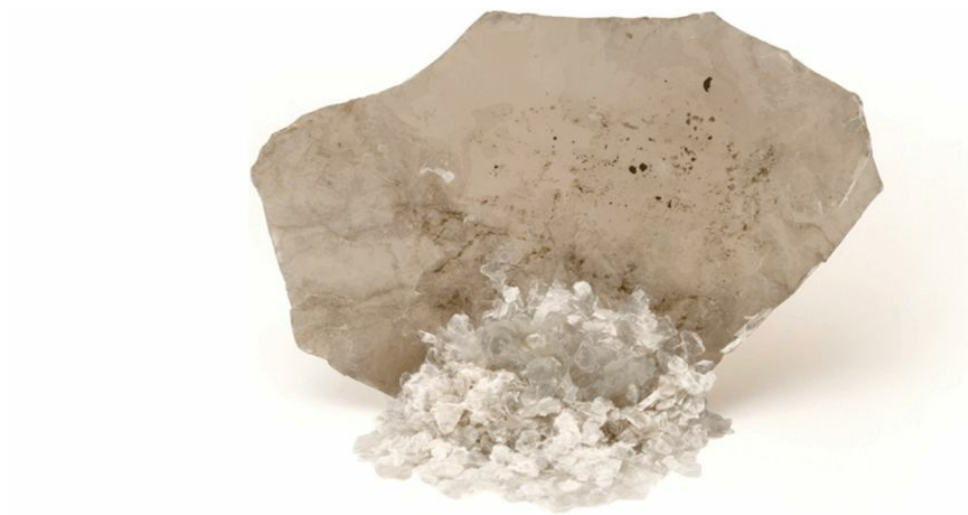
Figure 3.13 A large sheet of muscovite mica, which, when crushed, produces many smaller flaky fragments as a result of excellent basal cleavage.
