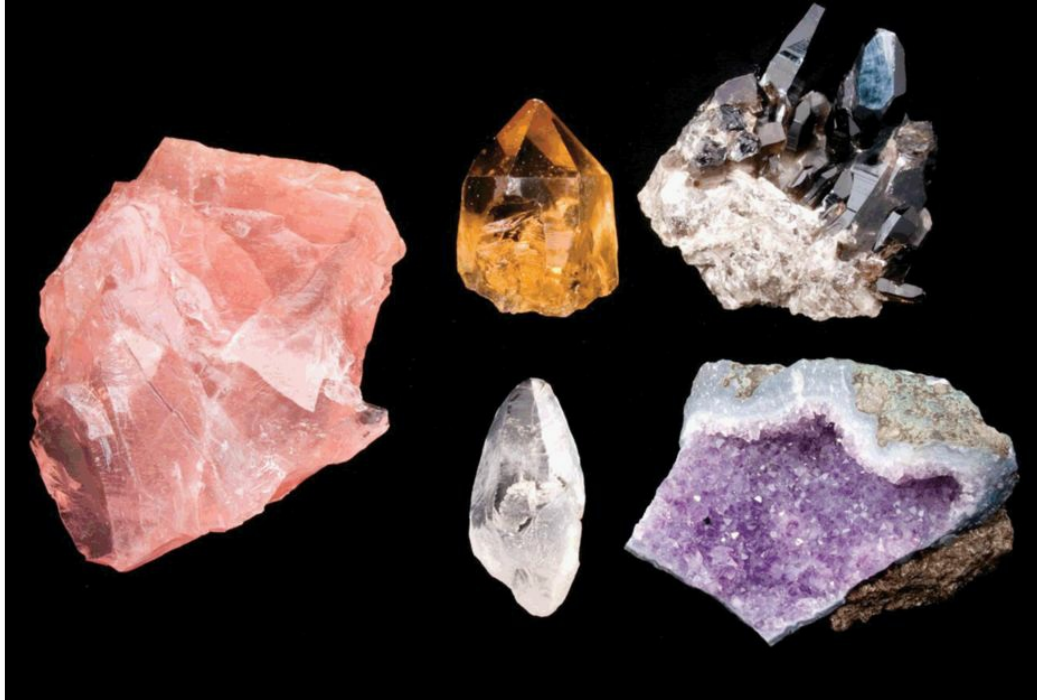
Figure 7.11 Hand specimens (clockwise from left to right) of rose quartz, citrine, smoky quartz, amethyst, and rock crystal (clear transparent quartz).
