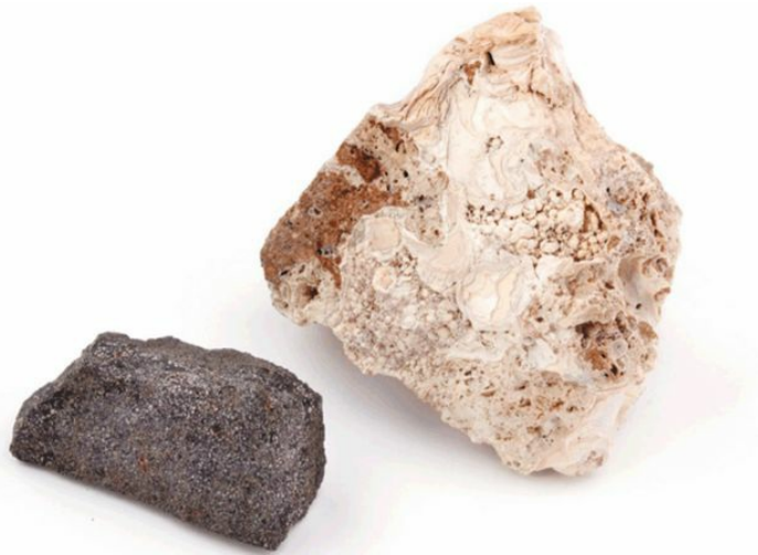
Figure 11.31 On the left, a black, granular hand specimen of phosphorite (the dark color is probably due to inclusions of organic matter); on the right, a phosphatic (apatite-rich) limestone.
