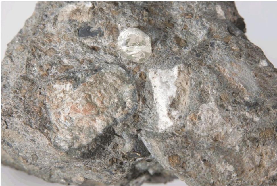
Figure 16.5 Clear, transparent, distorted octahedron of diamond (top center) in a matrix of kimberlite, which consists of angular fragments or xenoliths of mantle-derived rocks.
