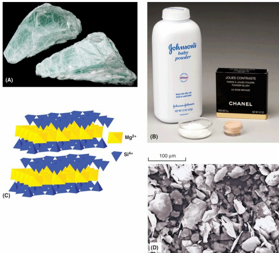
Figure 2.3 (A) Hand specimens of talc, \text{Mg}_3\text{Si}_4\text{O}_{10}(\text{OH})_2 . (B) Commercial containers of baby (talcum) powder and cosmetic facial powder. Two dishes, with talc and facial powder, respectively. (C) A perspective view of the layered internal atomic structure of talc. The \text{Mg}^{2+} ions are sandwiched between two opposing sheets of (\text{SiO}_4)^{4-} tetrahedra. (D) Talcum powder from the Petri dish in (B) photographed by scanning electron microscope. This shows the somewhat variable grain size of the tiny (very soft) flakes at about 400\times magnification.
