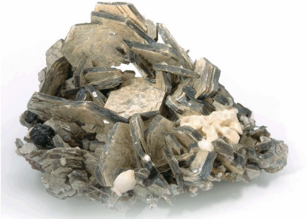
Figure 7.30 Randomly intergrown cluster of well-formed tabular crystals of muscovite with pseudo-hexagonal outlines. These are referred to as pseudo-hexagonal because the underlying structure of muscovite is monoclinic.
