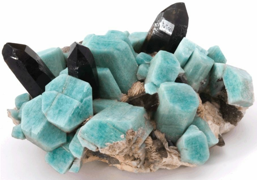
Figure 2.6 A hand specimen of beautifully crystallized green microcline feldspar (known as amazonite) and smoky quartz crystals. The crystals in
