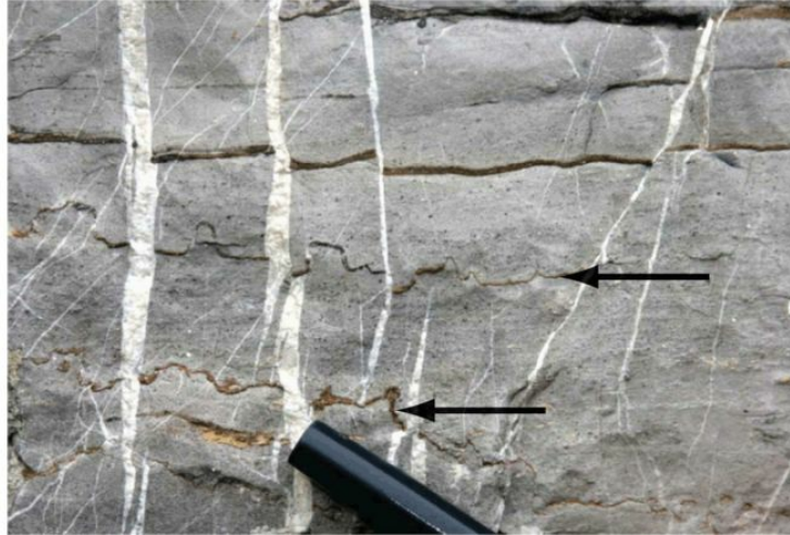
Figure 12.33 Horizontally bedded limestone in which vertical pressure solution generated irregular stylolites (arrows) parallel to bedding, and horizontal extension created white calcite veins along normal faults that are roughly perpendicular to bedding.
