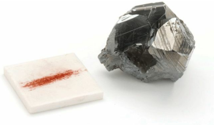
Figure 3.12 A black, metallic crystal of hematite, \text{Fe}_2\text{O}_3 . The streak of all hematite is red as shown on an unglazed porcelain plate.
