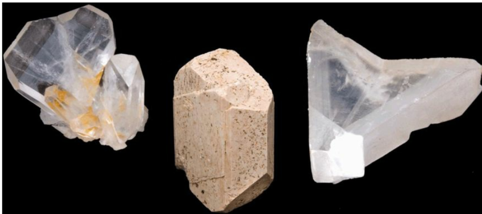
Figure 5.23 Photos of three twin types. From left to right: a Japan twin in quartz (a contact twin); a Carlsbad twin in orthoclase (a penetration twin); and a butterfly twin in calcite (a contact twin).
