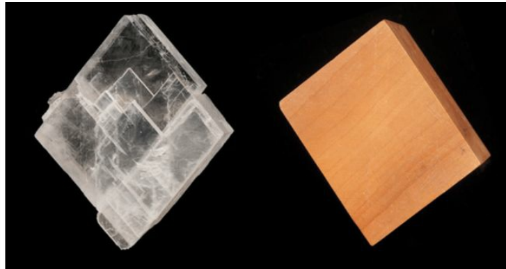
Figure 3.16 Excellent rhombohedral cleavage (three cleavage directions, but not at 90^\circ to one another) as shown by calcite, \text{CaCO}_3 . This optically clear, colorless variety of calcite is known as Iceland spar. A small wooden rhombohedral model shows the planar orientations that deviate from those seen in a cube.
