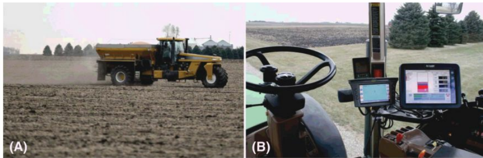
Figure 18.3 (A) A modern farm vehicle carrying three separate sources of nitrogen, phosphorus, and potassium fertilizer that are blended and applied at a specified rate determined by the vehicle's position as determined by a global position system (GPS). (B) Interior of the cab of a modern farm vehicle showing the GPS unit, which actually governs the navigation of the vehicle on the left and the computer controlling the mixing and application of fertilizer and seeds on the right.
