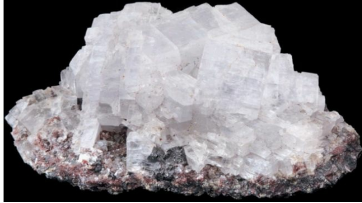
Figure 11.29 A cluster of equant anhydrite crystals each with three sets of different pinacoidal faces.
