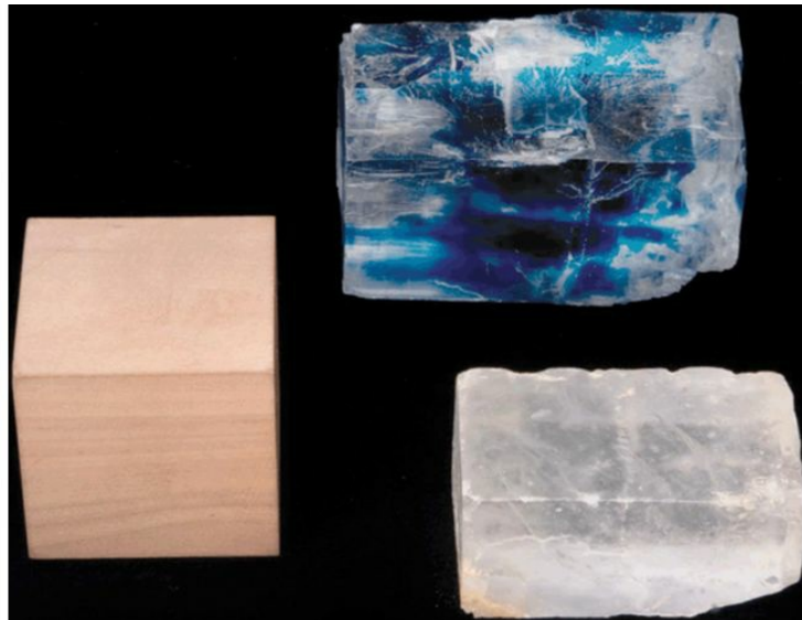
Figure 3.15 Excellent cubic cleavage (three cleavage directions at 90^\circ to one another) in halite, NaCl. Blue and white translucent cleavage fragments and a small wooden model of a cube.
