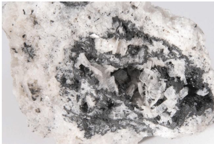
Figure 7.10 Close-up of a small vug in rhyolite with colorless to white, transparent sanidine crystals intermixed with black hornblende.
