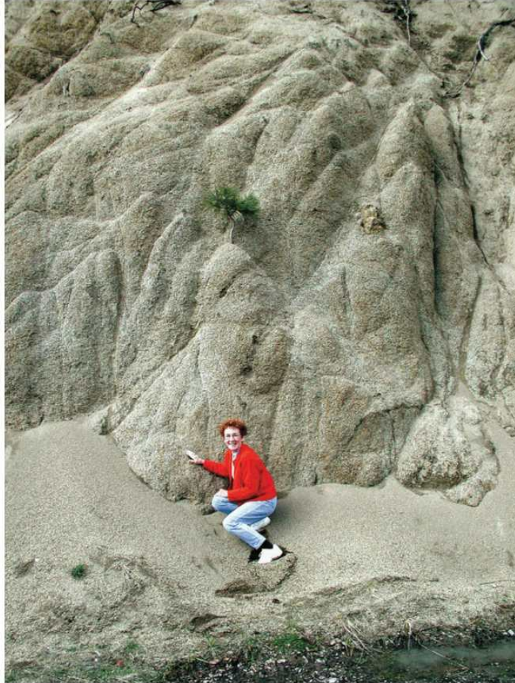
Figure 12.4 Road cut through deeply weathered granite near Sumpter, Oregon. Although original joints are still visible, weathering is so advanced that the mineral grains lack cohesion and are forming detritus (granite grus) along the base of the outcrop.
