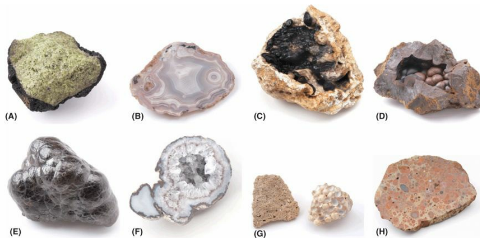
Figure 3.2 Illustrations of many of the states of aggregation listed in Section 3.2 . (A) Granular grains of yellow-green olivine in a volcanic bomb of dunite (a rock type made up essentially of olivine). (B) Finely banded as in this polished slab of agate. (C) Botryoidal, as shown by the outer, almost-black surface of chalcedony. (D) Botryoidal goethite. (E) Reniform hematite. (F) A geode with an outer lining of slightly blue chalcedony and a cavity lined with milky white, translucent quartz crystals. (G) Oolitic and pisolitic limestones. (H) Pisolitic bauxite.
