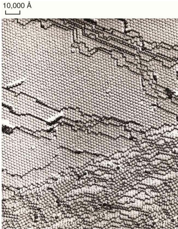
Figure 3.9 A scanning electron microscope image of opal with a chalky appearance. The amorphous spheres of \text{SiO}_2 \cdot n\text{H}_2\text{O} composition are \sim 2500 \text{ \AA} in diameter.
