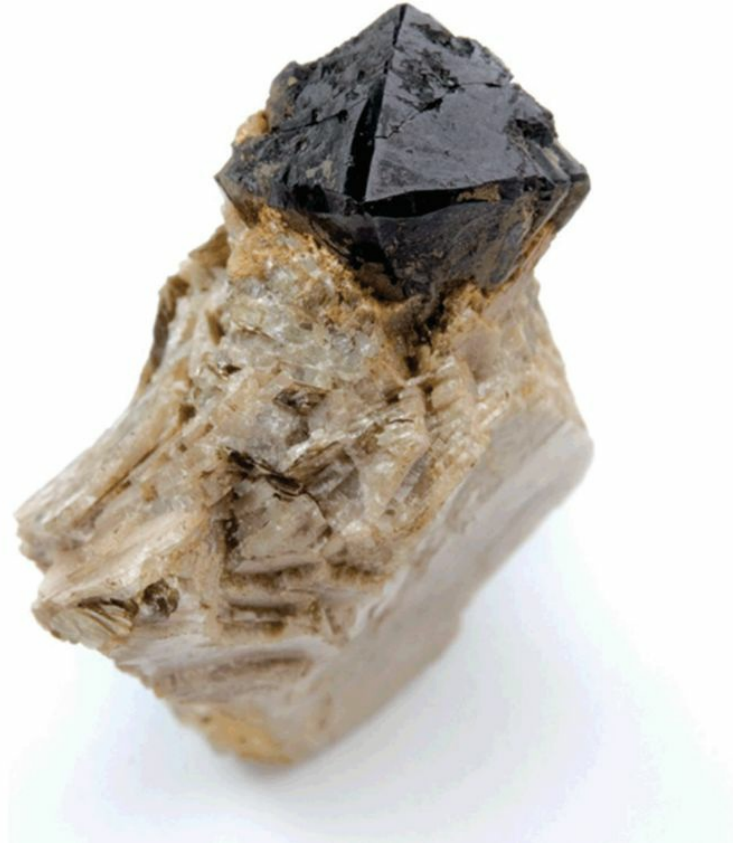
Figure 7.55 Octahedral crystal of uraninite on quartz. The four small modifying faces at the front tip of the octahedron are those belonging to a dodecahedron.
