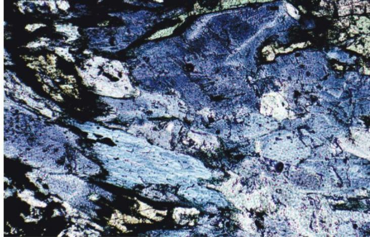
Figure 14.15 Glaucophane in a thin section as seen in plane polarized light. It is highly pleochroic and shows the typical lavender-blue color in one crystallographic direction. Width of field of view is 3 mm.
