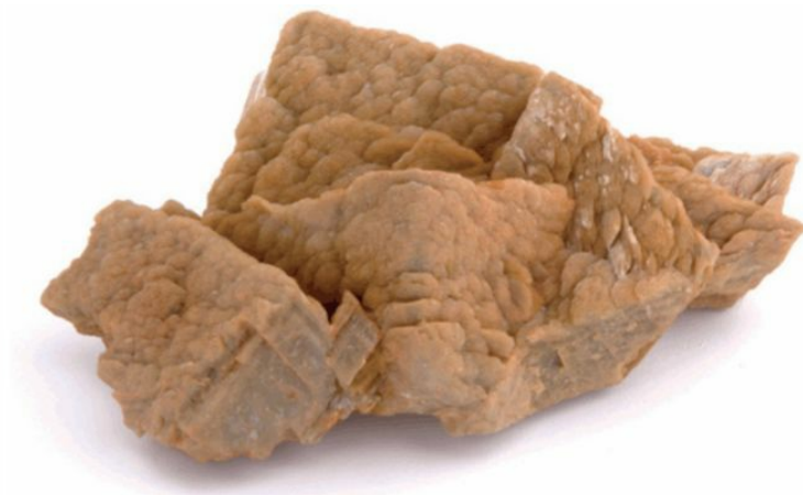
Figure 11.20 A group of yellowish-brown rhombohedral crystals of siderite with composite and somewhat curved faces.
