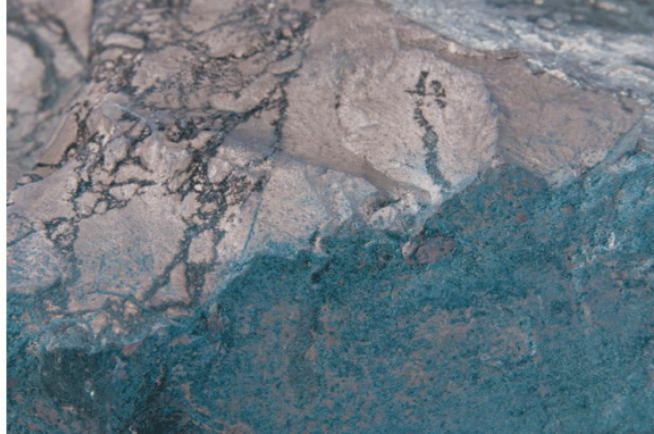
Figure 16.14 Massive bornite with a fresh surface of brownish-bronze color. The tarnished portion shows variegated purples and blues, also known as peacock ore.
