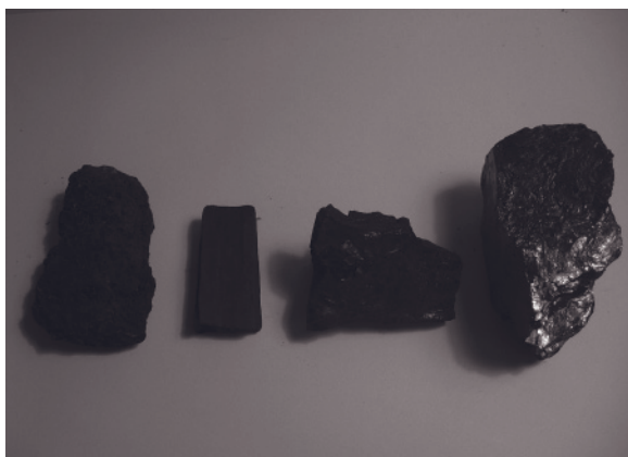
Figure 14.30 Peat and the major ranks of coal derived from it during coalification (left to right): peat, lignite, bituminous and anthracite. Note the increases in compactness, hardness and luster and change in color from brown to black (carbon rich) with increasing rank. (Photo by John O'Brien.) (For color version, see Plate 14.30, between pp. 408 and 409.)
