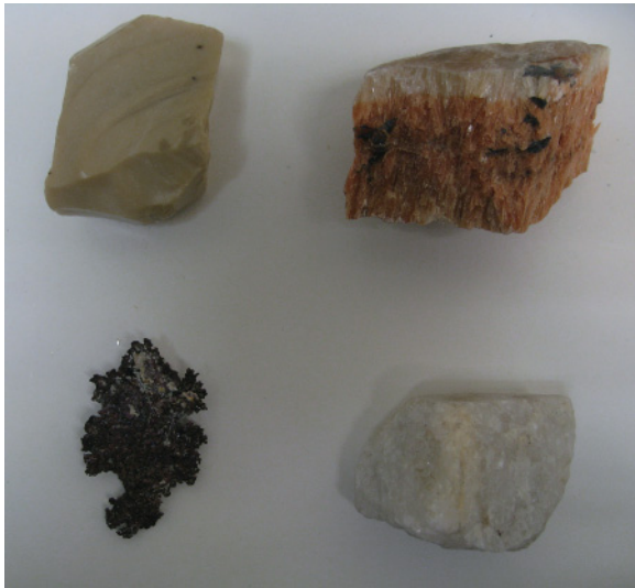
Plate 5.7 Fracture types, clockwise from upper left: conchoidal fracture in opal; splintery fracture in selenite gypsum; uneven or irregular fracture in alabaster gypsum; hackly fracture in native copper. (Photo by John O'Brien.)
