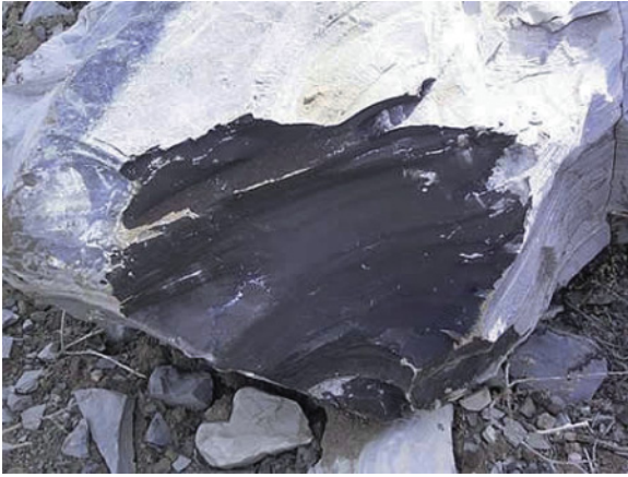
Plate 13.19 Oil shale with a dark color due to its oil content. (Photo courtesy of US Department of Energy, Argonne National Laboratory.)
