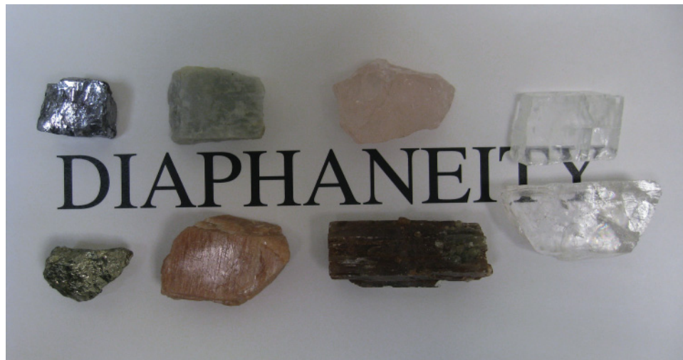
Plate 5.8 Diaphaneity, from left: first pair, opaque, metallic galena and pyrite, which do not transmit light; second pair, plagioclase and potassium feldspar, which are somewhat translucent; third pair, rose quartz and aragonite, which are moderately translucent; fourth pair, calcite and fluorite, which are transparent and transmit the underlying image. (Photo by John O'Brien.)
