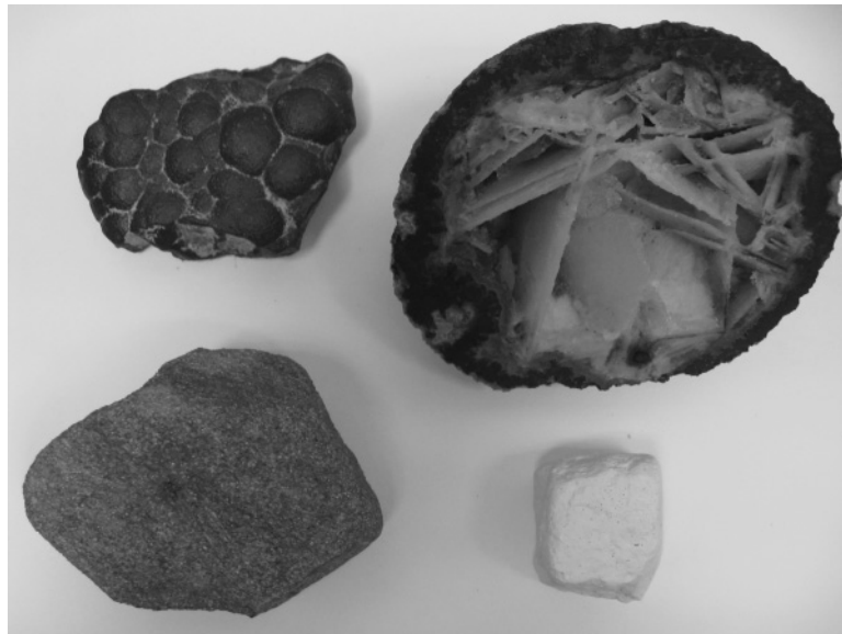
Figure 5.3 Crystal aggregate habits, clockwise from upper left: colloform (botryoidal) cassiterite; reticulate gypsum in geode; massive kaolinite; granular olivine. (Photo by John O'Brien.) (For color version, see Plate 5.3, between pp. 248 and 249.)
