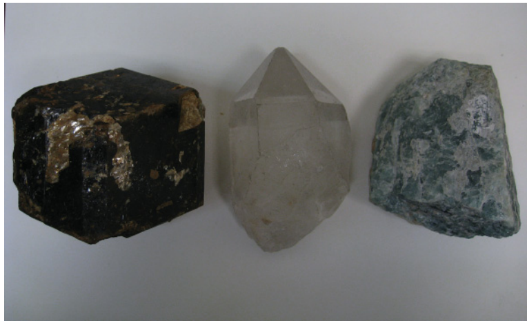
Plate 5.5 From left: euhedral tourmaline, completely enclosed by crystal faces; subhedral quartz, partially enclosed by crystal faces; anhedral apatite, lacking crystal faces. (Photo by John O'Brien.)
