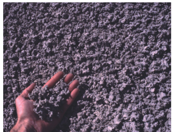
Plate 13.18 Bentonite, with its typical, lumpy popcorn-like appearance, Mowry Formation, Cretaceous, Wyoming. (Photo courtesy of Wayne Sutherland, with permission of Wyoming State Geological Survey.)
