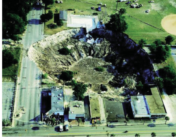
Plate B12.1b (i) Cave spring with an underground river emerging from a cave produced by subsurface dissolution, Virginia. (ii) Sinkhole, Winter Park, Florida produced by the sudden collapse of the surface into a subsurface cavity, May, 1981. (Courtesy of the USGS.)
