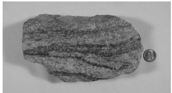
Figure 17.15 Gneissic color banding with light-colored quartz and feldspar layers and dark pyroxene layers. Note the fold hinge within the mafic layer in the left side of image, which suggests transposition processes. (Photo by Kevin Hefferan.)
