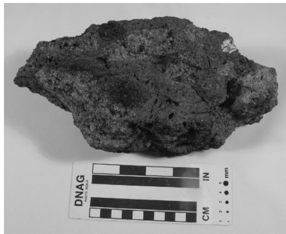
Figure 8.10 Olivine xenocrysts in vesicular basalt. (For color version, see Plate 8.10, between pp. 248 and 249.)
