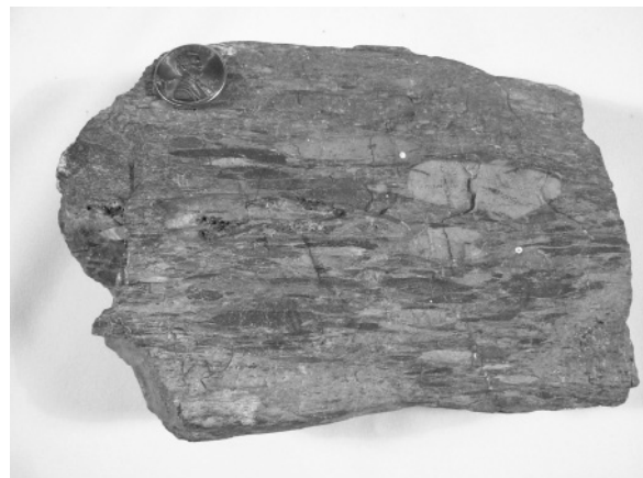
Figure 17.10 Stretched pebble conglomerate in which the clasts have been flattened parallel to the direction of the least compressive stress. (Photo by Kevin Hefferan.)
