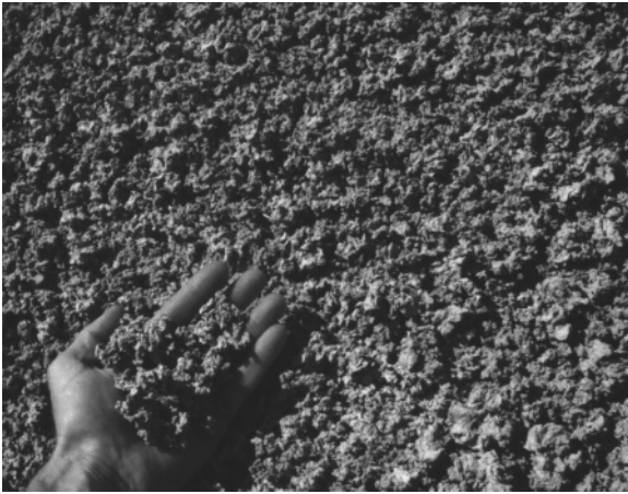
Figure 13.18 Bentonite, with its typical, lumpy popcorn-like appearance, Mowry Formation, Cretaceous, Wyoming. (Photo courtesy of Wayne Sutherland, with permission of Wyoming State Geological Survey.) (For color version, see Plate 13.18, between pp. 408 and 409.)
