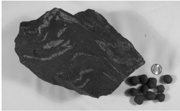
Figure 17.17 Lake Superior taconite rock sample displaying transposed folds. To the right, note the processed taconite pebbles produced in the mining process. (Photo by Kevin Hefferan.)
