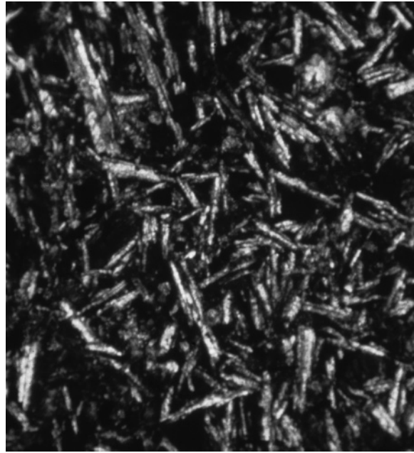
Figure 7.5 Aphanitic basalt with microcrystalline texture as viewed under a petrographic microscope. Note the euhedral to subhedral acicular plagioclase crystals embedded within a cryptocrystalline groundmass. Field of view is 2 cm. (Photo by Kevin Hefferan.) (For color version, see Plate 7.5, between pp. 248 and 249.)
