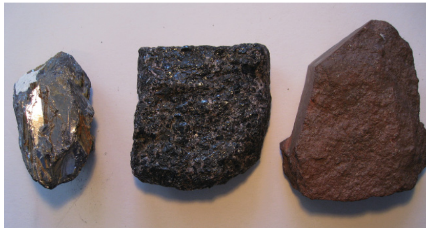
Plate 5.10 Mineral lusters, from left: metallic stibnite; submetallic chromite; dull hematite. (Photo by John O'Brien.)
