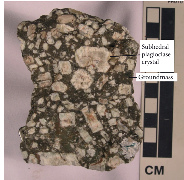
Plate 7.7 Andesite porphyry displaying aphanitic porphyritic texture. Note the subhedral plagioclase phenocrysts (white crystals) and the fine-grained aphanitic groundmass (gray). (Photo by Kevin Hefferan.)
