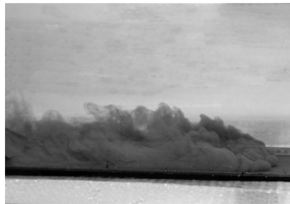
Figure 11.39 Turbidity current in a laboratory showing the head and main body, and the turbulent suspensions that developed over both. (For color version, see Plate 11.39, between pp. 248 and 249.)
