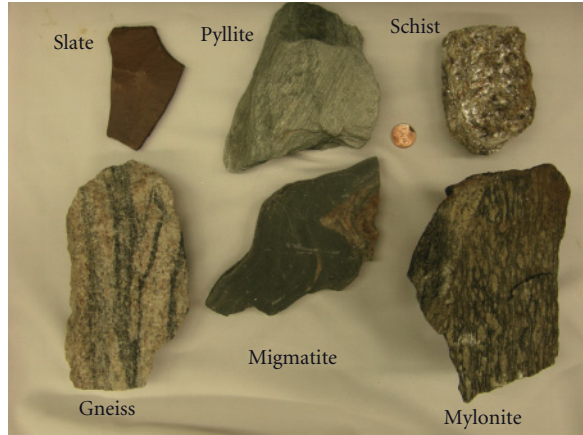
Plate 15.3 Common metamorphic rocks: (a) non-foliated rocks, (b) foliated rocks. (Photos by Kevin Hefferan.)
