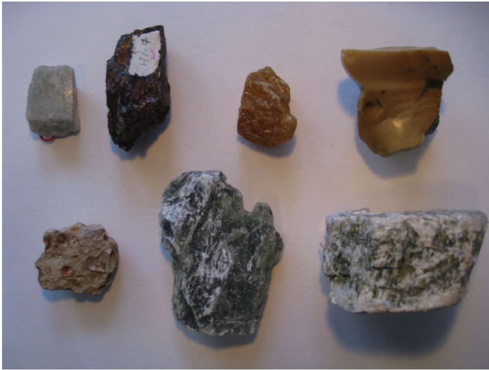
Plate 5.11 Non-metallic mineral lusters, clockwise from upper left: vitreous plagioclase; subvitreous garnet; resinous amber; waxy opal; silky serpentine; pearly soapstone; dull, earthy bauxite. (Photo by John O'Brien.)
