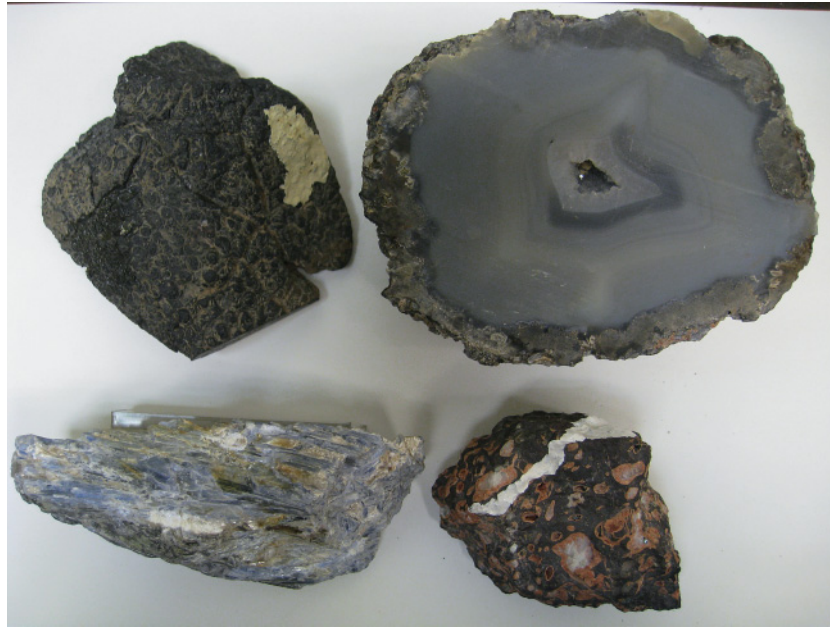
Plate 5.4 Crystal aggregate habits, clockwise from upper left: pisolitic calcite; concentrically banded chalcedony in geode; amygdaloidal calcite and thomsonite filling vesicles in basalt; lamellar to foliated kyanite. (Photo by John O'Brien.)
