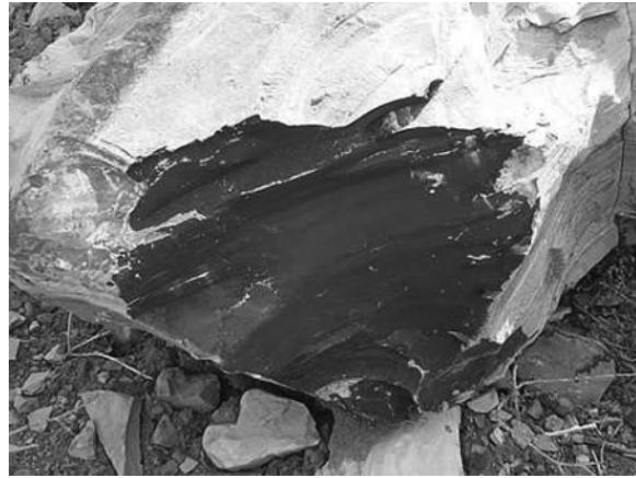
Figure 13.19 Oil shale with a dark color due to its oil content. (Photo courtesy of US Department of Energy, Argonne National Laboratory.) (For color version, see Plate 13.19, between pp. 408 and 409.)
