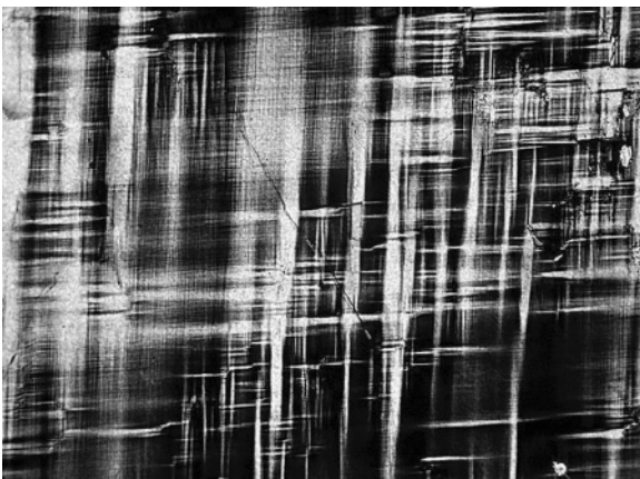
Figure 6.14 Crossed polars photomicrograph of a microcline crystal, displaying the gridiron twinning and low birefringence (first order gray and white colors) that make this mineral easy to recognize under crossed polars. (Photo courtesy of Kurt Hollacher, Union College.) (For color version, see Plate 6.14, between pp. 248 and 249.)
