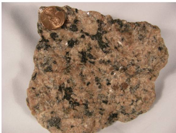
Plate 7.4 Coarse-grained phaneritic granite with early formed, euhedral potassium feldspar. Subhedral quartz and hornblende represent later, void-filling minerals. (Photo by Kevin Hefferan.)
