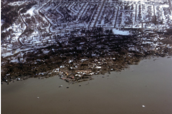
Plate 12.23 (a) Collapsed apartment buildings in Nigata, Japan, after the 1964 earthquake. (b) Neighborhood in Anchorage, Alaska, destroyed when the ground slumped, carrying structures more than 1 km, after sand lenses became liquefied during another 1964 earthquake. (From the Karl Steinbrugge Collection, courtesy of the National Information Service for Earthquake Engineering, EERC, University of California, Berkeley.)
