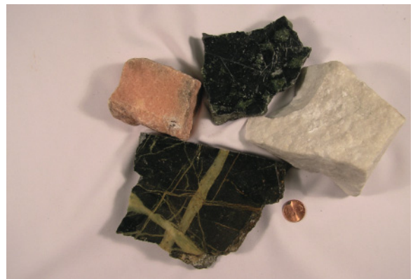
Plate 17.4 Marble occurs in multiple colored varieties depending upon chemical substitutions in calcite and dolomite and the presence of accessory minerals. (Photo by Kevin Hefferan.)
