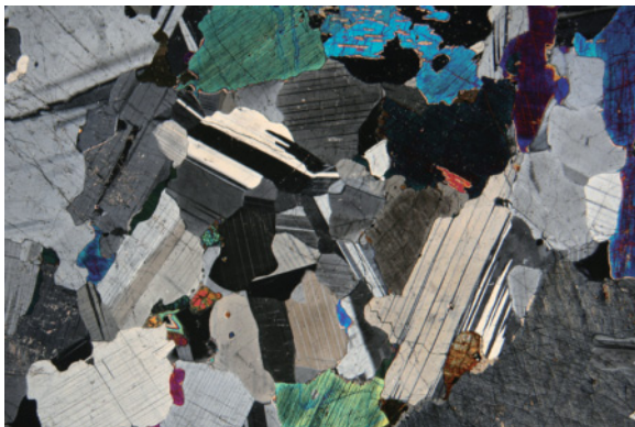
Plate 6.11 Photomicrograph of a thin section of gabbro viewed in crossed polars mode. The plagioclase is striped and has low birefringence (low first order white and gray interference colors). Brightly colored augite has moderate-high birefringence (well-developed second order interference colors in shades of blue, purple, red and orange). (Photo courtesy of Siim Sepp.)
