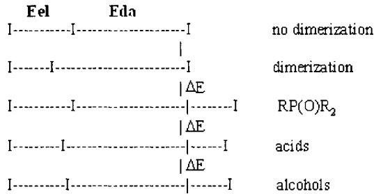
Figure 3: Simplified scheme of changes in interaction energy regarding a mineral with the collector compositions and RSA.
