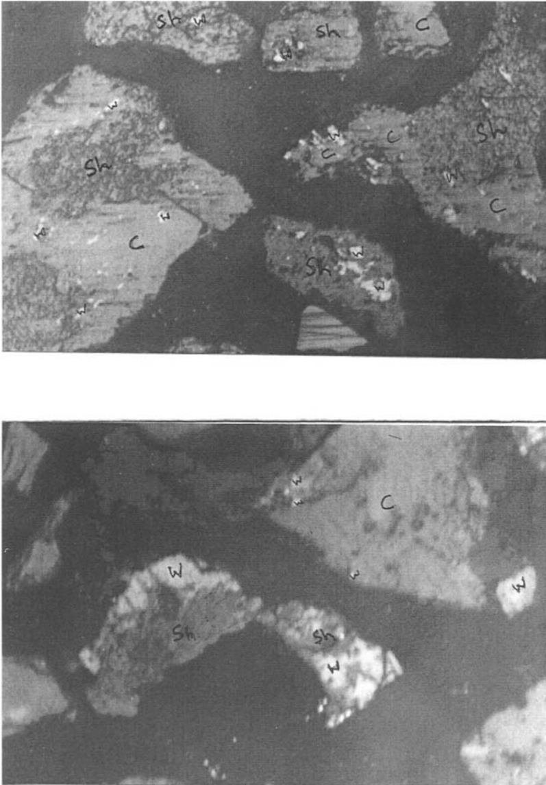
Figure 1: Photomicrographs: top: wolframite (W) as fine inclusions within cassiterite (C) and scheelite (Sh); bottom: scheelite (Sh) replacing wolframite (W) around grain boundaries and cracks.
