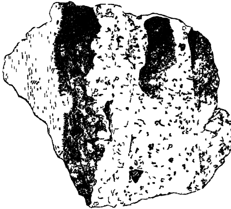
FIG 6—Vein in Griffith Mine, Georgetown Colo, Showing Two Periods of Vein Deposition (After Spurr and Garry)
