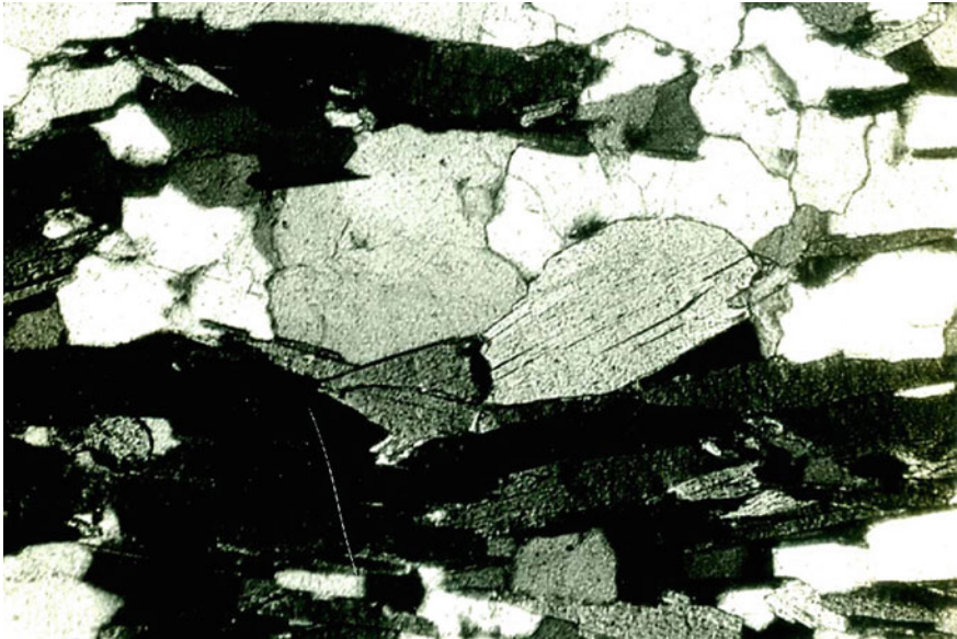
Fig. 1.31 A mica fish ( top-to-right shear) with a notch/mouth at one of the sides. The other side is irregularly ( parallel ) pulled apart. Cross-polarized light. Location Shyok Suture zone (India). Width of view 4 mm
