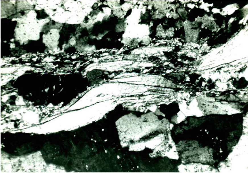
Fig. 2.9 Top-to-right brittle sheared slices of micas of somewhat trapezoid shapes. Notice that mica minerals are more prone to trapezoid shapes than the quartzofeldspathic matrix. Cross-polarized light. Location Zaskar Shear Zone (India). Width of view 4 mm
