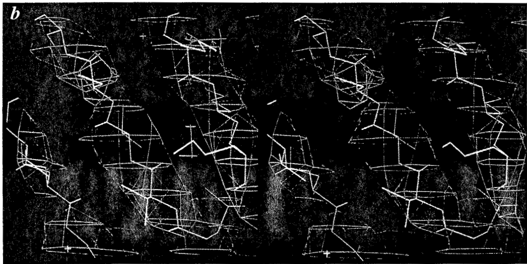
Plate 12 Electron-density maps at increasing resolution. Maps were calculated using final phases, and Fourier series were truncated at the resolution limits indicated: (a) 6.0 Å; (b) 4.5 Å; (c) 3.0 Å; (d) 1.6 Å. (For discussion, see Chapter 7.) ( Continues )
