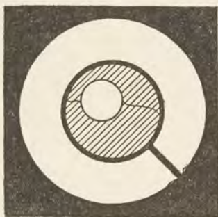
FIG. 20.—A loop of very fine cotton is floated on the soap film, and the part of the film inside the loop is touched with a hot needle. Instantly the loop flies into a perfect circle. (By courtesy of Prof. C. V. Boys.)
