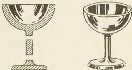
FIG. 48.—Ice molds and the making of a cup (from Tyndall).
