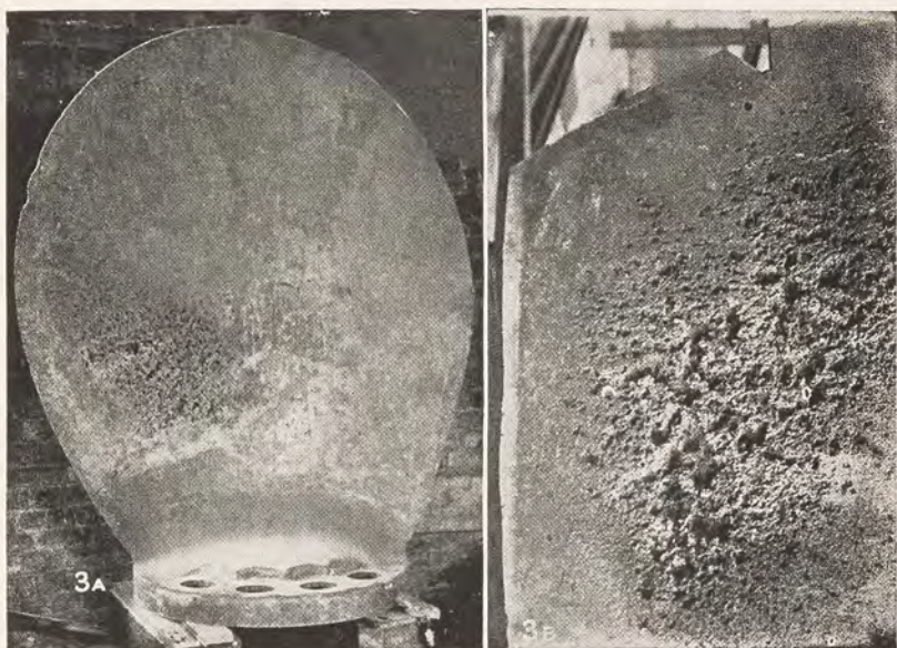
The right-hand figure shows erosion in a portion of an early propeller blade of the "Mauretania." Notice the small bite in the edge of the blade shown in full in the left-hand figure.
