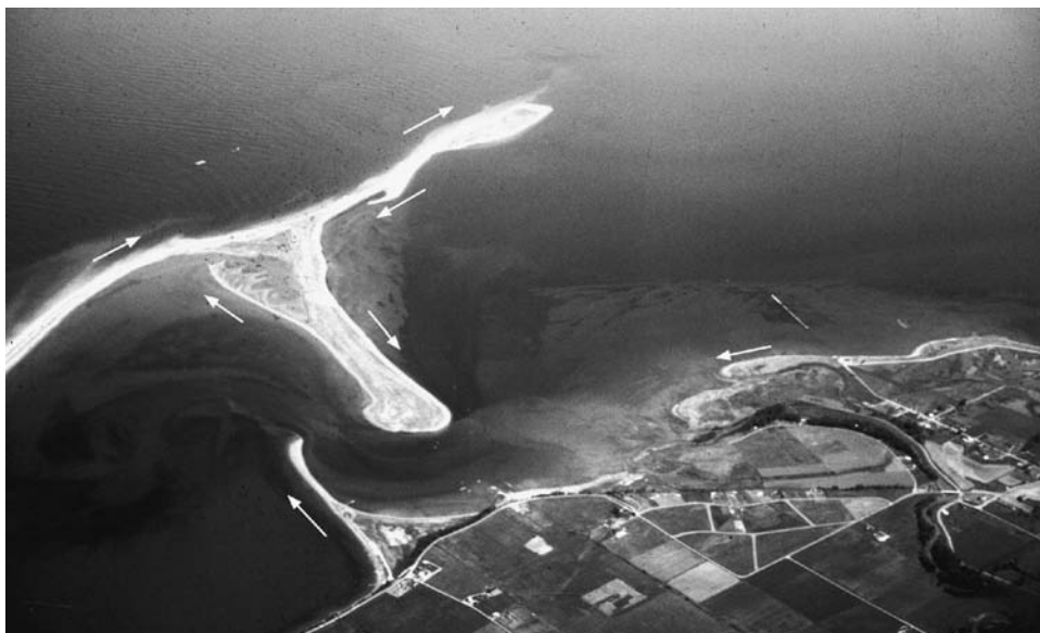
Figure 8.4 Dungeness Spit, on the coast of Washington State, USA, with arrows indicating the directions of longshore drifting, determined by local exposure to wind-generated waves
