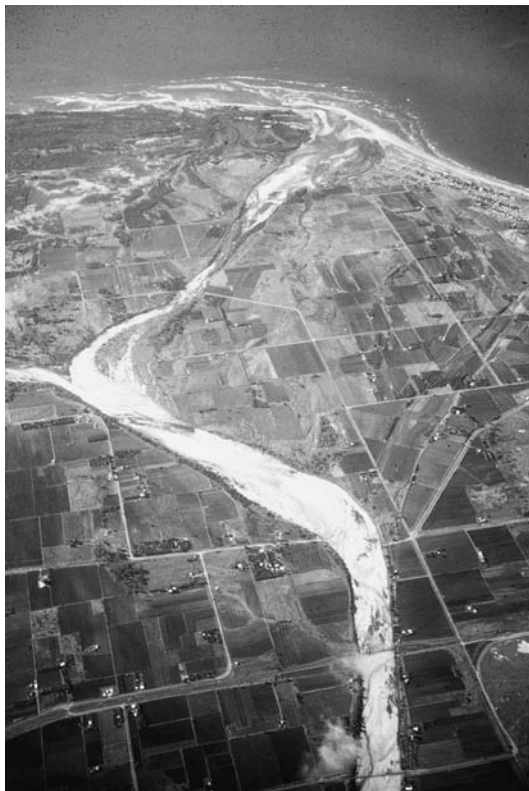
Figure 6.3 Fluvial sediment supply to beaches, illustrated by the River Don, in NE Australia. Sandy material in the channel is washed down to the river mouth during periods of strong fluvial discharge, and is then reworked and distributed along the coast by wave action
