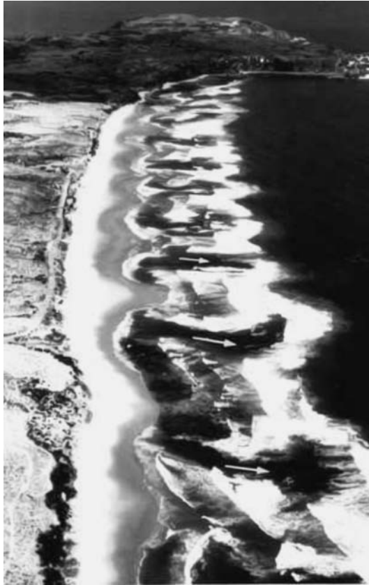
Figure 2.5 Rip currents (arrowed) in the surf on Woolamai Beach, Phillip Island, Australia. At the head of each rip current the beach has been lowered and cut back
