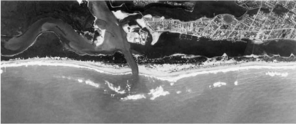
Figure 6.27 The artificial entrance to the Gippsland Lakes, cut through the outer barrier in 1889 and bordered by stone breakwaters. Sand accretion on either side of the breakwaters has formed coastal forelands with successive parallel foredunes, and wave patterns show the location of the looped offshore bar. Crown Copyright Reserved
