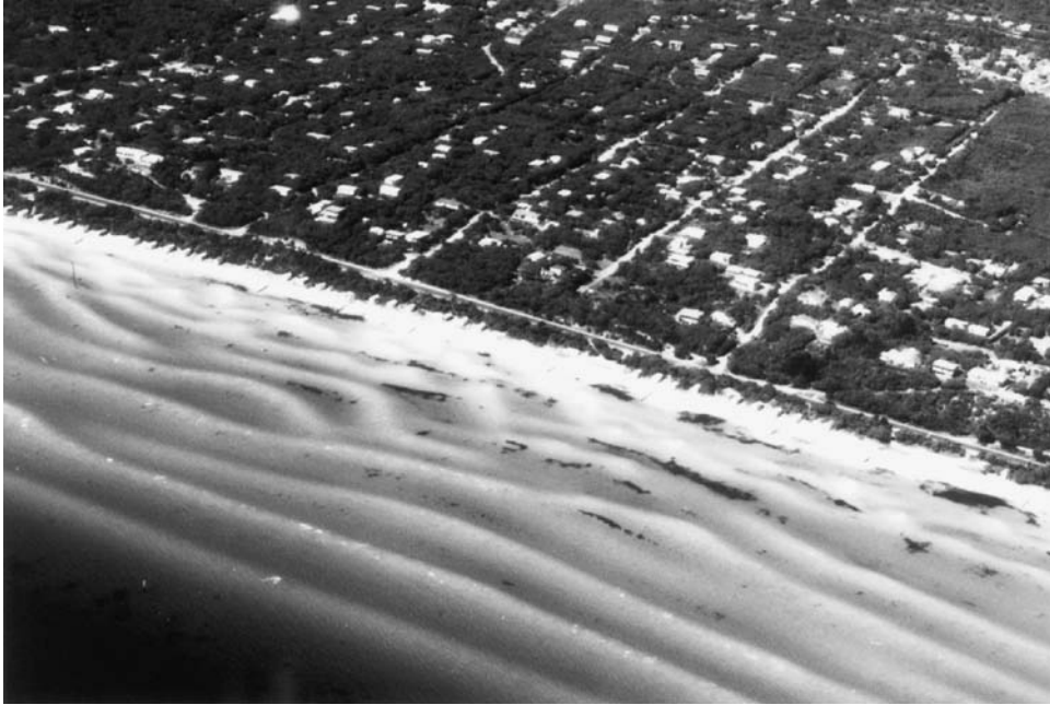
Figure 8.14 Multiple nearshore sand bars at Rosebud, Port Phillip Bay, Australia
