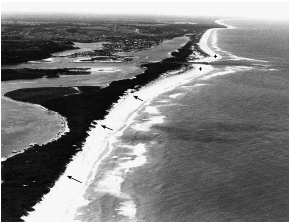
Figure 7.2 Erosion (arrowed) of the Ninety Mile Beach, on the outer barrier of the Gippsland Lakes in SE Australia, with accretion (+) on either side of the Lakes Entrance breakwaters (see Figure 6.27)
