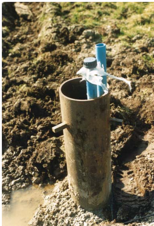
Figure 9.3 Piezometer group measuring water levels in two formations in an opencast working. Source: Photograph by LPT.
