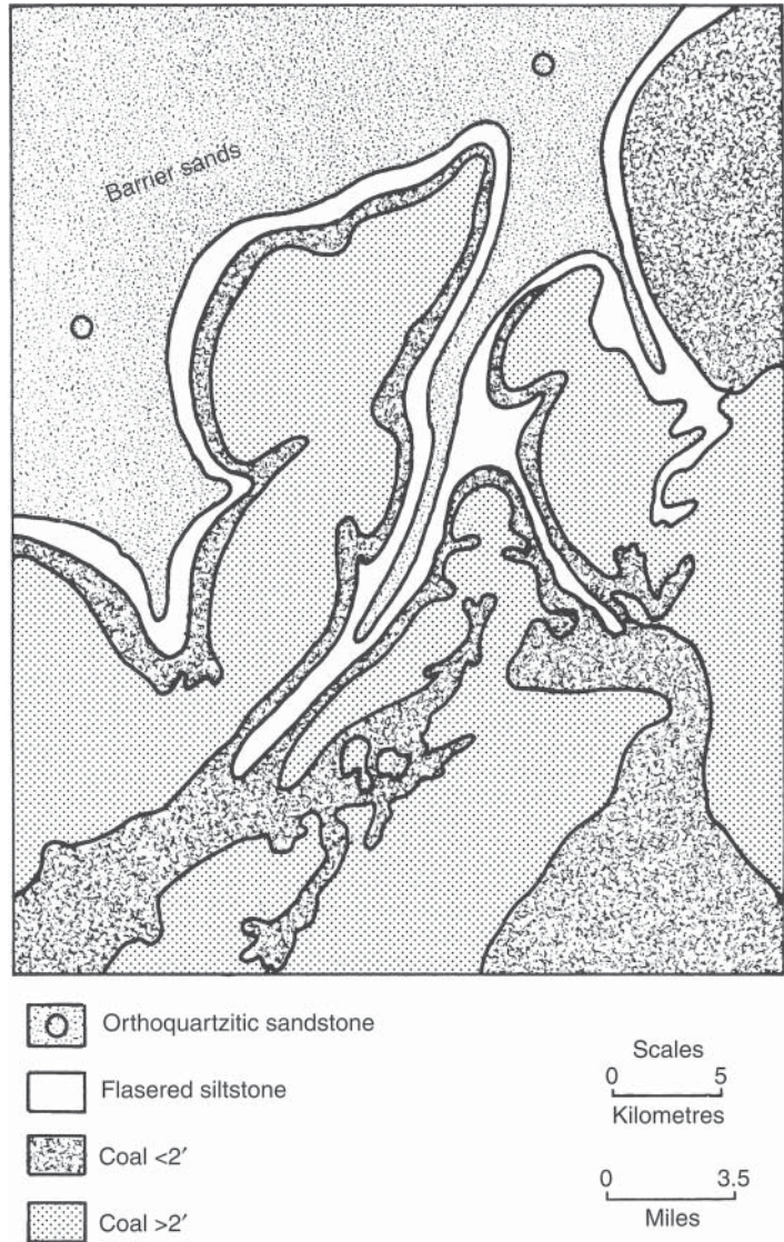
Figure 2.22 Mapped lithotypes compiled from 1000 boreholes over an area of 1000 km 2 , illustrating the regional depositional setting of the Beckley Seam, West Virginia, USA. Source: From Horne et al. (1979).
