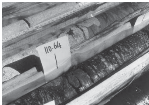
Figure 6.22 Borehole core photographed to show special features. In this instance, the erosive sandstone contact above the coal and the siderite nodules contained in the upper part of the coal seam are seen. Source: Photograph by M.C. Coultas.
