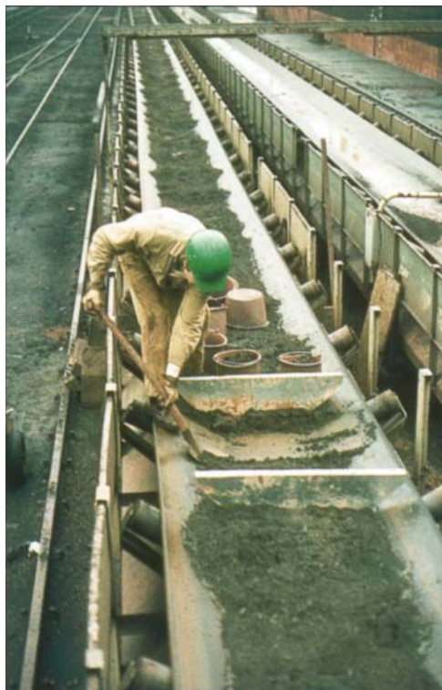
Figure 5.7 The collection of a stop belt sample from a main conveyor (Mazzone 1998).
