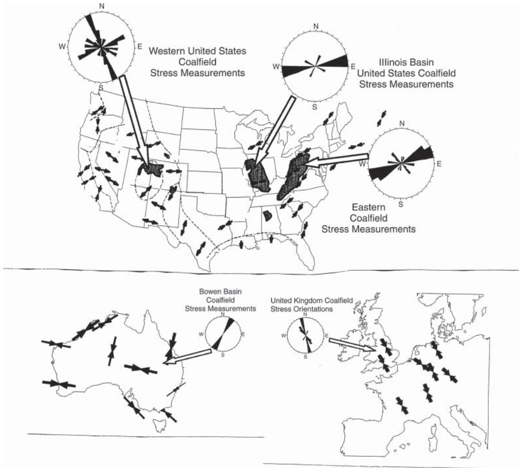
Figure 10.7 World stress maps of USA, Australia, and northern Europe showing principal stress directions together with stress measurements taken in specific coalfield areas (Mark and Gadde 2010).
