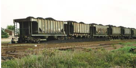
Figure 13.9 Bottom-discharge wagons (60 t), on Eastern Railways, India. Source: Photograph by courtesy of Dargo Associates Ltd.
