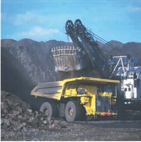
Figure 10.17 Large dump truck (280t) being loaded at Fording coalmine, Canada. Source: Photograph by courtesy of Komatsu Mining Systems.
