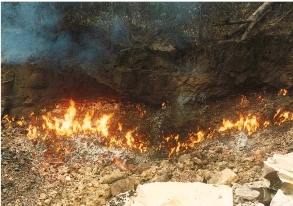
Figure 12.6 (a) Coal burning as a result of ignition by forest fires in Kalimantan, Indonesia. Source: Photograph by LPT. (b) Spontaneous combustion of coal in the highwall of an Indian mine. Source: Photograph by courtesy of Dargo Associates Ltd.
