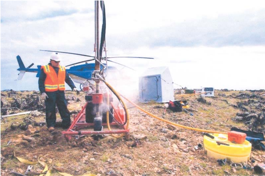
Figure 6.20 Voyager V2200 portable drilling rig.
