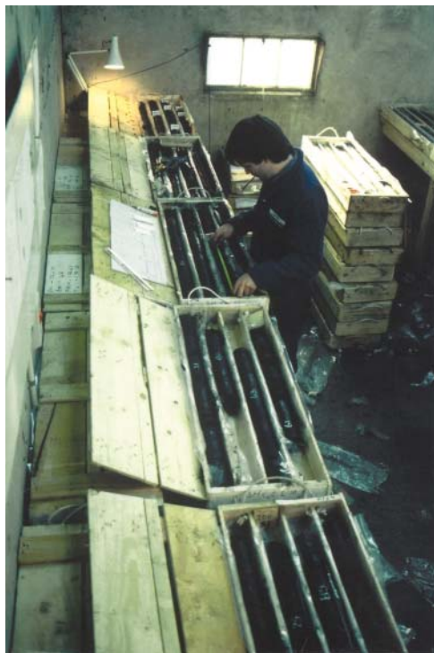
Figure 6.21 Coal geologist logging borehole core in a core shed on-site. Source: Photograph by LPT.
