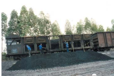
Figure 13.11 Top-discharge wagons with drop-down doors for side unloading, Guizhou Province, PRC. Source: Photograph by courtesy of Dargo Associates Ltd.
