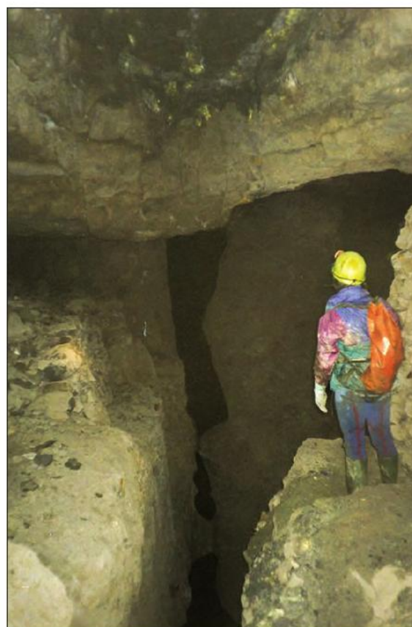
Dangerous stopes following a vein called Tatter’s String in the Brownley Hill mine. Helen Wilkinson photo.
