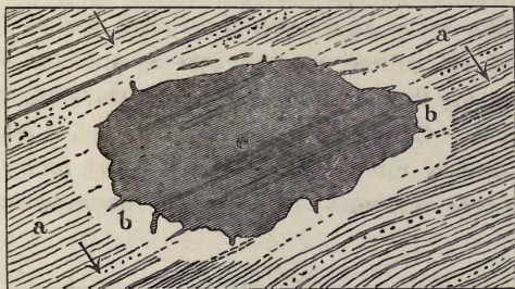
FIG. 106.—Ground-plan of Granite-boss with ring of Contact-Metamorphism; ( a ) sandstones, shales, etc., dipping at high angles in the direction of the arrows; ( b ) zone or ring within which these rocks are metamorphosed; ( c ) granite sending out veins into b .
