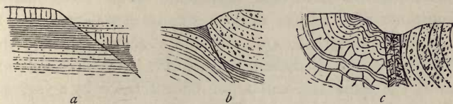
FIG. 100.—Examples of normal Faults.
