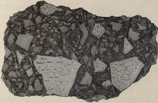
FIG. 73.—Brecciated structure—volcanic breccia, a rock composed of angular fragments of lava, in a paste of finer volcanic debris.
