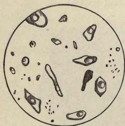
FIG. 68.—Cavities in quartz containing liquids (magnified).
