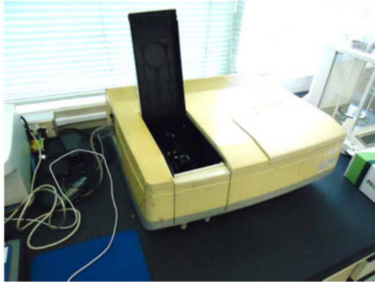
Figure 3. Optical evaluation apparatus is UV-VIS Spectrophotometer.
