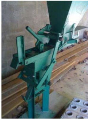
Figure 2. Manual press Vimaq model V2 used to molding bricks.
