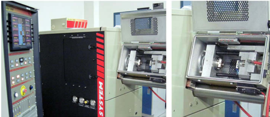
Figure 1: Work area of the Gleeble ® . On the right: vacuum chamber with compression setup.
