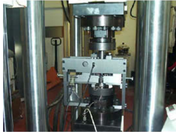
Figure 3. Servo hydraulic uniaxial testing machine used to induce fretting damage in Ti-6Al-4V and 7075-T6 samples
