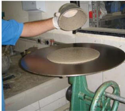
Figure 1. The consistency test - flow table.
