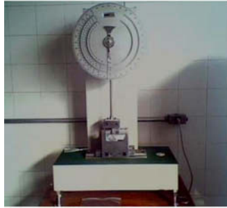
Figure 2: Pantec impact pendulum.
