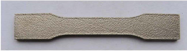
Figure 9. The fabricated IN718 sample by SLM
