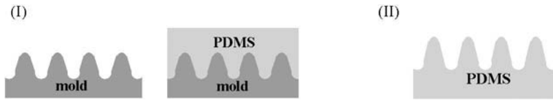
Figure 1. Schematic view of the nanoimprint process, (I) the biomimetic microlens array mold is immersed in PDMS mixture and cured, (II) the mold is removed.
