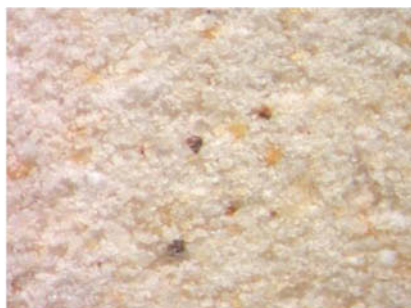
Figure 8 - Image of sample - treated HCl 6h at 90°C. 1cm corresponds to 1.3micron.
