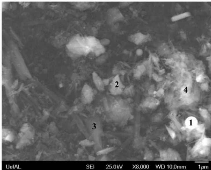
Figure 2. SEM image of different microparticles (1 - 4) in the slag sample
