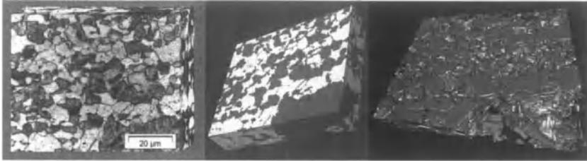
**Figure 4:** Steel 1 - image stack (l.), RVE (m.), reconstructed ferrite grains (r.)
