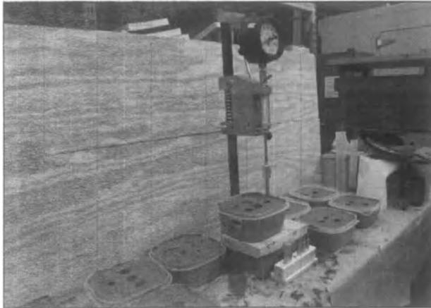
**Figure 2 Measurement of concrete setting time**
