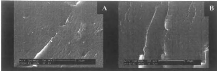
Figure 3. Scanning Electron Microscopy (SEM) surfaces micrographs for EVOH/treated piassava composites. Figure 3(A) EVOH/treated piassava 5 %; Figure 2(B) EVOH/treated piassava 10 %;
