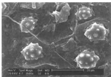
**Figure 5. Micrograph of a piassava fiber**
