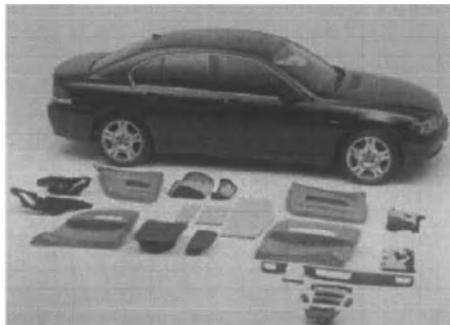
Figure 1. BMW sedan and its different parts made of polymer composites reinforced with lignocellulosic fibers. ([www.bmwgroup.com](http://www.bmwgroup.com))
