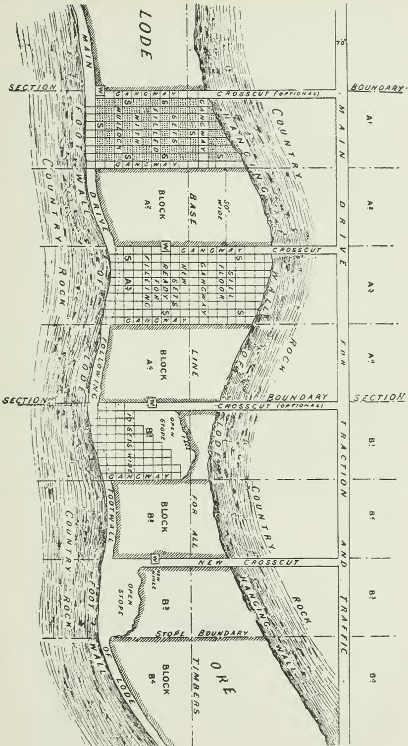
Plan showing the "Block System" of stope and timbering as adopted at the Central Mine.
