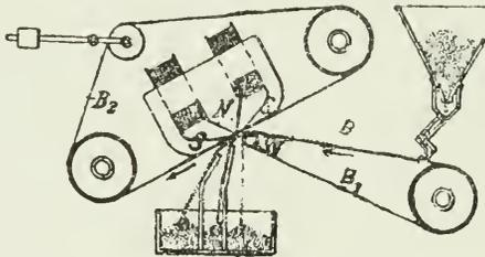
the gangue dropped straight through. The magnetic particles were carried round for a fractional space, and fell on one side of an adjustable shutter, thus being divided from the tailings.
