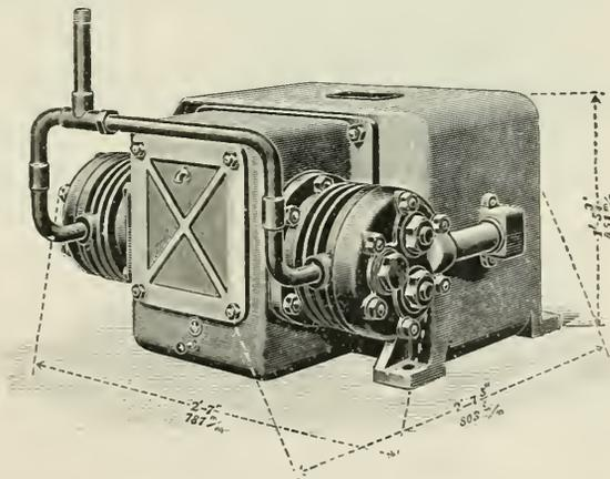
TYPE OF ELECTRIC MOTOR COMPRESSOR.
