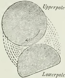
parallel, the upper one cylindrical, and capable of rotation, the lower one semi-cylindrical, and fixed. The dotted lines indicate the magnetic field, which has its greatest intensity where the poles are close, and gradually decreasing as the distance increases. The crushed and dried ore is fed in between these poles by means of an inclined shoot, slightly pressed by a spring against the upper
