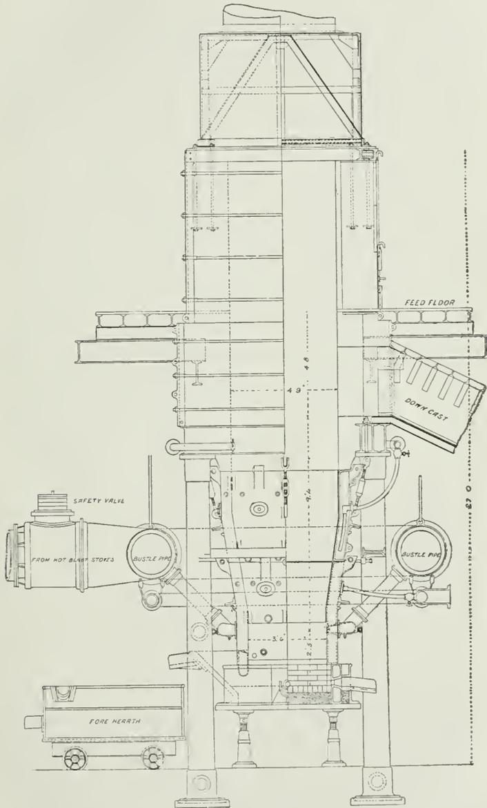
Blast Furnace. Cross Section and End Elevation.
