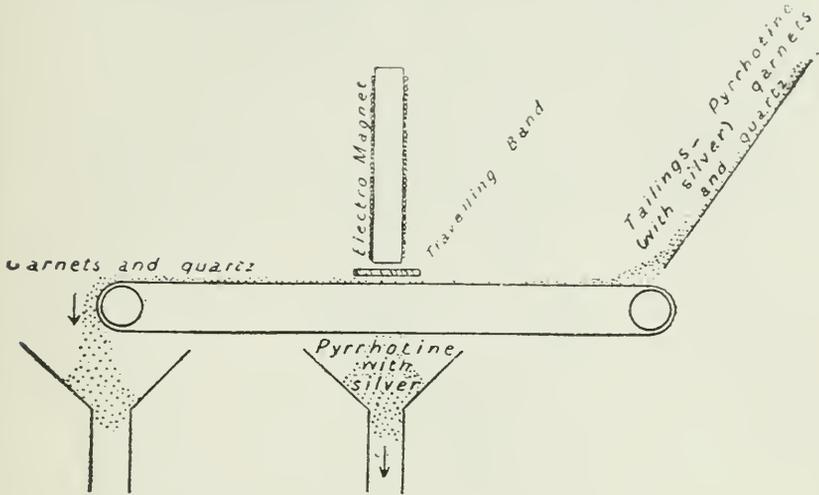
and adhered to the underside of the cross belt until carried over the edge, the garnets and quartz, as gangue, passing over the end.
