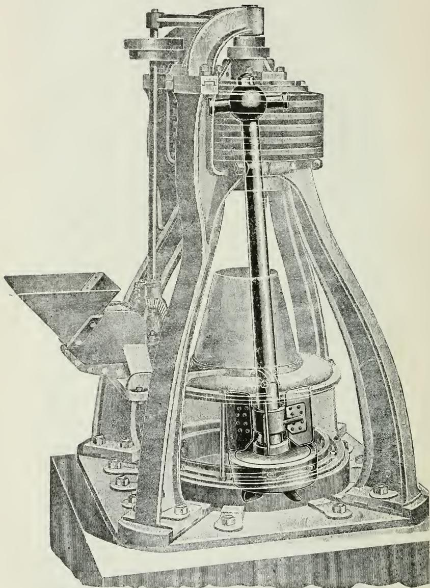
30-inch Griffin Mill arranged for Dry Pulverising.
