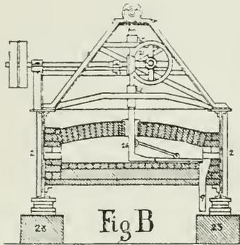
water is circulated in them. A cast-iron shoe may be readily slipped on or off. The iron used in a medium-sized furnace amounts to about 20 tons, a ton being the heaviest part. About 1000 red bricks are used in the construction. The wood used is 5cwt. per ton of ore roasted, when an ordinary reverberatory would take 12cwt. This type of furnace is deservedly popular. Its cost is not as great
