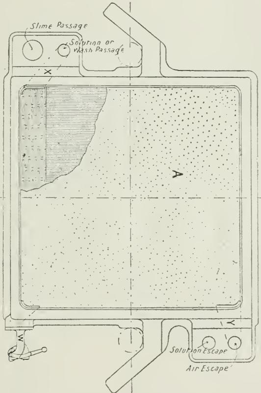
Solution Plate for Filter-Press.
