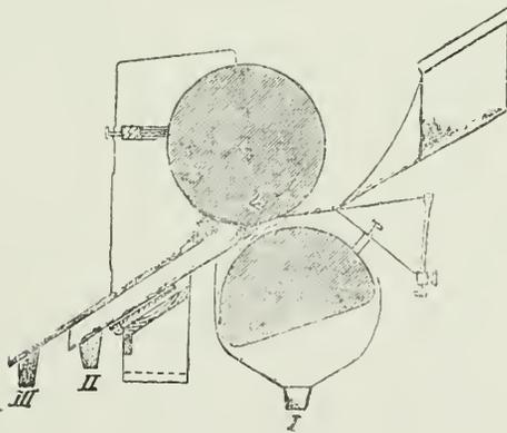
cylinder, as shown in the illustration. The quantity of ore fed in depends on the pitch of the shoot and the velocity of rotation. All para-magnetic minerals cling to the under surface of the upper pole, while the dia-magnetic substances fall over the lower into a receptacle (I) placed below. The faintly para-magnetic minerals soon drop from the cylinder, and are then carried down a lower shoot (II). The more highly para-magnetic particles cling to the
