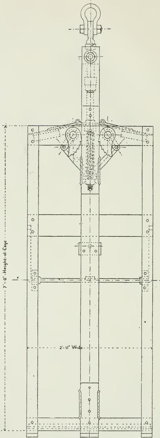
The Bush Patent Mining Cage—Side Elevation.
