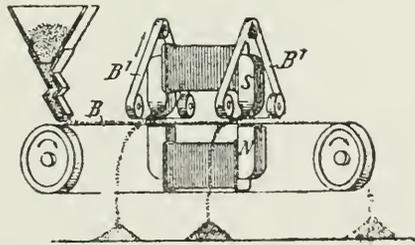
manner with Odling's machine, and dropped into bins at the side. With this system, it is possible to arrange a number of poles one after the other, each being more powerfully excited than the other. By this means, minerals of different permeability may be removed one after the other. This machine is used for separating titanic
