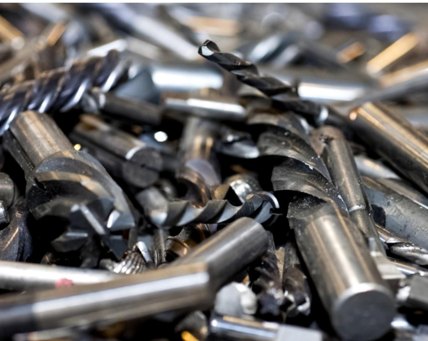
Tungsten-carbide is used in drill bits to increase their hardness and durability. Australia has the world's second largest resources of tungsten.
