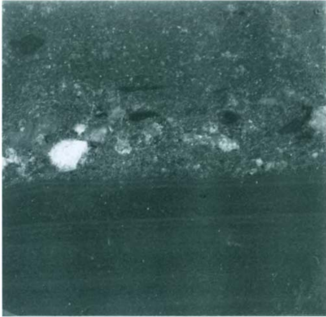
Fig. 5.12. Graded bed of greywacke with basal quartz and shale clasts abruptly overlying interlaminated siltstone and claystone. Torridon Group (Pre-Cambrian), Raasay, Scotland. Specimen 6 cm high.
