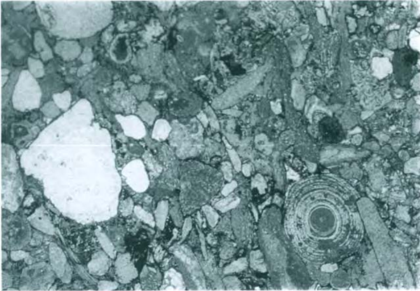
Fig. 6.70. Thin section of basinal turbidite sandstone showing transported skeletal grains and oolites. Conway Castle Grits (Lower Paleozoic), North Wales (20 \times ).
