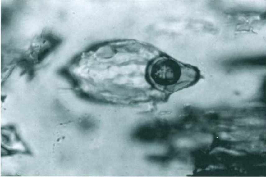
Fig. 7.12. Photomicrograph of an authigenic quartz crystal with a fluid inclusion that contains a globule of oil. (Courtesy of A. Rankin.) It is possible to analyse the inclusion to discover the temperature and chemistry of the fluids in which the crystal grew.
