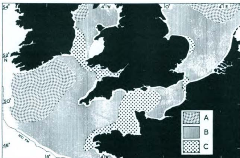
Fig. 6.49. Maps showing the alignment of tidal currents (upper) and of sediment (lower) for part of the north-west European continental shelf. A = mud, B = sand sheet and ridges, C = gravel and scoured sea floor. (From Stride, 1963, by courtesy of the Geological Society of London.)
