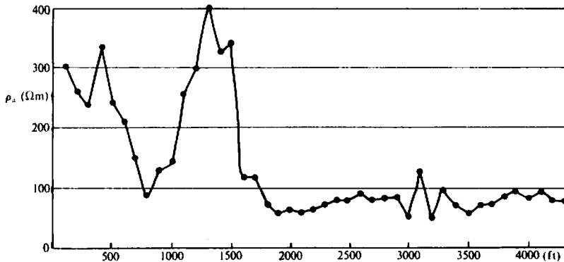
Figure 8.45. Resistivity mapping with Wenner spread over limestone and sandstone section separated by vertical contacts. Station interval 100 ft, a = 100 ft. (After Van Nostrand and Cook, 1966.)
