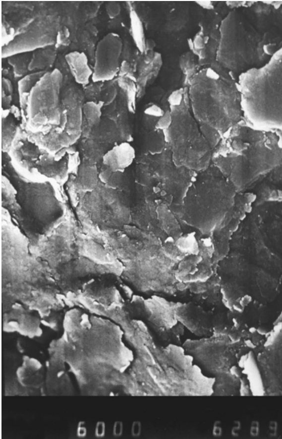
Fig. 11. Scanning electron micrograph of Fithian, Illinois illite.
