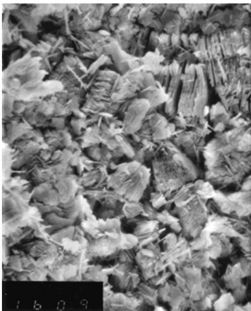
Fig. 32. Scanning electron micrograph of Belitung kaolin.
