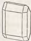
Fig. 129. A ten-sided prism, with two broad faces, terminated by two principal planes, corresponding with the lateral planes.
