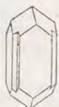
Fig. 112. A double, or twin crystal, consisting of two four-sided prisms joined together, and intersecting each other so as to make their axes coincide.
