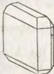
Fig. 105. A four-sided prism, also truncated, and terminated by four planes standing obliquely on the lateral planes.
