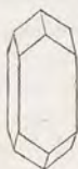
Fig. 111. A compressed four-sided prism, terminated by a pyramid, consisting of four rhombic faces.
