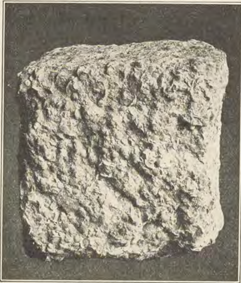
Fig. 110. A block of limestone from Egypt made up entirely of shells of the protozoön Nummulites
