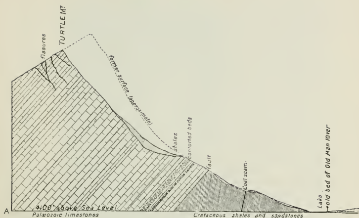
FIG. 49.— Profile of Turtle Mt., showing the amount of material removed in the Frank rock-slide. (Brock)
