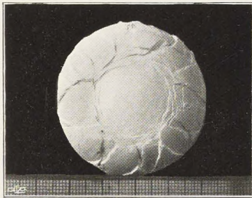
Fig. 2. Sphere of Carrara Marble after deformation by Kick's Process using alum as an embedding material.
