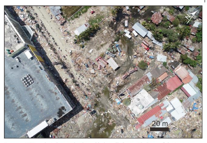
Figure 18.10 A UAV image showing houses, roads, and automobiles damaged by the tsunami. See Figure 18.9 for location.
