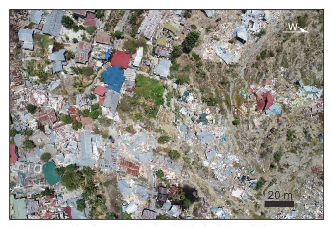
Figure 18.7 UAV image in Palu city showing sand liquefaction damaged lots of buildings. See Figure 18.6b for location.
