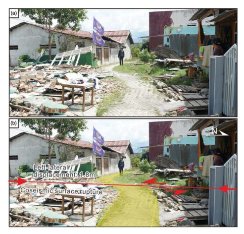
Figure 18.5 Left-lateral offset road. (a) Uninterpreted field photograph taken in Palu City. See Figure 18.2b for location. (b) Interpretation of field photography shown in (a). The red line depicts the location of the fault. The road was left-laterally displaced by 1.8 m.
