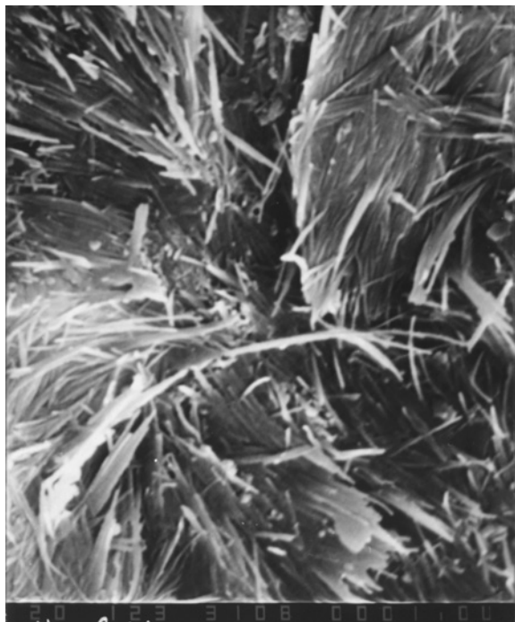
Fig. 15. Scanning electron micrograph of palygorskite.
