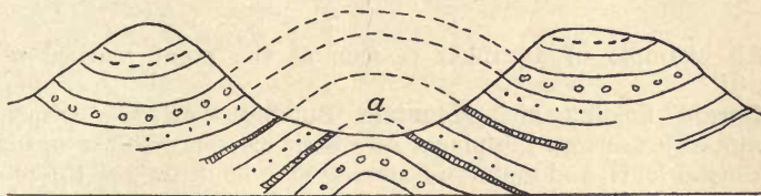
FIG. 81.—Showing valley excavated along course of an anticline, and ridges composed of beds arranged in synclinal folds.
