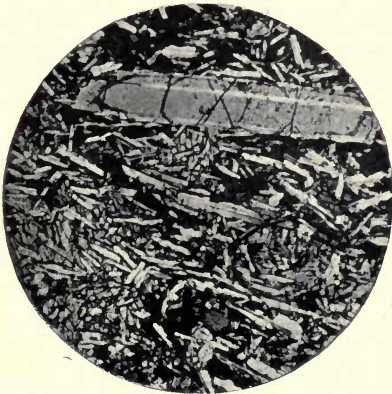
FIG. 146.—Microphotograph of olivine-basalt from North Auckland, N.Z., showing phenocryst of plagioclase and ophitic structure of ground-mass ; there is a general orientation of feldspars.
