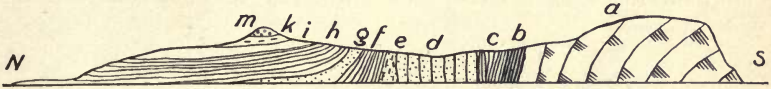
FIG. 73.—Showing monoclinal folding of Lower Tertiary strata in section of the Isle of Wight, Totland Bay to Headon Hill. (After H. W. Bristow.)
