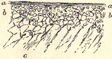
FIG. 2.—Showing graduation from (c) rock to (b) subsoil, and thence into (a) vegetable soil.
