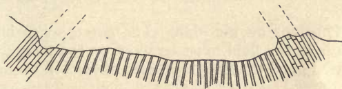
FIG. 256.—Showing variations of dip of highly-inclined strata in the centre of a steep anticline.
