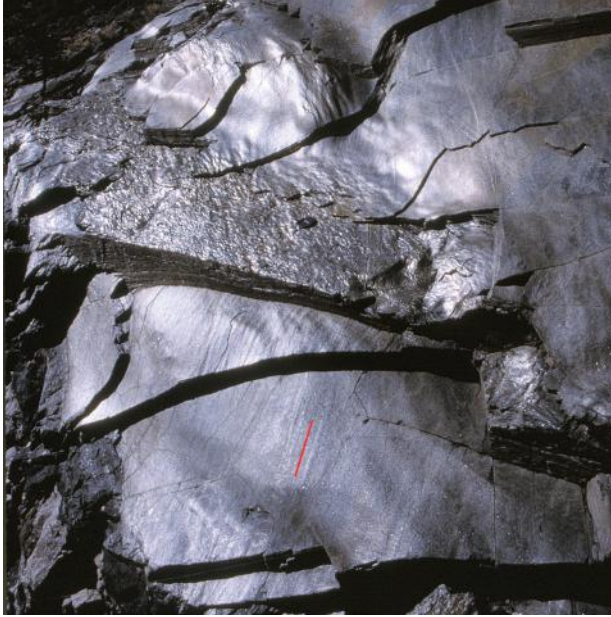
Figure 15.7 Foliation and cleavage surface in muscovite – biotite schist, reflecting the sunlight. The foliation is the result of parallel alignment of biotite and muscovite crystals. The alignment and excellent mineral cleavages of muscovite and biotite allows the rock to break along the foliation, so the rock cleavage is parallel to the foliation. Some of the irregularities in the foliation are caused by local deformation around quartz vein boudins. Small folds on the shiny cleavage surface, surrounding and parallel to the red line, are a weak cleavage-cleavage intersection lineation. Big Thompson Canyon, Colorado, USA.
