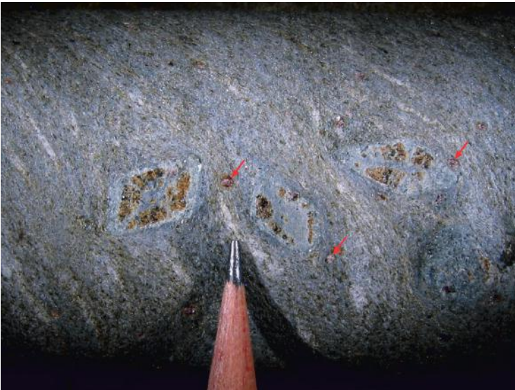
Figure 22.5 Drill core of pelitic schist with orange-brown staurolite porphyroblasts. The porphyroblasts have been partially replaced by a gray mixture of chlorite and muscovite. The replacement is irregular, affecting both the staurolite rims and cores, but leaving the intermediate parts. Based on examination of intact prograde staurolite in nearby rocks, it turns out that staurolite cores were rich in quartz inclusions. Not only did the inclusions increase the grain boundary surface area along which fluid could migrate, but the extra quartz allowed faster progress of the quartz-consuming retrograde reaction (approximately staurolite + biotite + quartz +
