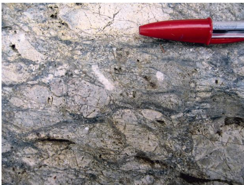
Figure 25.9 Rhyolitic pyroclastic rock, with light-colored clasts and darker, fine-grained material in between, metamorphosed to greenschist facies. The pen is oriented parallel to a spaced foliation and cleavage that wraps around the larger fragments. The fragments have resisted deformation and still have igneous textures, including recognizable, though sparse, phenocrysts. The dark matrix is made up mostly of a fine-grained, foliated mixture of white micas and quartz. Littleton, New Hampshire, USA.
