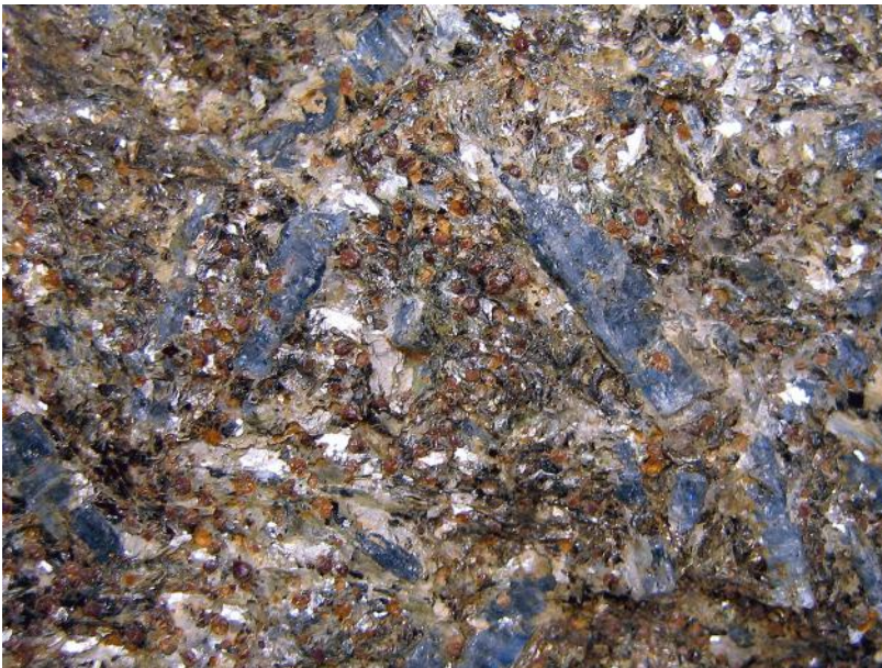
Figure 2.8 Close up of kyanite – garnet – muscovite – biotite schist. In schists, mineral grains are typically large enough to see and identify by eye or with a hand lens, in contrast to slate and phyllite where the grains are too small, except for porphyroblasts. The pervasive brownish-orange color is limonite staining from weathered sulfides, which easily penetrates the muscovite cleavage and fractures around garnets. The image field width is about 8 cm. Quabbin Reservoir, Massachusetts, USA.
