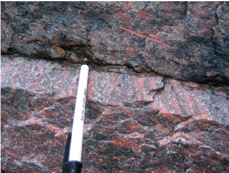
Figure 15.12 Lineated and foliated granitic augen gneiss. A strong lineation, parallel to the pen, is exposed on a joint surface that is close in orientation to the foliation (red line). The lineation and foliation are defined by extended and largely recrystallized pink and light-gray feldspar augen and the thoroughly recrystallized gray quartz – biotite matrix. The rock has almost no cleavage. Comstock, eastern Adirondacks, New York, USA.
