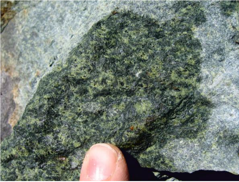
Figure 9.7 Gabbro, metamorphosed at epidote amphibolite facies, that is almost undeformed, shown wet and dry on a freshly broken surface. It contains the mineral assemblage chlorite – hornblende – epidote – calcite – albite – quartz, and is much coarser than nearby metamorphosed basalts. In thin section, relict augite can be found in the cores of some hornblende pseudomorphs after augite. Størås, Sør Trøndelag, Norway.
