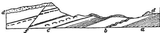
a, b, c. Stratified rocks inclined to the horizon. d. Superficial detritus. f. Fault interrupting and displacing the strata.
