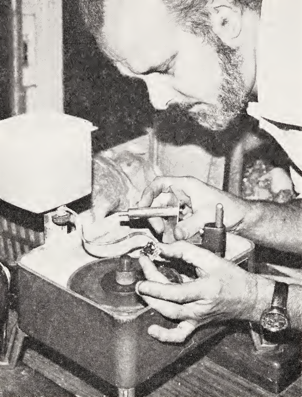
Page 114 (above) 'Gem Master' machine (see p 140) by M. L. Beach, of Twickenham, England, makes use of O'Brien templates; (right) Geogem (British) facetting appliance, comprising a sophisticated head on a mast, swivellable upon a stand. Transfer jig and a set of dopsticks in foreground
