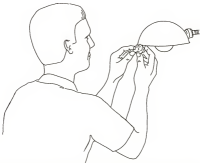
FIG. 12. Using a desk lamp to check for flaws in a transparent gemstone.
