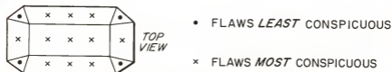
FIG. 4. Placement of small flaws in round brilliant and step-cut gems to disguise their presence.
