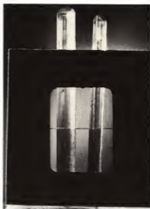
FIG. 8. Split-polaroid dichroscope placed before a pink tourmaline to show the two dichroic colors of rich pink and pale pink.
