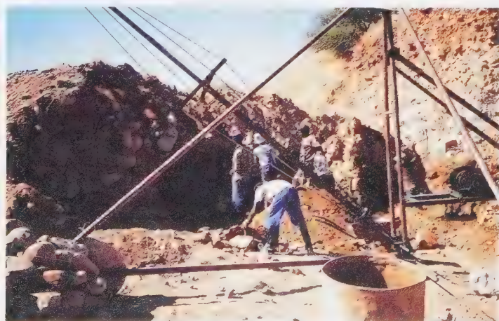
Figure 14. Basic alluvial operations along the Vaal River near Gong Gong in South Africa. At left, a team operation moves red gravel close to a lifting arm, and, on the right, are their basic trommel and washing pan. (George E. Harlow.)
