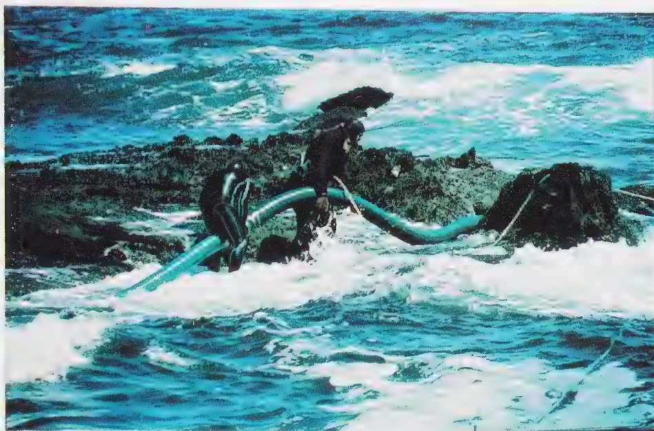
Figure 18. Suction pipes used to pump diamond bearing gravel are being moved into the surf by divers at DePunt, South Africa. (John J. Gurney.)
