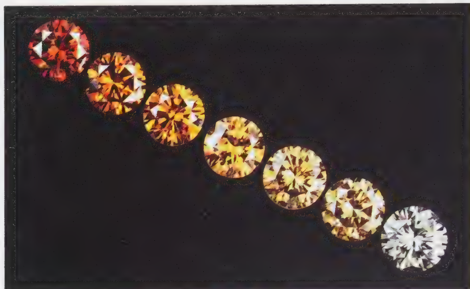
Figure 7. To give them a range of colors, diamonds can be treated by exposure to a source of radiation and then possibly by heating in an inert atmosphere. (Tino Hammid/courtesy of Gemological Institute of America.)
