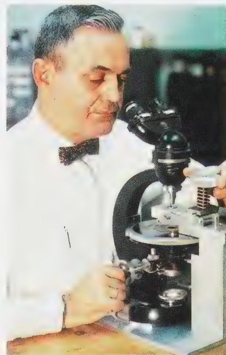
Figure 12. Diagram of lever-arm diamond anvil cell (adapted from Caveney, 1979) and Alvin Van Valkenburg in 1963 using such a device to study materials at high pressure including what he called "gincicles" (bottom) alcohol crystals formed when liquid alcohol is raised to high pressure in the diamond anvil cell. (Courtesy of Geophysical Laboratory, Carnegie Institution of Washington.)
