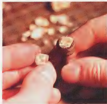
Figure 23. A diamond being notched (top) and cleaved (middle), with the two halves after cleaving. (Courtesy of De Beers.)
