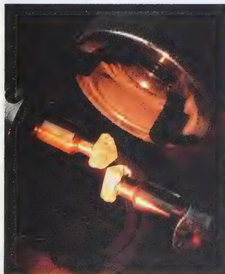
Figure 25. The bruting of two diamonds captured in stroboscopic light, which permits more rapid and accurate shaping. (Courtesy of De Beers.)
