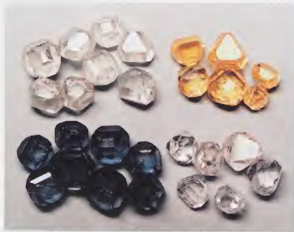
Figure 5. De Beers diamonds grown by the temperature-gradient method. The yellow diamonds were grown from a cobalt solvent with a small concentration of titanium to act as a nitrogen getter. The residual nitrogen concentration was about 20 ppm. The nearly colorless and blue stones were grown from an iron solvent, with aluminum added as a nitrogen getter; for the blue crystals a small quantity of boron was added to the growth capsule. The weights of the diamonds range from 1 to 3 carats, and they were grown for experimental purposes. (Courtesy of De Beers.)
