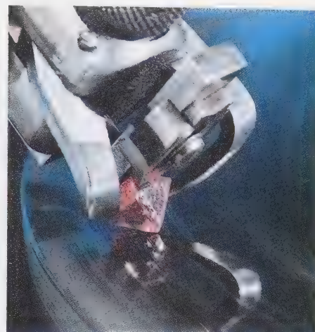
Figure 26. A diamond held in a mechanical dop and being polished on a diamond lap. (Courtesy of Argyle Diamonds.)
