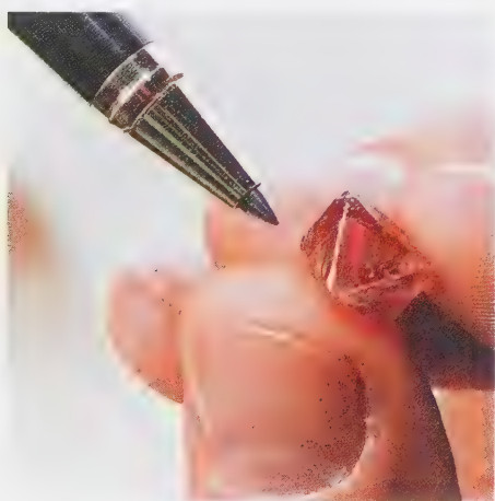
Figure 22. A diamond being marked for cutting with an ink pen. (Courtesy of Argyle Diamonds.)
