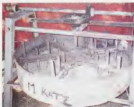
Figure 10. A 4-foot rotary washing pan. The gears drive the star-shaped support for vanes that push gravel along the base of the pan. When the pan is filled with "puddle" and gravel, heavy minerals, including diamonds, move to outer wall while waste washes out the center hole. (George E. Harlow.)
