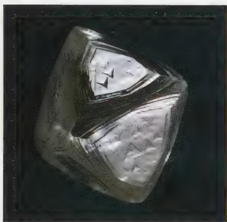
Figure 3. The octahedral diamond crystal shown (above) is approximately 8 mm wide, and the “ball and stick” model (below) of the diamond structure shows the atoms 1 cm apart and the bond arrangement that produces octahedral cleavage in diamond. If the model were expanded to show all the atoms in the real crystal, it would stretch for 519 km (325 miles), roughly the distance from New York City to Niagara Falls, N.Y., as shown on the map (right).
