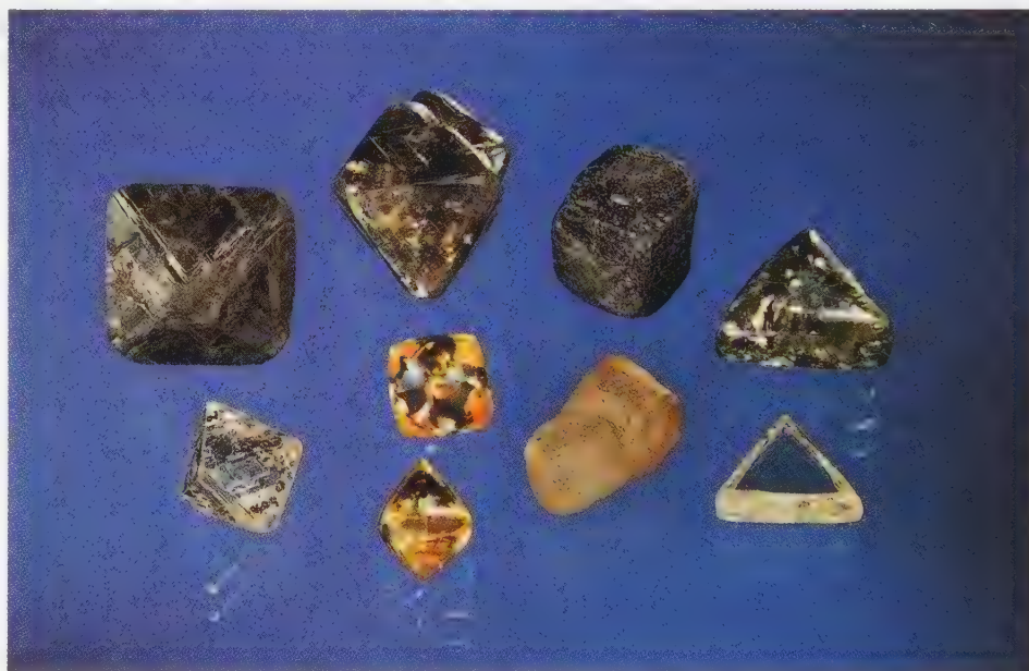
Figure 5. The photograph shows octahedron (left), etched octahedron (center), cube (top middle right), intergrown dodecahedron (bottom middle right), etched macle (upper right), and flat macle (lower right). The idealized drawings below show some of these basic habits of diamond: from left to right they are an octahedron, a cube, a cubo-octahedron (combined) form, a macle twin, and a dodecahedron. (Harold and Erica Van Pelt/courtesy of American Museum of Natural History.)
