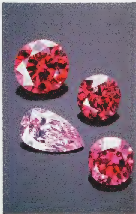
Figure 15. Red and purple are among the rarest hues in diamonds, and pink is certainly one of the more attractive colors. Each of these colors is due in total or in part to a color center resulting from deformation. However, the atomic details of the center, and whether or not it incorporates an impurity, remain mysteries. These stones range between 0.50 and 0.95 carats. (Tino Hammid/courtesy of Gemological Institute of America.)
