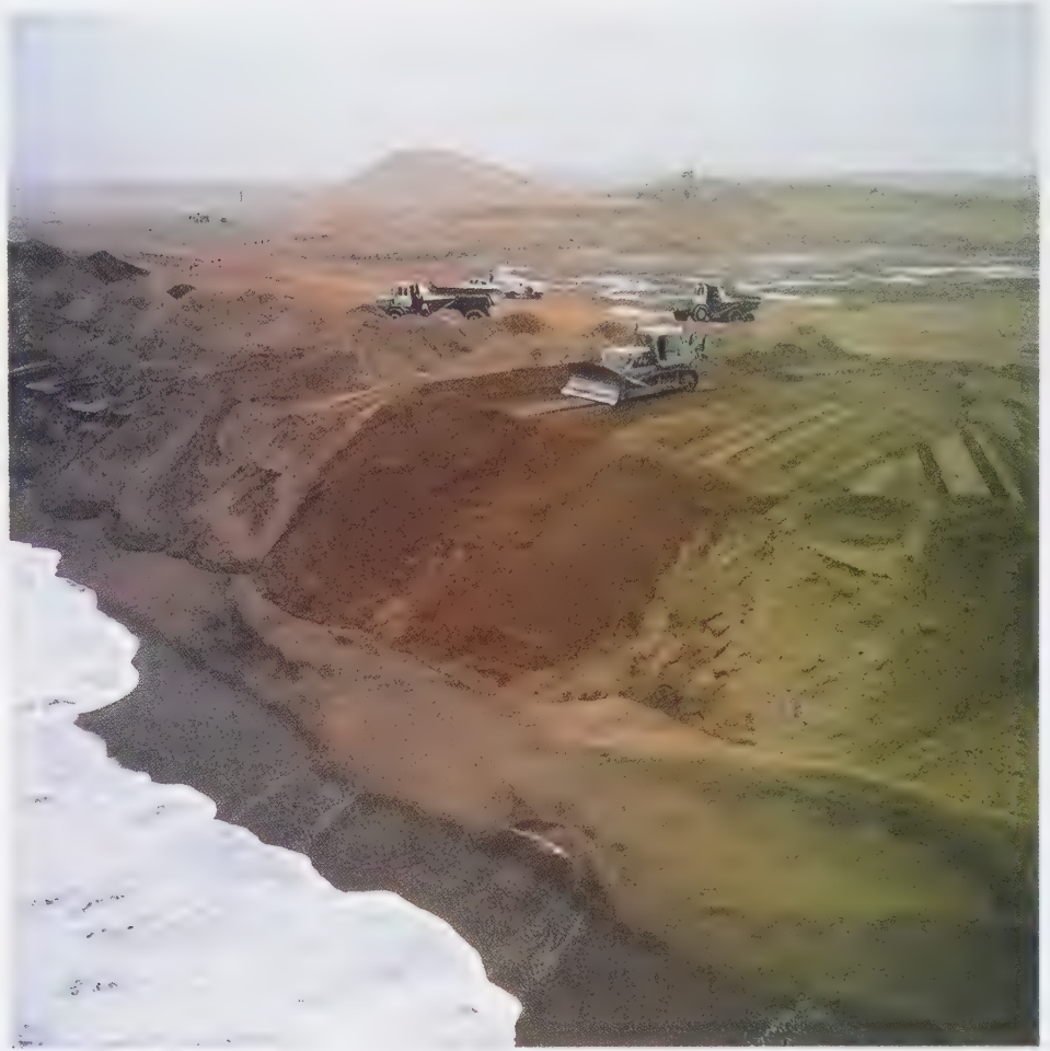
Figure 22. Massive sand walls hold back the sea during the mining of diamond-bearing terraces in the foreshore to depths of 20 m (66 feet) below mean sea level. Consolidated Diamond Mines (now Namdeb) has used this engineering technique successfully in Namibia. (Courtesy of De Beers.)
