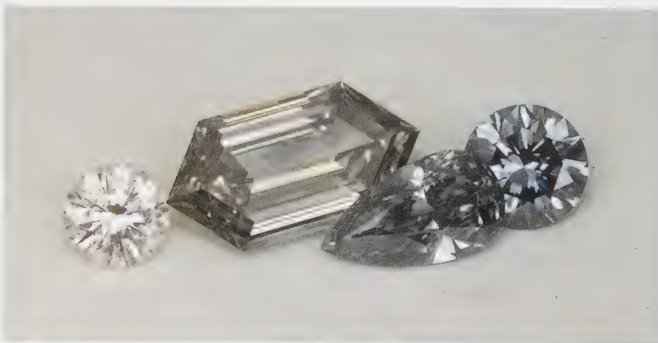
Figure 23. Hydrogen is believed to be the cause of color in these gray and grayish violet and blue diamonds. The colorless (E-color) reference stone on the left weighs 0.35 carats. (Stephen Hofer.)
