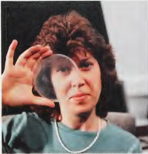
Figure 9. A wafer of CVD diamond (Diafilm) grown by De Beers, illustrating its exceptional transparency. The wafer is 105 mm in diameter and 630 \mu\text{m} thick (about 4 by 0.025 inches). (Courtesy of De Beers.)
