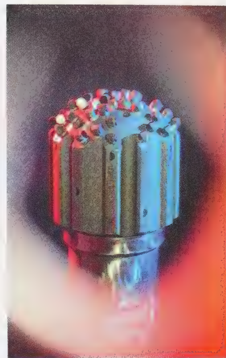
Figure 30. A drill bit armed with polycrystalline diamond (PCD) teeth used in petroleum exploration. The long life of the diamond edges reduces the frequency of removing the entire drill assembly (perhaps several thousand meters) and, thereby, reduces the cost. (Courtesy of GE Superabrasives.)
