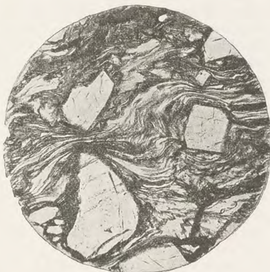
Fig. 211. Flow structure shown in a thin section of lava. Magnification 45.
