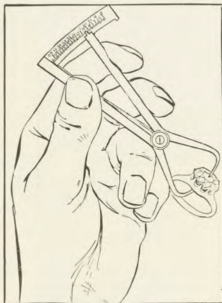
"THE MOE" DIAMOND GAUGE AND CALCULATOR.
