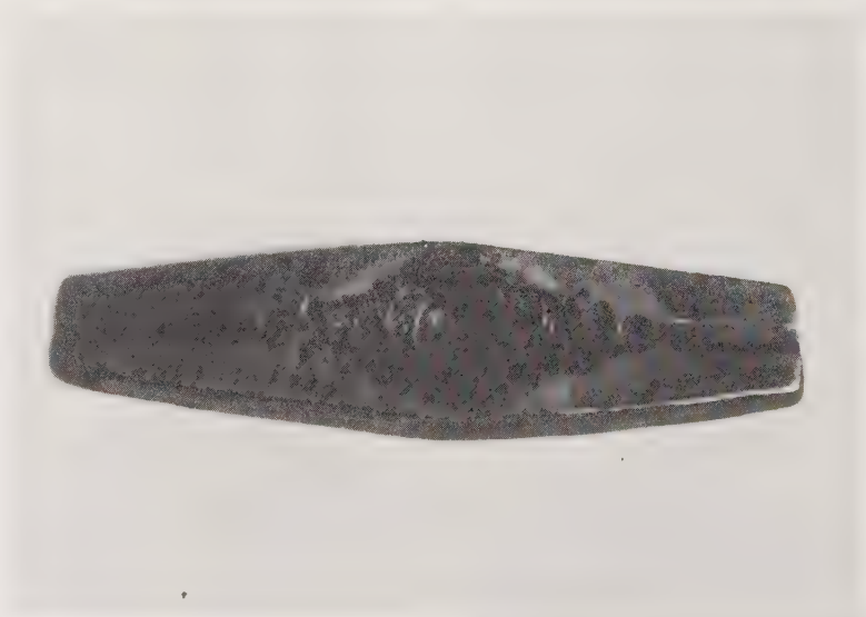
Fig. 6 Die stamped sheet using layers of paper to forge the sheet into the die under the blows from a hammer
