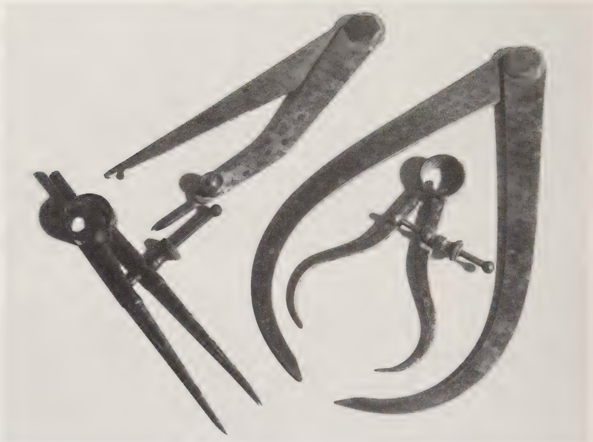
Fig. 29 Dividers and callipers for marking out and comparing
