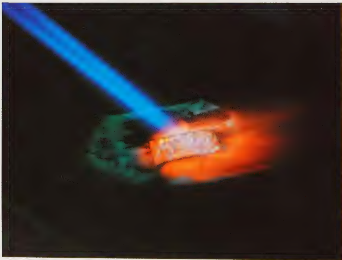
Fusing silver sheet and pieces of silver under a hot gas flame
