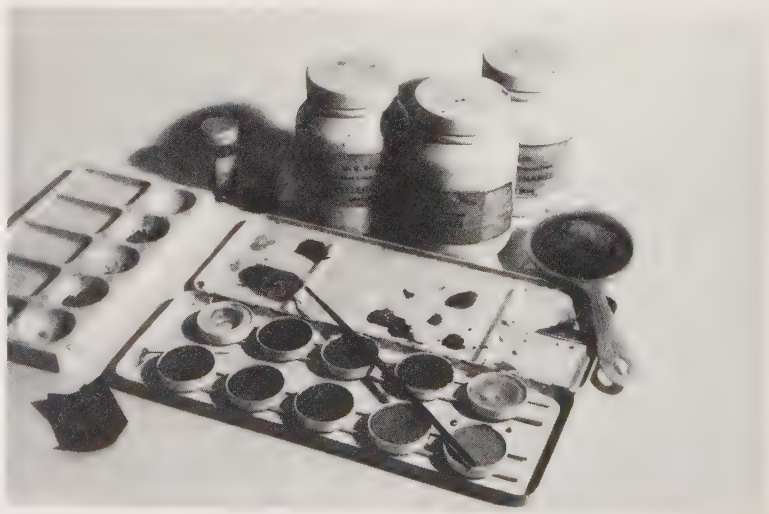
Fig. 12 Painting enamel and powdered enamel
