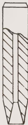
Diag. 215 Hollow sharp edge cutting punch with rod to assist in pushing out cut piece
