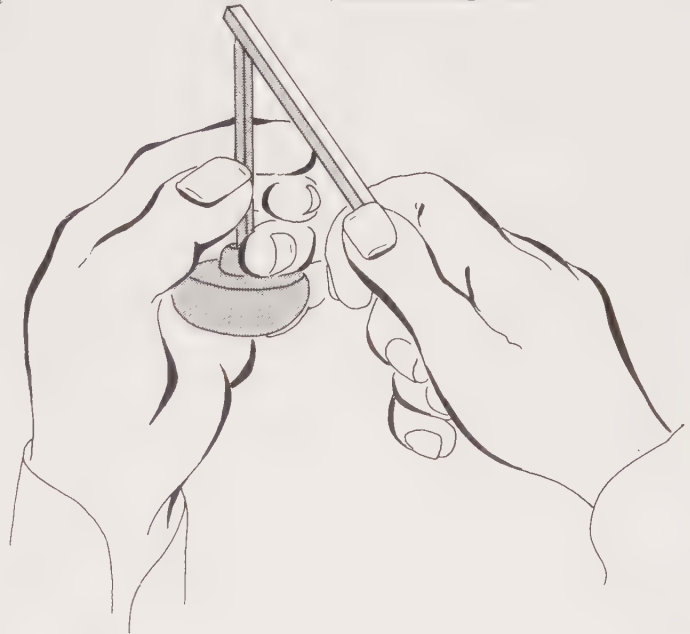
Diag. 5 Using an Arkansas stone to relieve the back of a graver
