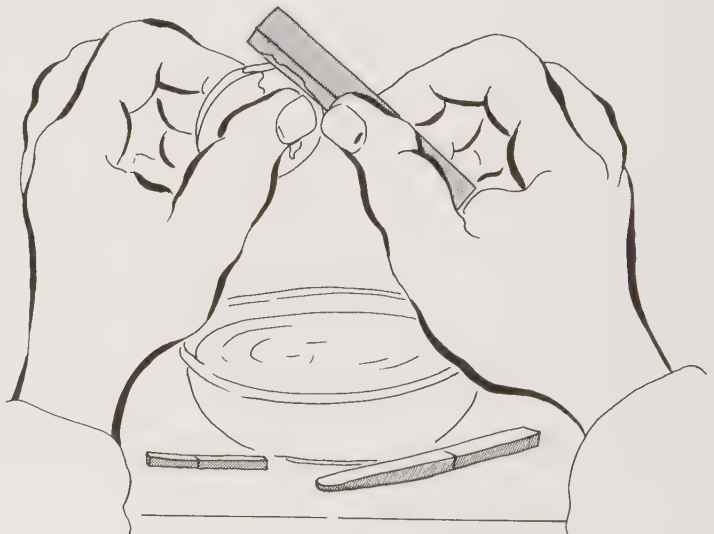
Diag. 136 Water of Ayr stone being used to smooth the edge of a piece
