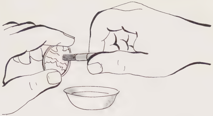
Diag. 110 Using a glass brush to clean a piece prior to enamelling
