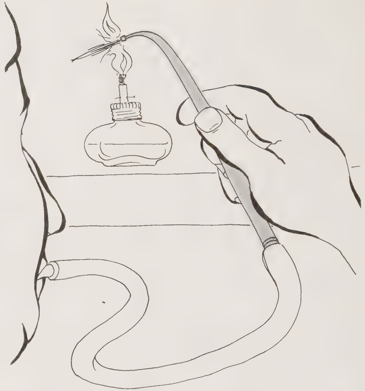
Diag. 40 Blow pipe in use with a spirit lamp
