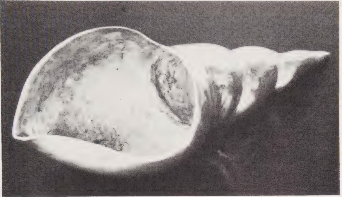
Fig. 17 Silver shell made by forming up a cone and hammering it up to shape over a mandrel
