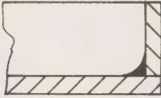
Diag. 129 Normal solder fillet
