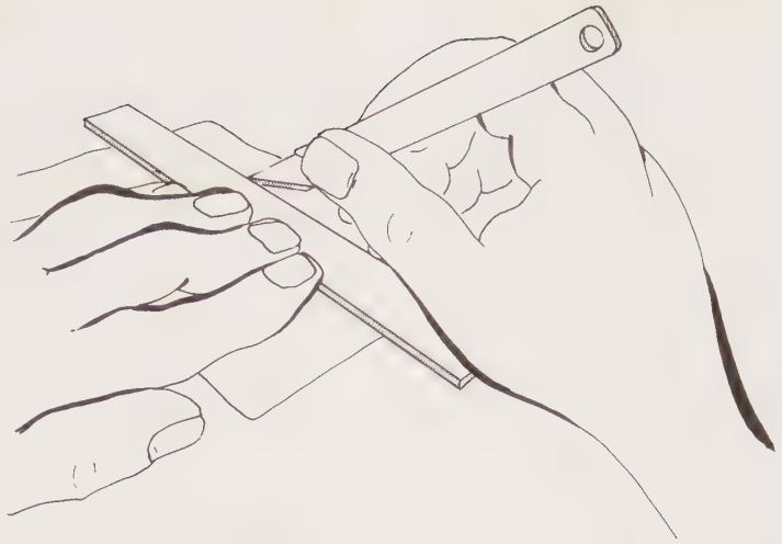
Diag. 72 Cutting a straight edge with a craft knife
