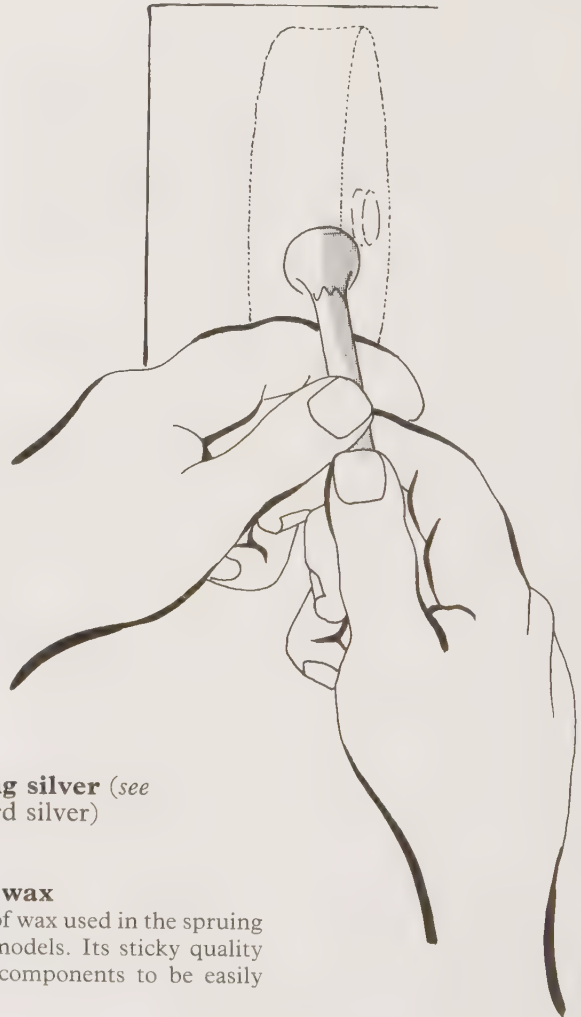
Diag. 259 Grinding a stone to shape
