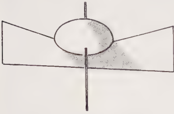
Diag. 109 Stainless steel support for counter enamelling
