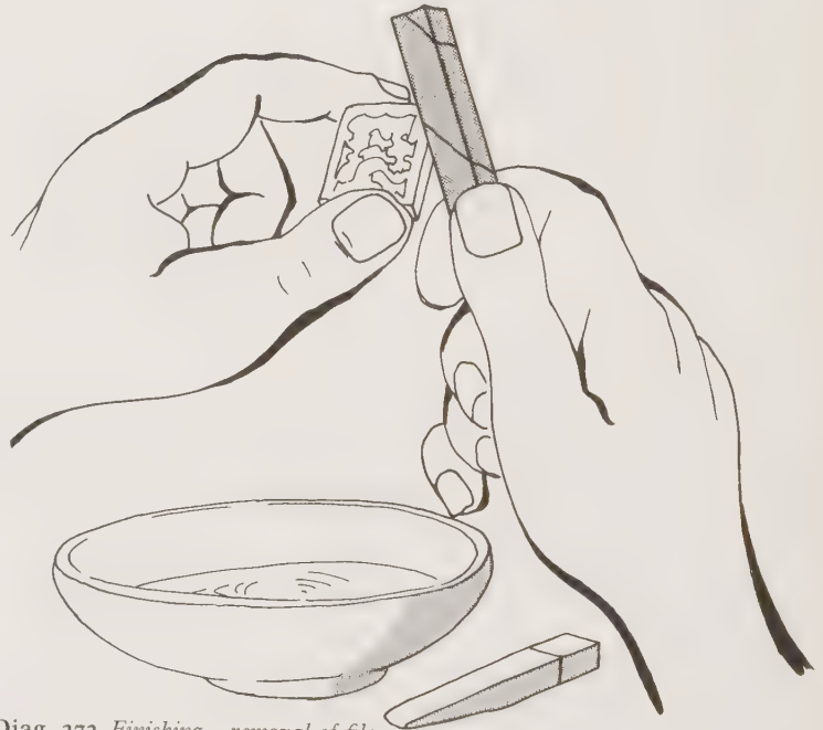
Diag. 272 Finishing – removal of file marks with water of Ayr stone
