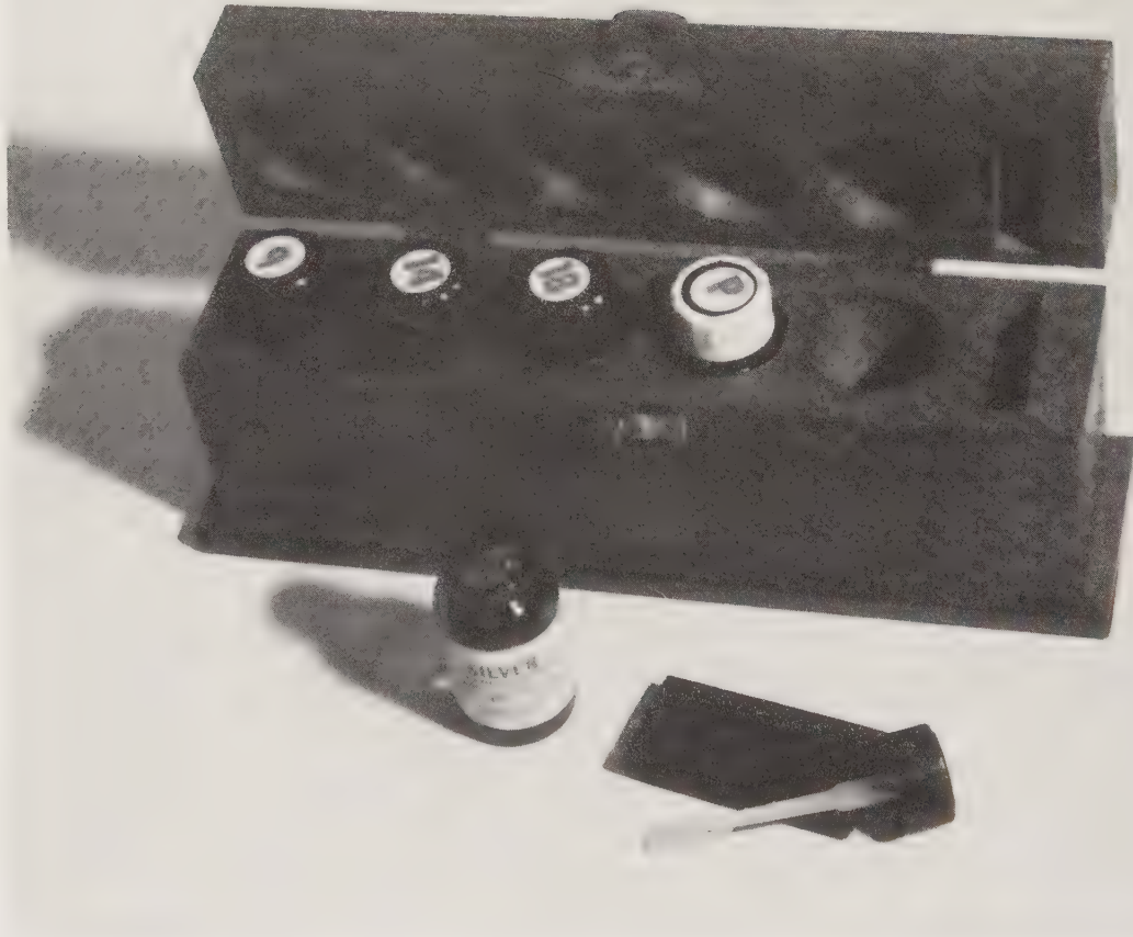
Fig. 2 Acid testing kit for precious metals
