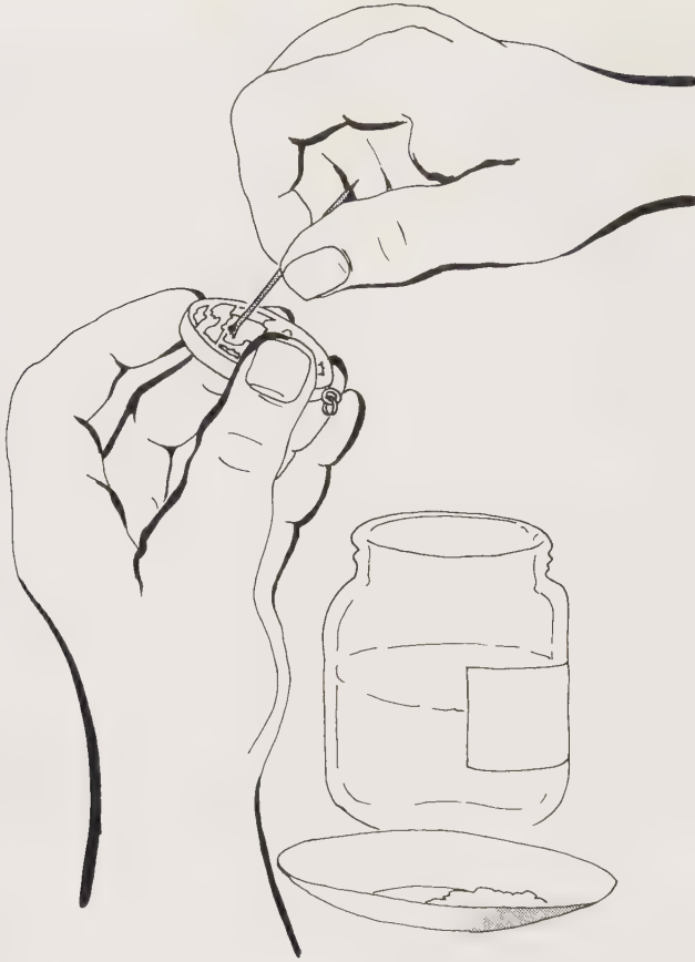
Diag. 106 Using emery powder
