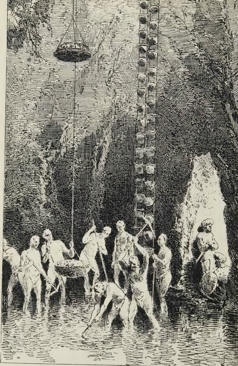
An ancient diamond mine at Panna, India. Buckets carry earth to surface; armed guards control shaft entrance at right.
