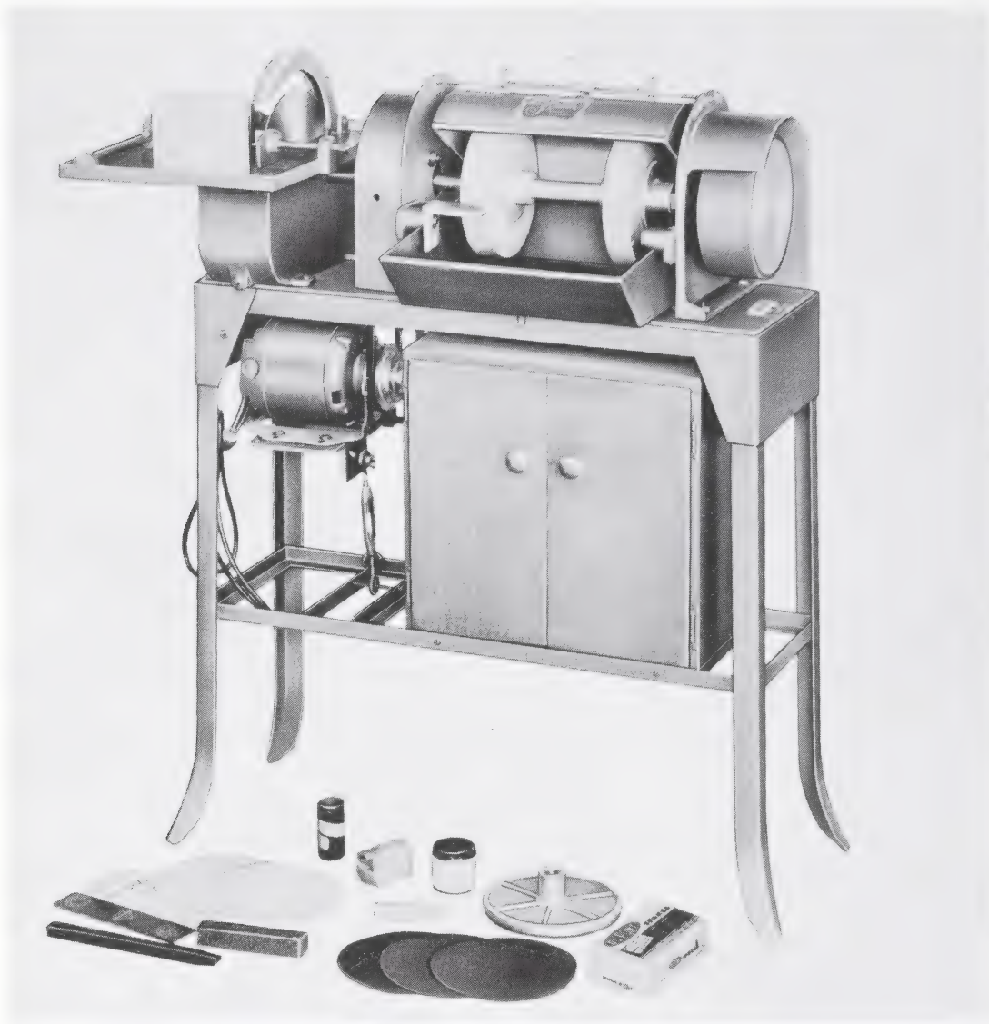
FIG. 122. Frantom De Luxe model lapidary outfit manufactured by Frantom Lapidary Equipment Company, Gardena, California. Priced at $238.00, complete with motor, saw and blade, grinding wheels, polishing disks and buffs, in addition to all accessories. (Photo by Folger, Los Angeles.)
