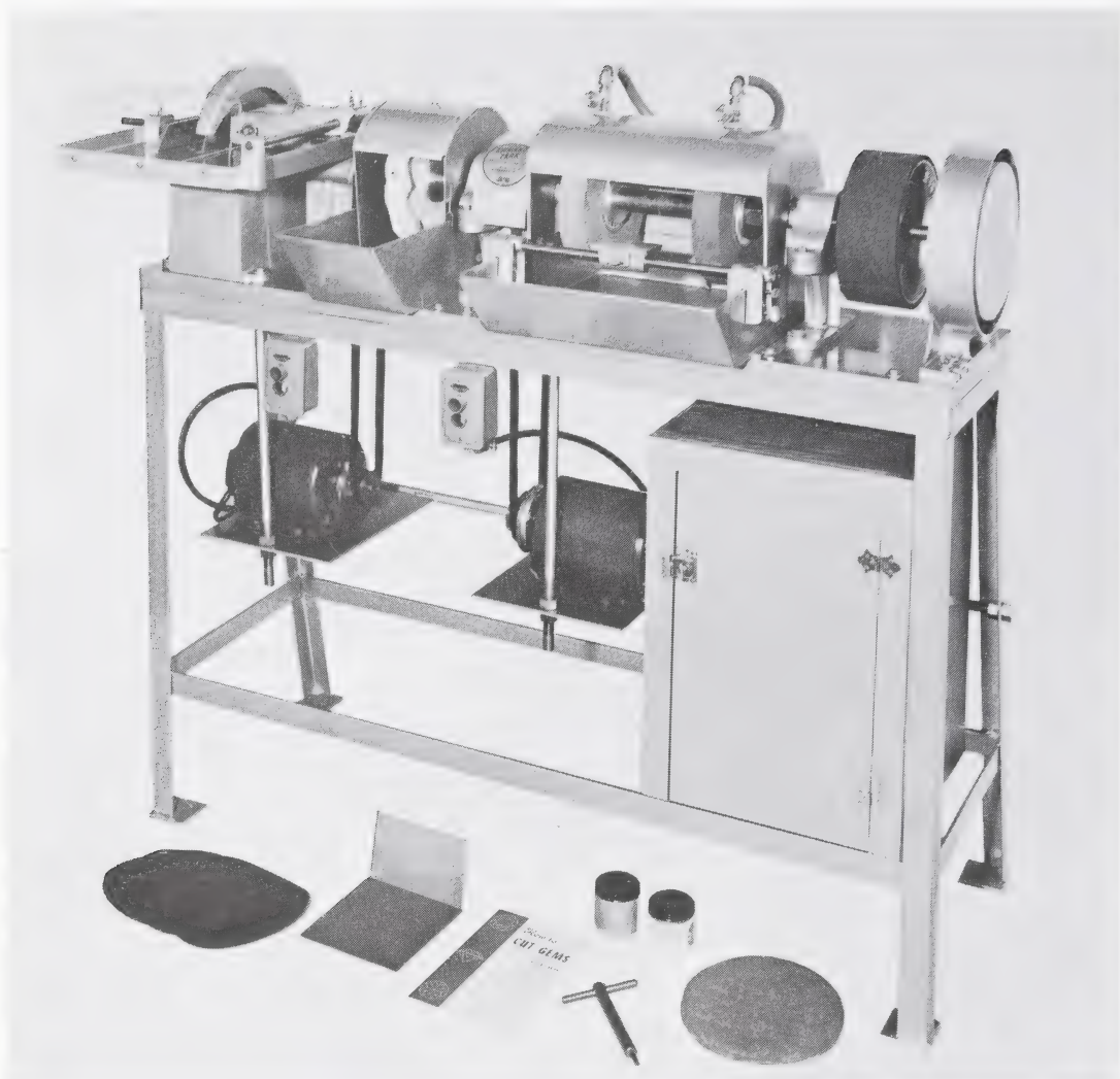
FIG. 127. Complete combination unit for lapidary work, manufactured by Highland Park Manufacturing Company, South Pasadena, California. This unit has everything including a saw with a separate motor, accessories and a storage space for unused polishing felts, etc. It retails complete with motors for approximately $320.00. ( Photo by Allen Hawkins, Pasadena. )
