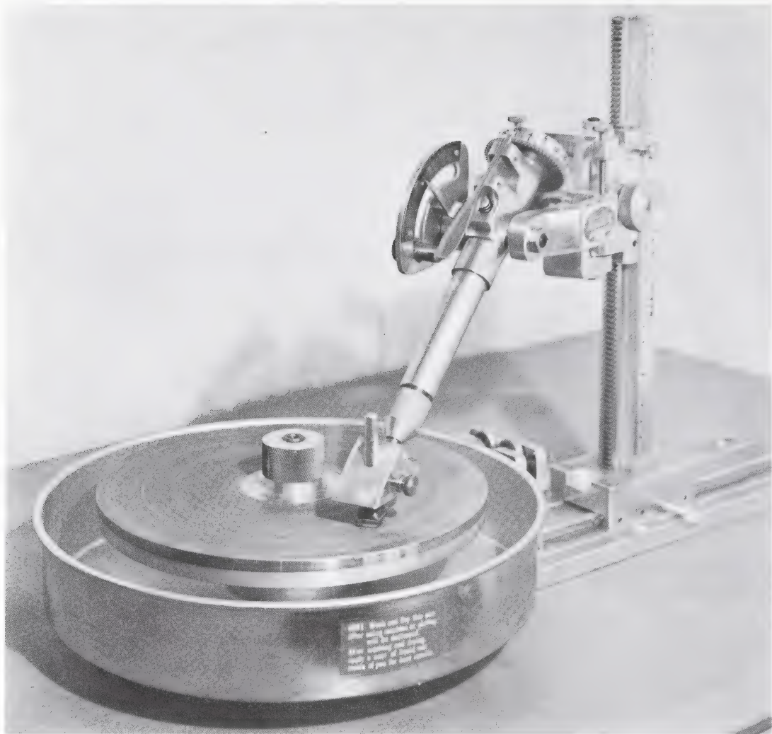
FIG. 118. Master facet unit with a 45^{\circ} angle dop for faceting the table on a cut crystal gemstone. Manufactured by M. D. R. Mfg. Co., Los Angeles.
