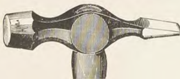
Fig. 26.—Steel-head Hammer with Flat Face and Pointed Pane.
