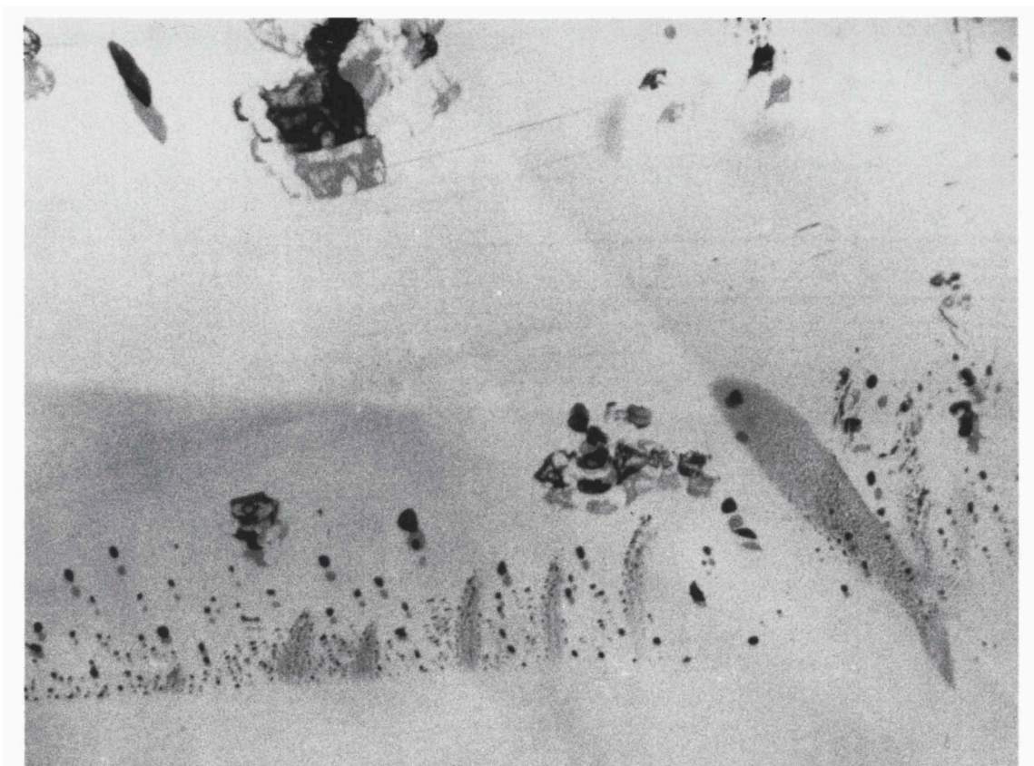
Fig. 4. Liquid inclusions in sphene RGM 151 855 from Sri Lanka, \times 25 . Note the strong doubling of the inclusions.
